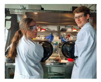
Postdoc Dr. Valerie Siller and PhD student Samuel Gatti assemble air-sensitive Li-ion and Na-ion test cells with solid and liquid electrolytes.
