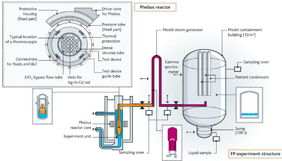
*Schematic diagram of the PHEBUS FP test setup and the test fuel bundle [8]*
