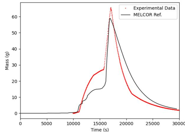
*Aerosol suspended mass in the containment atmosphere [12]*
