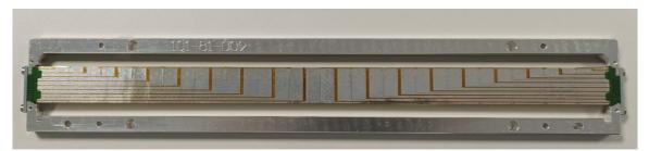
1) The HDI flex is installed on a ring frame and glue is applied at its back so that chips can be glued on it.
