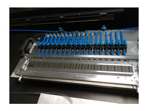
A series of 18 silicon chips aligned on the chuck. Alignment precision  $^{\sim}6 \ \mu m$ .
