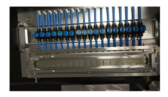
**3)** The ring frame is slotted in over the chips on the chip chuck.
