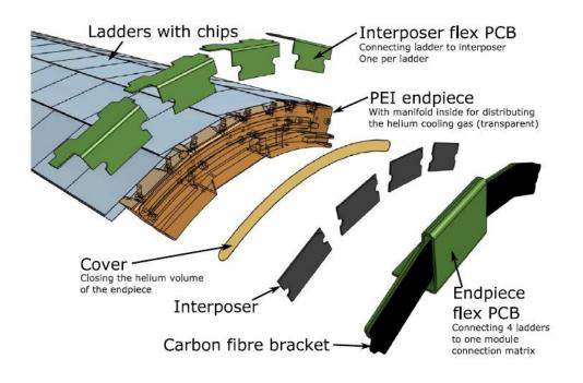
Exploded view of the outer layer module assembly.
