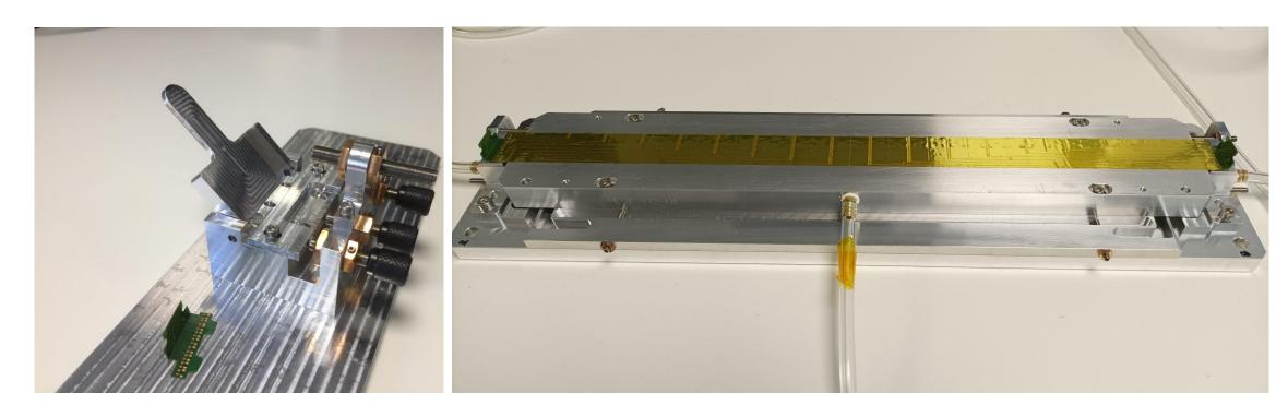
Left: flex interposer bending tooling. Right: the HDI flex is placed on a vacuum chuck and aligned against the flex interposers mounted at the ends.
