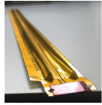
Flex tape mock-up with V-fold (right).
