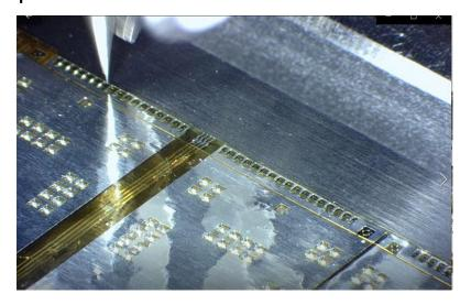
7) V-folds glue deposition on the glue robot.
