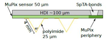
V-folds are made of  $25\mu m$  thick polyamide layer with a V-shaped cross section. They run along the ladder longitudinal side, from end to end.
