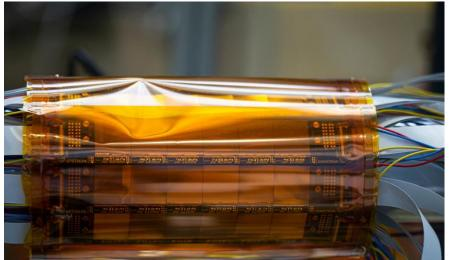
This is the inner module of the tracker detector in Mu3e. There are two layers made of 18 (8+10) ladders containing 6 chips each.
