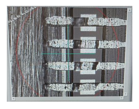
**4)** Fine alignment of Al traces on the HDI flex against the chip pads underneath.
