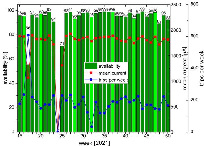
**Figure 1:** Weekly availability of the High Intensity Proton Accelerator facility in 2021. Already in the first 2 weeks of operation an availability of 96% was achieved. The two major drops in availability were caused by the electrostatic injection channel (70h) and the difficulties in re-commissioning the Ring after the magnet AXA repair (6d).
