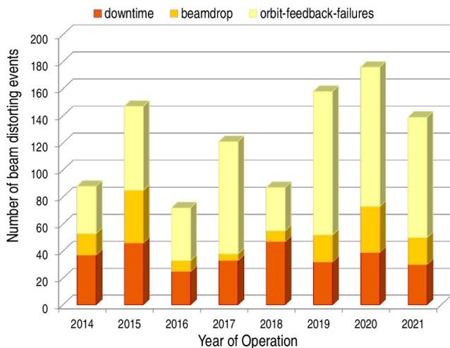
**Figure 6:** Number of beam distortions at the SLS
