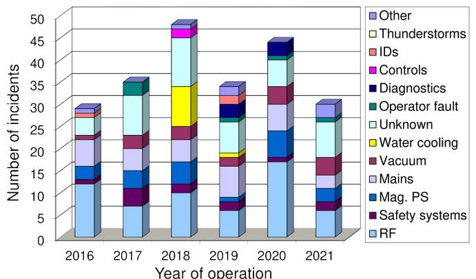
**Figure 5:** Beam outage count per system for the SLS
