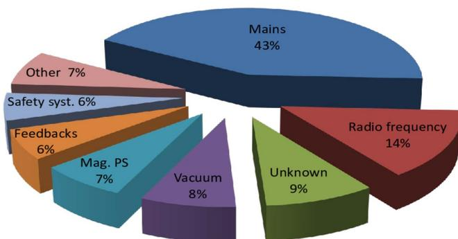
**Figure 7:** Beam outages per failure category at the SLS
