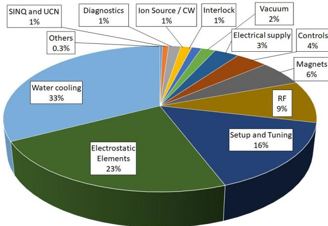
**Figure 4:** Beam outages per failure category at HIPA.
