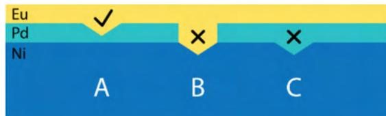
Figure 1: Refinement strategy of CR using a thin layer of Pd deposited onto of a suitable backing foil (e.g., Ni): electroplated element (e.g., Eu) is envisaged to form an intermetallic compound with the underlying Pd by CR (A), whereas a diffusion into the backing foil (B) has to be minimized; diffusion of Pd into the backing is likewise unfavorable (C).
