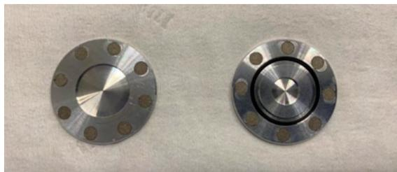
Figure 3: The coin target (24 mm diameter, 2 mm thick).
