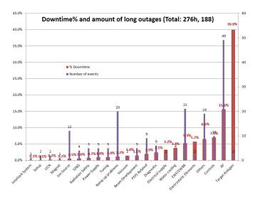
Figure 2: long outage (t>5m) characteristics of the High Intensity Proton Accelerator facility in 2020
