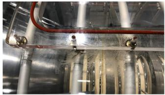
**Figure 1:** Acrylic glass tube surrounding the acceleration section of the Cockcroft-Walton. The visible brownish "bloom", formed a conductive layer of 100 M $\Omega$  instead of the required 50 G $\Omega$ .
