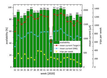
**Figure 1:** weekly availability of the High Intensity Proton Accelerator facility in 2020
