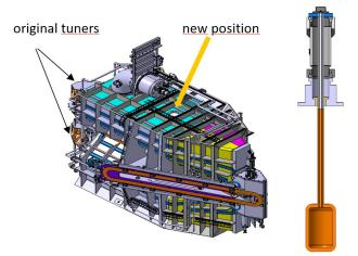
**Figure 3:** right, draft design of a new tuner without finger contacts. The movable displacer will extend 1 m into the resonator to tune the resonance frequency within a range of 200 kHz. It will be installed in a new position in addition to the original tuners.
