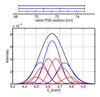
FIG. 7. Simulated elastic intensities from the 7th analyzer segment along one PSD tube plotted as a function of  $E_f$ . The peak energy for the different pixels (red) is slightly shifted due to the prismatic analyzer. By binning pixels (blue) the intensity can be increased while slightly worsening the energy resolution. The integrated intensity is shown by the black line. The pixel position along the PSD tube for the different binnings is sketched above.
