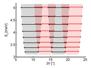
FIG. 4. Angular coverage of two neighboring analyzer segments for two sample scattering angles,  $2\theta$  (black) and  $2\theta + 3.75^{\circ}$  (red). For the first analyzer segment at  $E_f = 3.2$  meV there is almost no overlap between the two measurements while the overlap increases to 2/3 for the last analyzer segment at  $E_f = 5$  meV.
