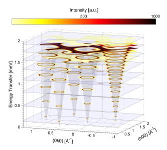
FIG. 10. Calculated intensity for a typical spin wave excitation covered by an 81 step scan (step size  $1^{\circ}$ ) with the same parameters as used in Fig. 9. Here, for visibility all 24 energies are only shown in the outermost cone. For the rest of the data only the maps from the central energy of each analyzer segment are shown.
