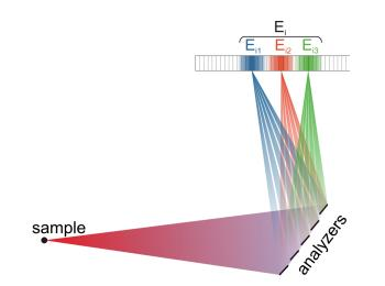
FIG. 6. Sketch of the prismatic analyzer concept. Five analyzer blades are oriented in a focusing Rowland geometry. Due to the relaxed mosaicity (60') and distance collimation, the slightly different reflected energies represented by the different coloring are clearly separated and detected in the pixels of the position sensitive detector.
