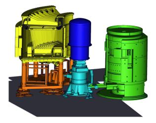
FIG. 12. Design drawing of the CAMEA spectrometer. The monochromator part (green) and sample table (light blue) are preserved while the secondary spectrometer (substructure (orange) and vacuum vessel (yellow)) are newly constructed. The vessel is thoroughly shielded against general background in the guide hall. The inner part of the vessel is shown in detail in Fig. 11.
