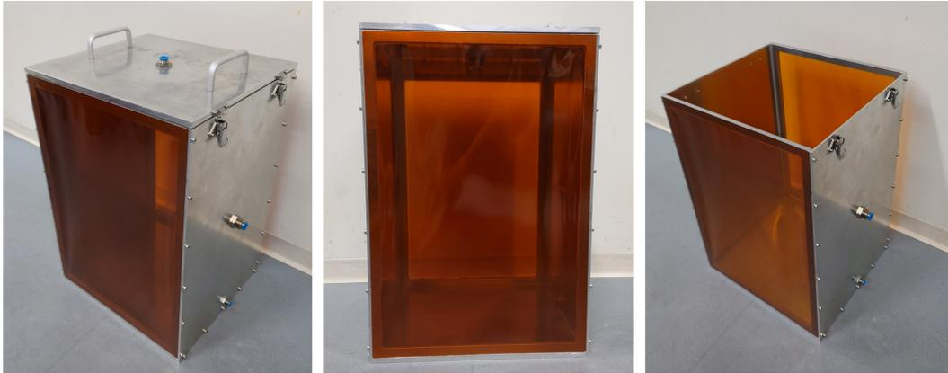
Fig. 8: The inflation chamber. The orange-brown Kapton foil is used to seal the chamber along the beam axis achieving minimal beam interaction.
