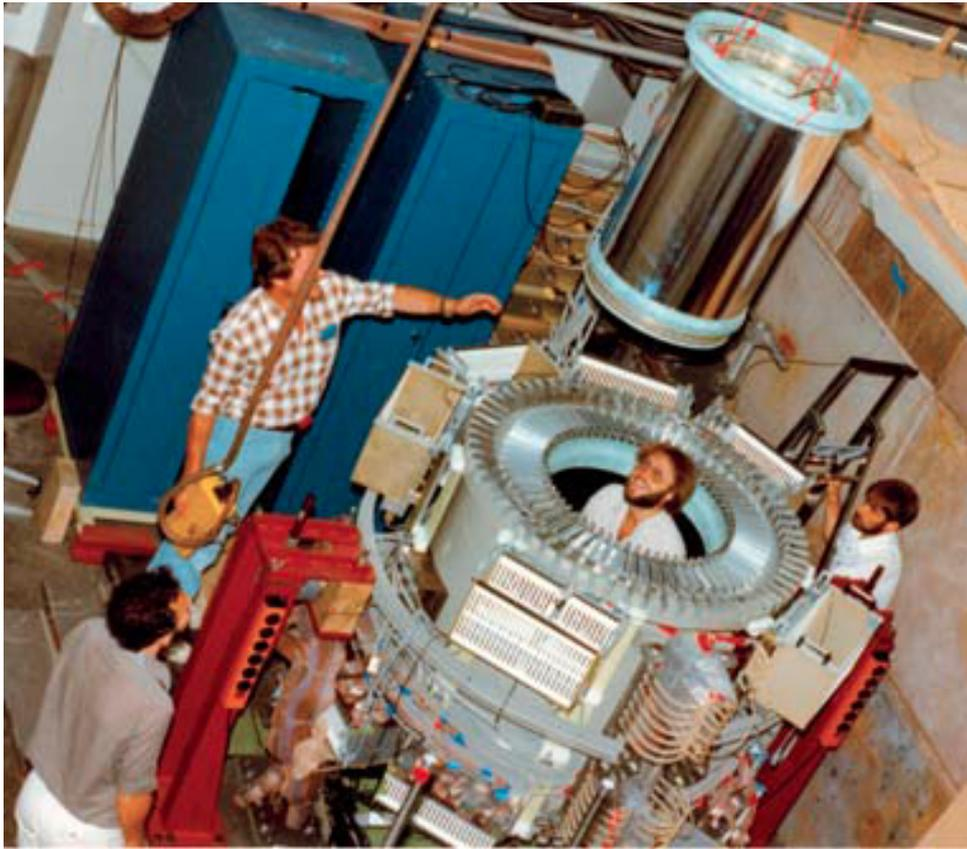
Figure 7.4: The assembly of the SINDRUM I detector in the vertical orientation. The MWPC are being lowered into the setup by (clockwise from top left) Erwin Hermes (technician UZH), Norbert Kraus (PhD student UZH), Nik Lordong (Technician PSI), and within the setup Michael Doser (Master student ETHZ).
