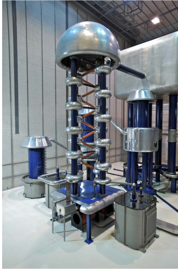
Figure 1.25.: PSI Cockcroft-Walton accelerator.
