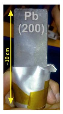
When the Pb crystal is aligned, you will acquire a series of either constant-q or constant-energy scans (or a combination) in order to map out the phonon-dispersion (hv as a function of q) along a selected high-symmetry direction (h 0 0). How to perform a scan will be shown to you by the local contact. However, just as an example, the two scans shown above in Fig. X are at the TASP instrument performed by running the following two text commands in the SIX-prompt:
