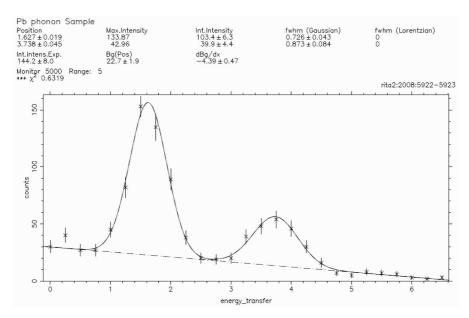
Figure 6: Screenshot from the FIT program showing how a constant-q scan is fitted by two Gaussian functions. The positions (energy transfer) showed in the top left corner together with the **q**-point at which the scan was performed will yield two unique (E,q) points of the phonon dispersion curves [see Fig. 7(a) below]. Remember to also record the error-bars of the position!
