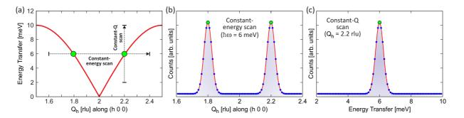
Figure 5: (a) Schematic view of how two points of the phonon dispersion curve can be measured using either (b) constant-energy scan or (c) constant-**Q** scan. By performing multiple scans it is possible to map out the complete dispersion (see below).
