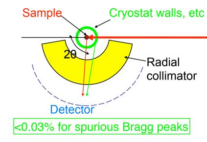
Radial collimator with the shielding.
