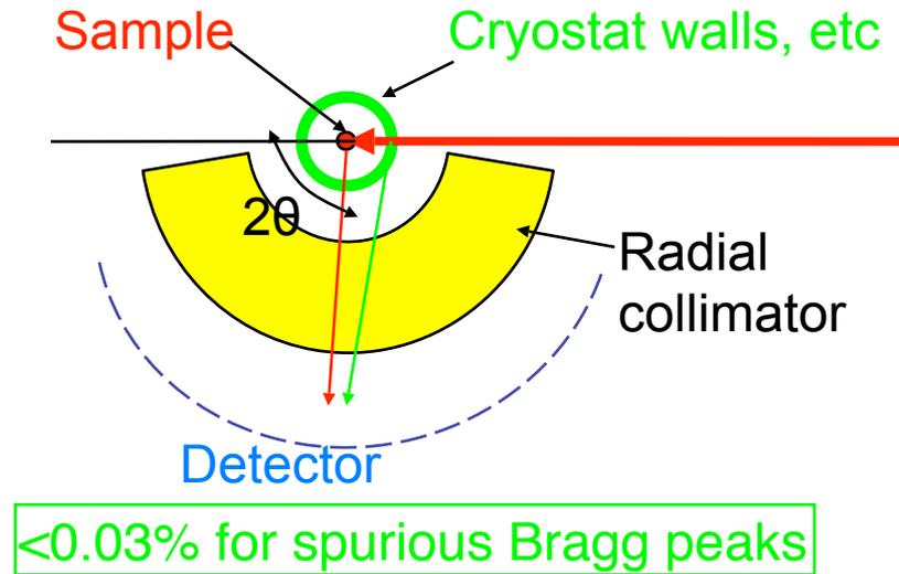
Radial collimator with the shielding.
