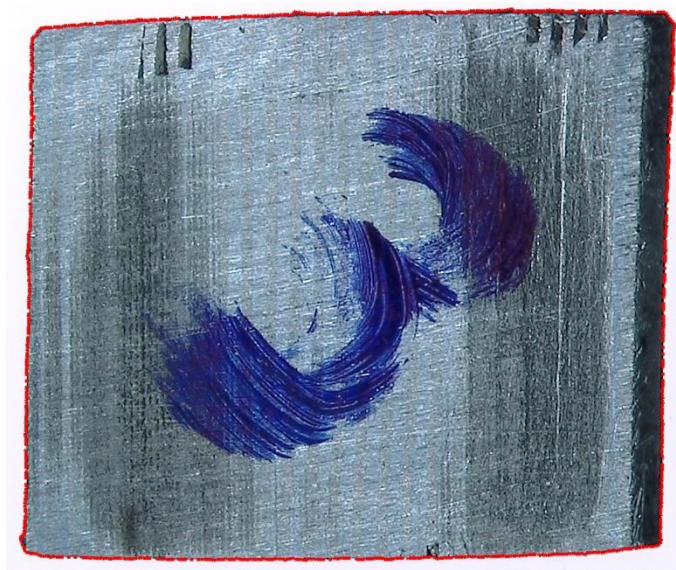
Figure 4-1 Example of GHFS optical area measurement and in-software sensor edge tracking
