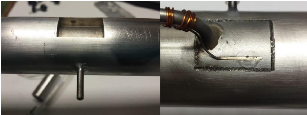
Figure 3-14 GHFS installation in the deep pocket
