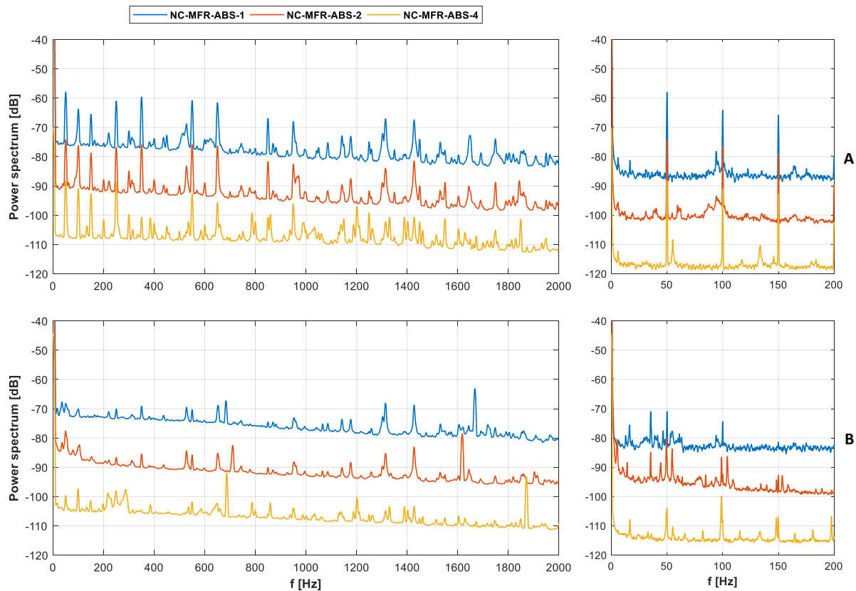
Figure 6-63 Power spectra comparison of the measured heat flux signal recorded with sensor 1 (A) and 2 (B), various experiments. For clarity of viewing, second and third spectrum offset by -15dB and -30dB. Experiments NC-MFR-ABS-1, NC-MFR-ABS-2, NC-MFR-ABS-4.
