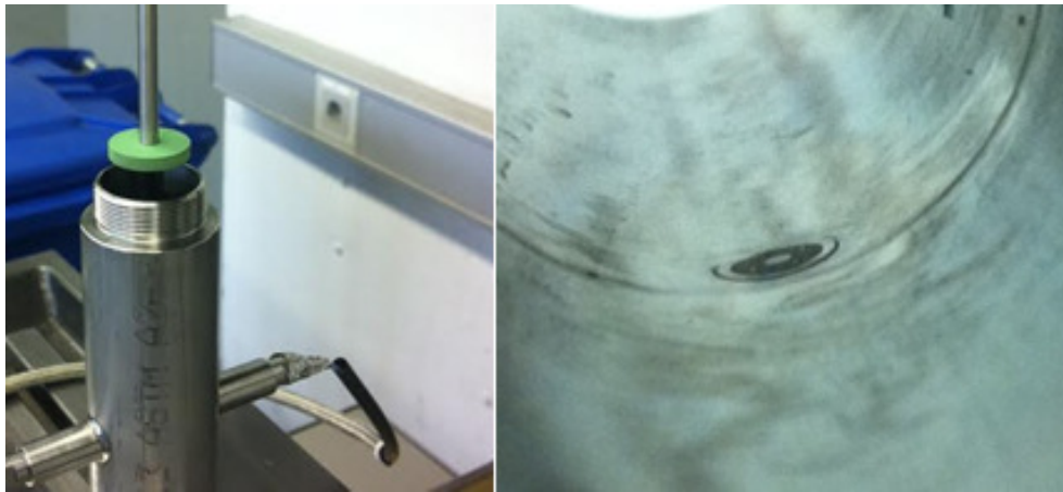
Figure 3-20 Polishing of an electrode array face, to match inner tube wall curvature
