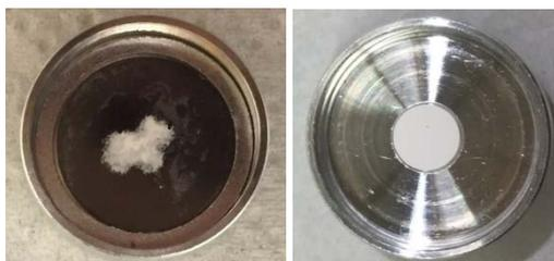
**Fig. 1:**  $^{44}\text{CaCO}_3$  pressed on to graphite (left). Enriched  $^{44}\text{CaO}$  pressed into a 6 mm pellet (right).
