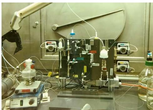
**Fig. 1:** The  $^{64}\text{Cu}$  chemical separation system.
