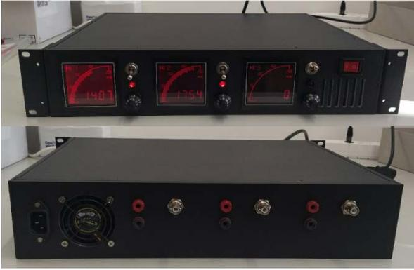
**Fig. 2:** Front panel (top) and rear panel (bottom) of the HVPS unit integrating 3 HV channels in 19" chassis.
