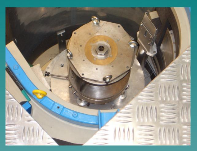
Photo of a high pressure setup using Paris-Edinburgh pressure cell at HRPT diffractometer. The sample volume is less than 100 mm<sup>3</sup>, approximately two orders of magnitude smaller than in a standard setup.
