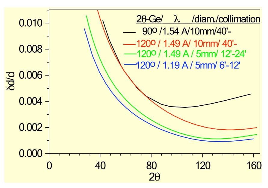
Comparison of resolution functions for different primary-secondary collimations. Typical modes are HI:40'-, MR:12'-24', HR:6'-12'. Counting rates are decreased by a factor of ~3 and ~(8-10) for MR and HR, respectively.
