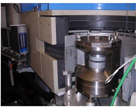
detector shielding + radial collimator + BN anvils + low noise ellectronics = excellent peak to background ratio
