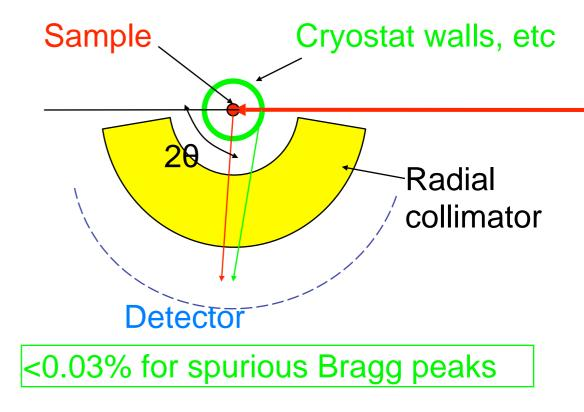
Radial collimator with the shielding.
