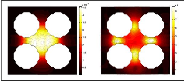
Figure 2: Sample results from a single-phase mixing test: time-averaged concentration distribution (left) and standard deviations of the concentration (right).
