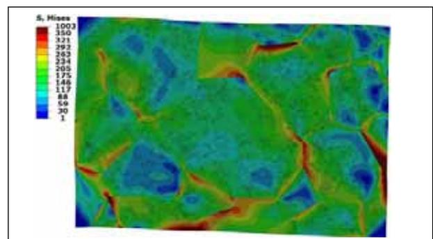
Figure 2: Von Mises stress distribution (in MPa) as a consequence of pure thermal loading.
