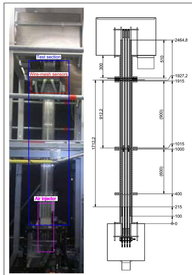
Figure 1: Overall view of the SUBFLOW test section.
