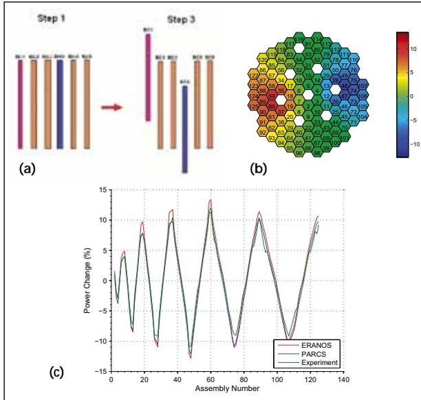
Figure 2: Results from the ‘blind’ CRS simulations: (a) change in the CR positions; (b) map of the resulting power deformation; and (c) assembly-wise comparison of the calculated and measured power changes.
