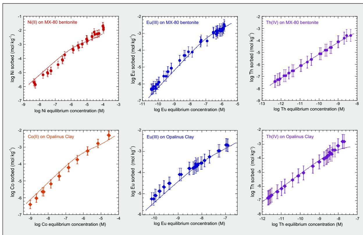
Figure 2: Sorption isotherms on MX-80 bentonite and Opalinus Clay: experimental results and modelling.
