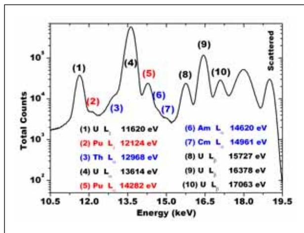
Figure 1: Fluorescence spectrum of the irradiated MOX sample. Positions (3), (6) and (7) are indicated for Th, Am and Cm, respectively, but with signals too low to be detected.
