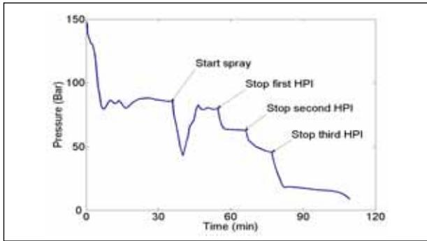
Figure 1: Pressure response during an SB-LOCA with operator actions.
