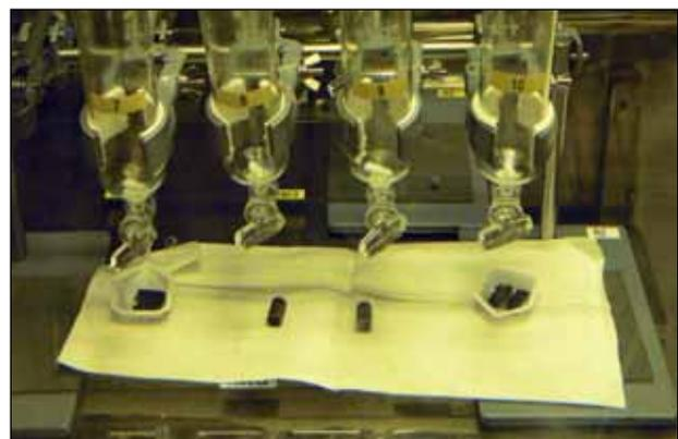
Figure 1: Experimental set-up for leach experiments (picture taken before the start of the experiments).
