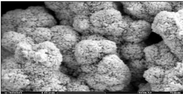
Figure 2: Conglomerations of small primary particles at 3000x magnification.
