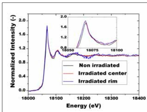
Figure 2: Plutonium L<sub>III</sub> XAFS spectra for the non-irradiated and irradiated MOX fuel in the centre and rim zones.
