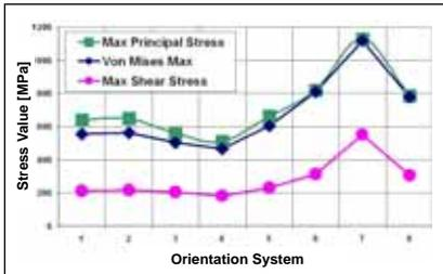
Figure 4: Maximum von Mises, principal and shear stresses for different orientations and grain sizes.
