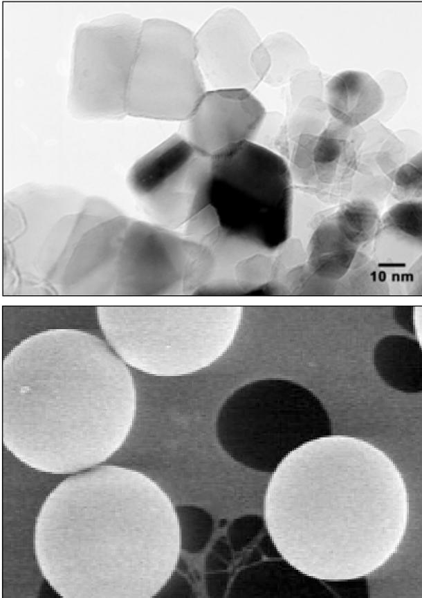
Figure 2: Electron micrographs of test aerosols: agglomerates (top) and spherical particles (bottom).
