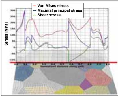
Figure 3: Von Mises, maximum principal and shear stress variations due to thermal loading along a horizontal line crossing several grain boundaries.
