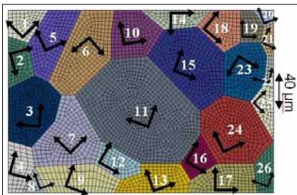
Figure 1: 2D polycrystal model: arrows indicate the orientations of the elastic properties of the grains.
