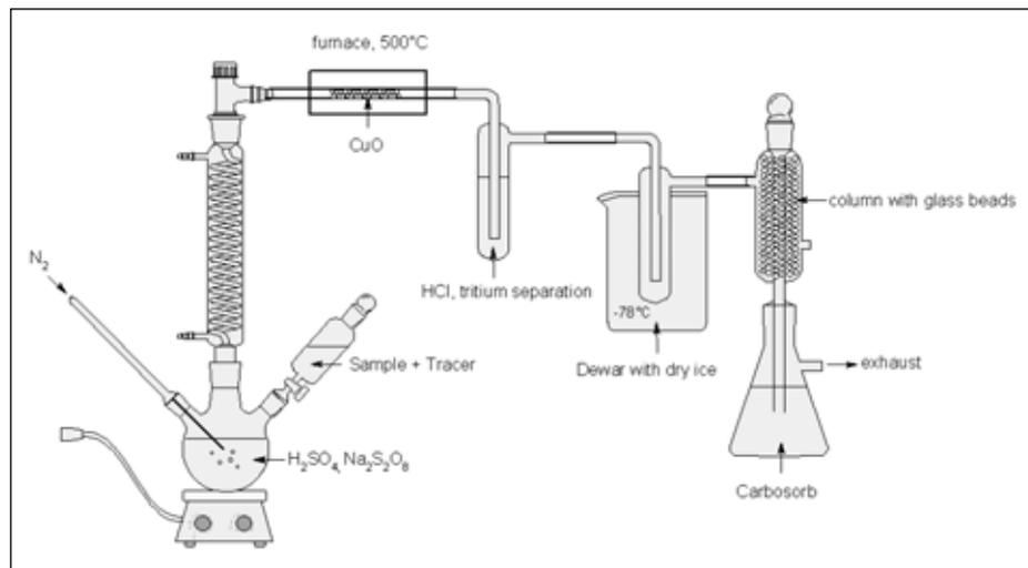
Figure 2: Experimental set-up for  $^{14}\text{C}$  extraction.
