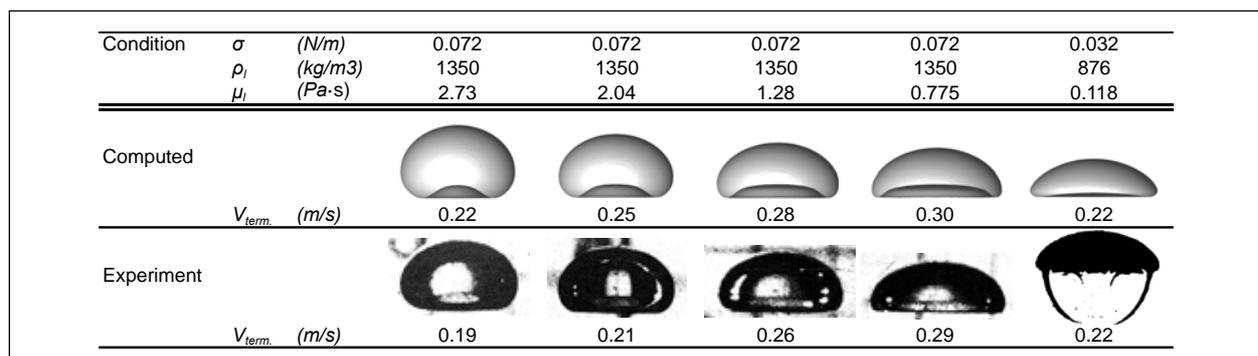
Figure 1: Shapes and terminal velocities of rising air bubbles in a liquid pool for different surface tensions ( $\sigma$ ), liquid densities ( $\rho_l$ ) and liquid viscosities ( $\mu_l$ ).
