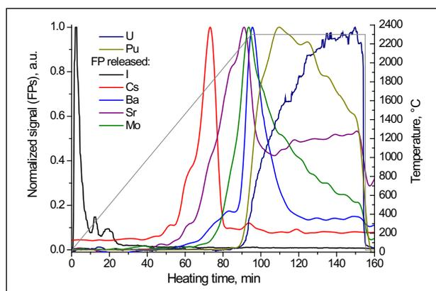
Figure 2: Release of FPs from irradiated uranium oxide fuel (burn-up 3.8%) measured using ICP-MS.
