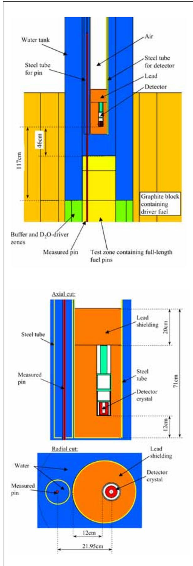
Figure 2: Axial (top) and radial (bottom) views of the MCNPX model of the planned measurement station in PROTEUS.
