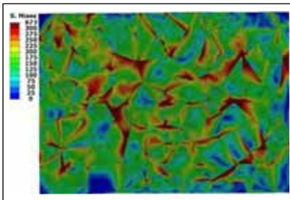
Figure 5: Von Mises stresses [MPa] for small grains.
