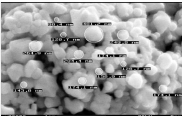
Figure 4: Size determination of elementary particles.
