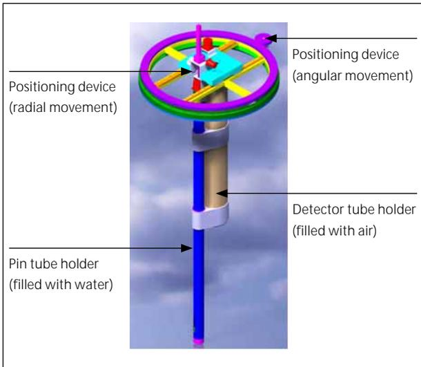
Figure 1: 3D view of the planned measurement station in PROTEUS.
