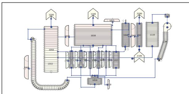
Figure 3: TRACE model of the Phénix primary circuit.
