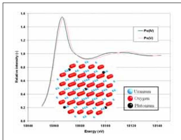
Figure 3: Plutonium L<sub>III</sub> XAFS spectra calculated for the MOX solid solution.
