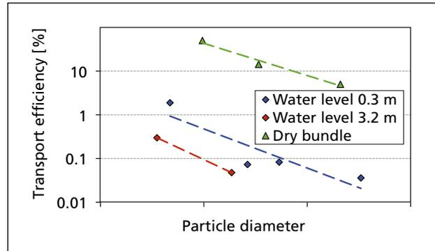
Figure 3: Aerosol transport efficiency in a stream generator bundle under dry and flooded conditions, as measured in the ARTIST facility.
