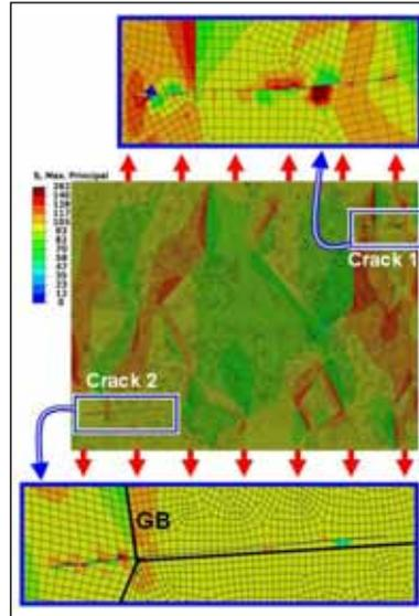
Figure 6: Maximum principal stresses [MPa] and crack growth for combined thermal and (uniaxial) mechanical loading, as predicted using XFEM.
