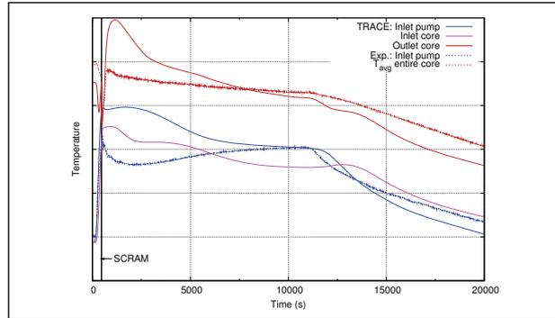
Figure 4: Evolution of the primary circuit temperatures: a comparison between blind predictions and experimental data.
