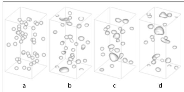
Figure 3: Multiple-bubble simulation at successive times: (a)  $t=0$ ; (b)  $t=0.12$ ; (c)  $t=0.24$ ; (d)  $t=0.36$ . All times in seconds.
