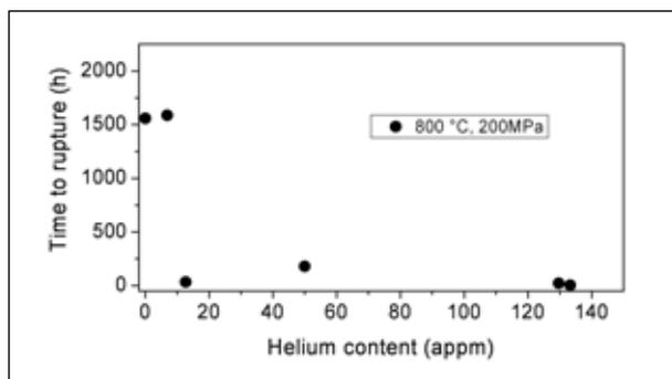
Figure 3: Creep time-to-rupture for samples at 800°C and 200 MPa implanted at up to 1333 appm He.
