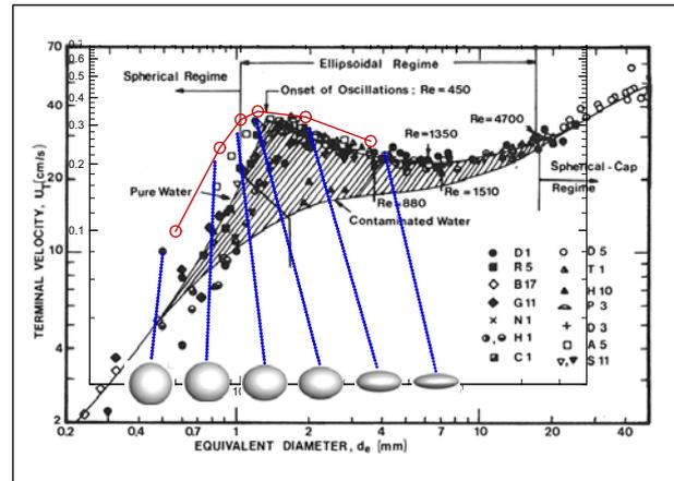
Figure 2: Terminal velocity of air bubbles rising in water. Red circles represent computed values.
