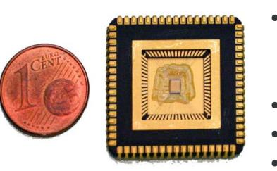
High Voltage Monolithic Active Pixel Sensor • 42x36 pixels • 30x39 µm² pixel size • Binary Readout • Single Threshold
