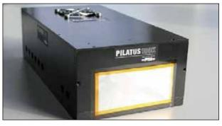
The PILATUS 100K detector box. The active area of the detector is  $84 \times 34 \text{ mm}^2$ .
