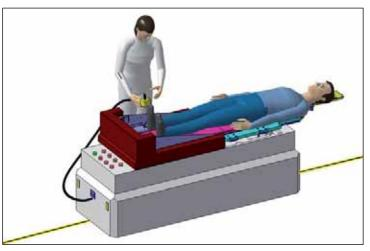
Figure 1: Patient transport system and the optical guidelines.
