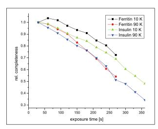
Figure 2: Averaged relative completeness vs. exposure time for insulin and ferritin at 10 K and 90 K.
