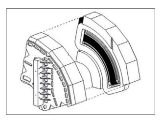
Figure 3: Planned layout of the 90° bending magnet for double parallel beam scanning.
