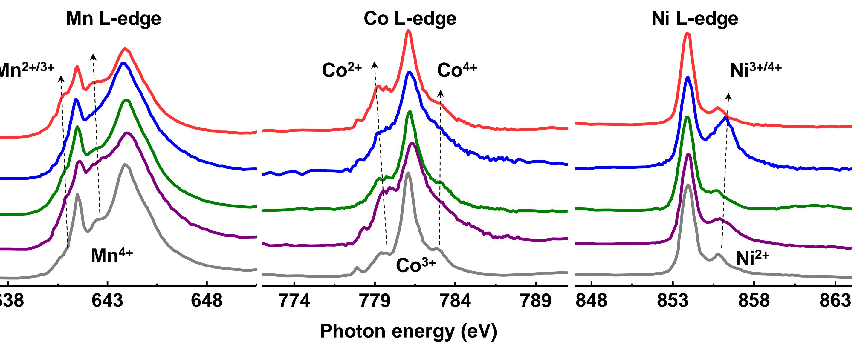
TM oxidation states evolution at surface differs from bulk counterpart
