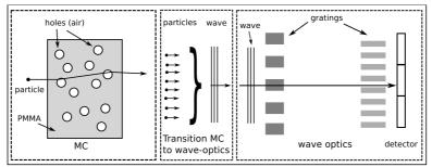
Figure 1: Sketch of the simulation framework
