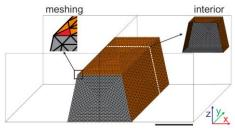
**Fig. 3:** Initial geometry for a reflow simulation of a single line demonstrating the triangular meshing and the soapfilm-approach.
