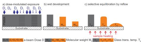
**Fig. 1:** Schematic of the process flow combining electron beam grayscale lithography and polymer reflow for selective pattern equilibration.
