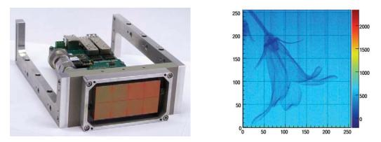
Figure 1: First JUNGFRAU 1.0 prototype module (left), X-ray transmission image of a flower recorded with JUNGFRAU 1.0 (right).
