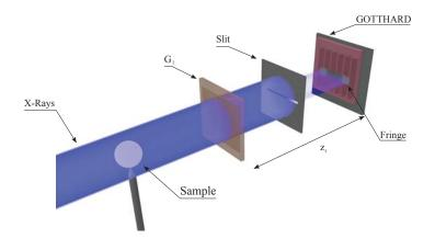
Fig. 1 Setup of the G2-less grating interferometer. The microstrip detector is placed at a distance of zt = 15 cm downstream of the G1. The microstrips have a length of several mm and therefore the beam is additionally collimated by a 2  $\mu$ m tungsten slit directly in front of the sensor.
