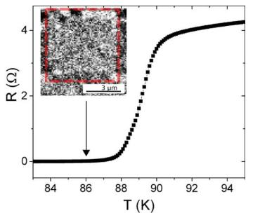
Figure 1: Resistance versus temperature curve of YBCO thin film indicating the Tc of 89 K, Inset: XMCD image of a 6  $\mu$ m Py square taken at 86 K. The square is highlighted with red dashed line, dark cross corresponds to the out-of-plane magnetization component.
