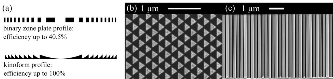
**Fig. 1:** (a): Binary and kinoform phase profiles sketches. (b,c): Scanning electron micrograph of kinoform lenses with 200 nm pitch, showing the (a) top view and the (c) cross section of triangular kinoform elements in silicon.
