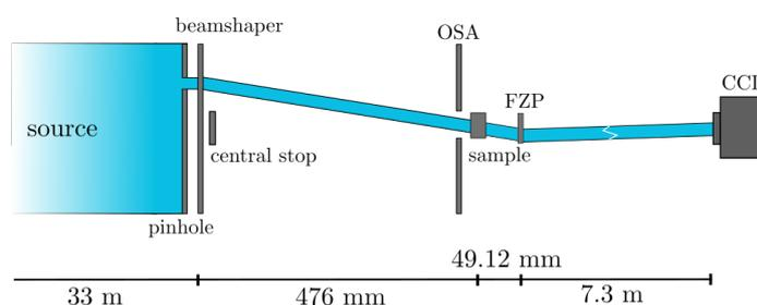
Figure 1: Schematic drawing of a Fourier ptychographic setup at the cSAXS beamline. A 1 mm beamshaper and a 100  $\mu\text{m}$  Fresnel zone plate were used as condenser and objective lens of the X-ray microscope respectively. The condenser was illuminated with a coherent beam at 8.7 keV.
