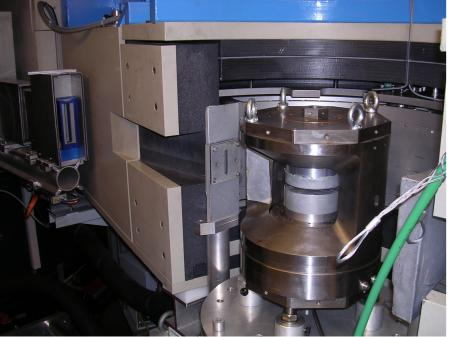
detector shielding + radial collimator + BN anvils + low noise ellectronics = excellent peak to background ratio
