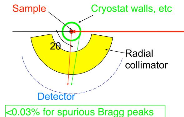
Radial collimator with the shielding.
