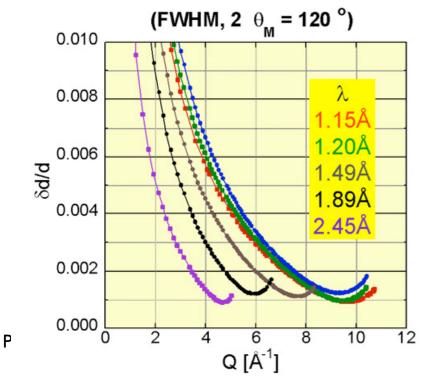
DMC: experimental resolution functions Ad/d (Q,)
