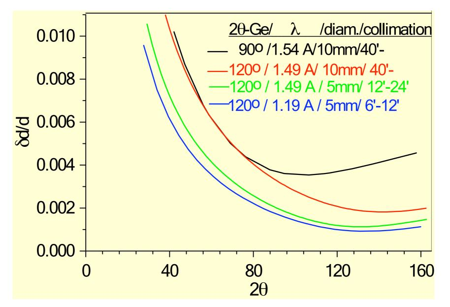
Comparison of resolution functions for different primary-secondary collimations. Typical modes are HI:40'-, MR:12'-24', HR:6'-12'. Counting rates are decreased by a factor of ~3 and ~(8-10) for MR and HR, respectively.
