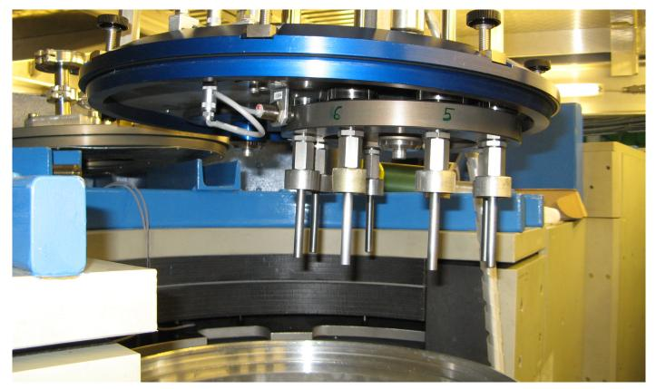
Fully loaded with 8 samples, the sample changer is ready to be installed in-place on the HRPT sample table.
