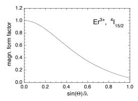
Figure 2: Magnetic form factor for the trivalent rare-earth ion Er<sup>3+</sup> (dipole approximation) with ground state <sup>4</sup>I<sub>15/2</sub>.
