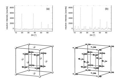
Figure 4: (a) Neutron diffraction pattern (magnetic scattering only) and corresponding magnetic structure in  $Nd_3Pd_{20}Ge_6$  below  $T_{N1} = 1.75$  K. While the Nd moments on one site are antiferromagnetically ordered, the moments on the other site remain disordered. (b) Magnetic neutron diffraction pattern and corresponding magnetic structure below  $T_{N2} = 0.58$  K; also the second Nd sublattice is magnetically ordered.
