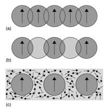
Figure 1: Schematic illustrations of (a) direct exchange, in which the magnetic ions interact because their charge distribution overlap; (b) superexchange, in which magnetic ions with non-overlapping charge distributions interact because both have overlap with the same nonmagnetic ion; and (c) indirect exchange, in which in the absence of overlap a magnetic interaction is mediated by interactions with the conduction electrons.
