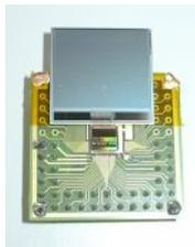
**Fig. 1:** Test structure with the Si-microstrip detector bonded to the MYTHEN readout ASIC.
