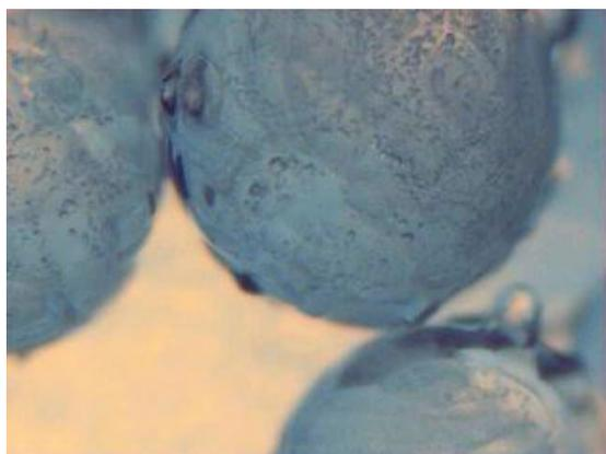
**Fig. 1:** Photo of the produced ice grains with diameters of 700-1000  $\mu\text{m}$ .
