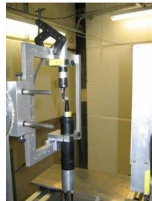
**Fig. 3:** Plastic scintillator detectors on DUT frame.
