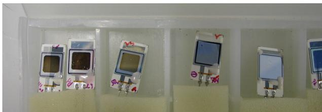
**Fig. 1:** Diodes covered with different materials (Pd, Pt, Au and Al).
