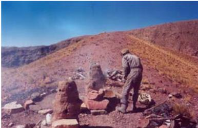
**Fig. 1:** A traditional smelting furnace in use for lead production near Porco, Bolivia (photo B. Mills) [3].
