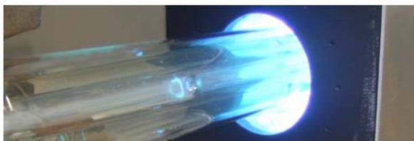
**Fig. 1:** Photolysis reactor. The reactive solution covers the inner wall of a temperature controlled flow tube.
