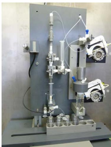
Fig. 1: <sup>44</sup>Sc production semi-automated system.
