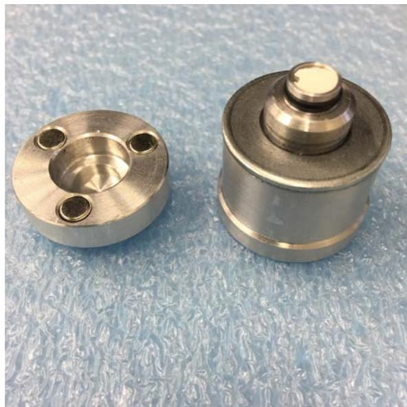
**Fig. 2:** Prototype target shuttle with pellet in place.
