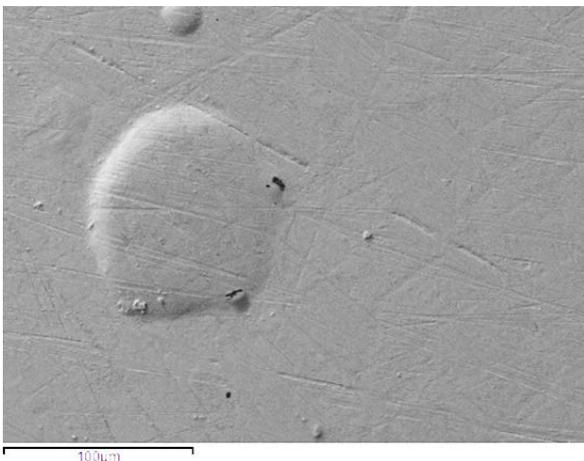
**Fig. 2:** Plateau observed on the surface of a sample processed at 300 °C after grinding and polishing. In the region of the plateau increased Cs and Bi concentrations were detected.
