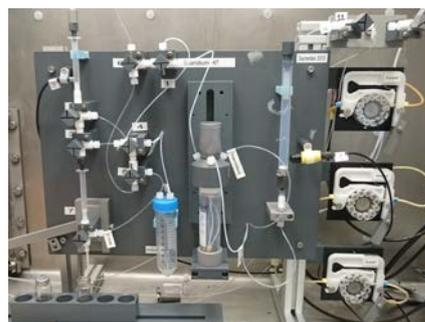
**Fig. 1:**  $^{47}\text{Sc}$  separation panel designed for the operation in the hot-cell.
