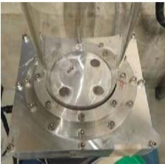
**Fig. 1:** Overview of the irradiation setup. The collimator with 3 open channels is inside a Plexiglas tube used as UCN guide. The rectangular box mounted on the bottom of the tube is the housing of the neutron detector.
