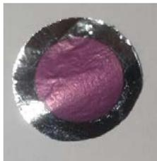
**Fig. 4:**  $\text{AuAl}_2$  (“purple gold”) created by heating 100 nm Au layer on Al backing.
