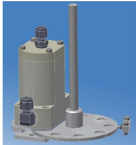
**Fig. 2:** Representation of the new  $^{252}\text{Cf}$  fission source. Most prominent is the wheel containing 8 holes for different stopping foils and a blind position for closing the source. Above the wheel, the reaction chamber with gas in- and outlets is visible. The holder containing the  $^{252}\text{Cf}$  sample is placed directly below the recoil volume. The entire setup is surrounded by a vacuum tight chamber.
