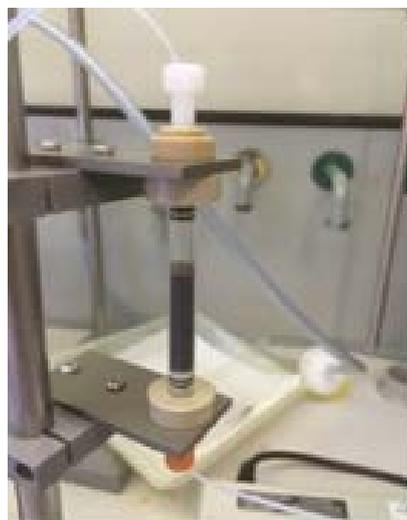
**Fig. 2:** Column setup with use of CLEVASOL for caesium extraction from the radioactive waste solutions.
