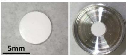
**Fig. 2:** Representative picture of a 6 mm pellet target made of 30 mg CaO as prepared (*left*) and after encapsulation in the aluminum target capsule (*right*).
