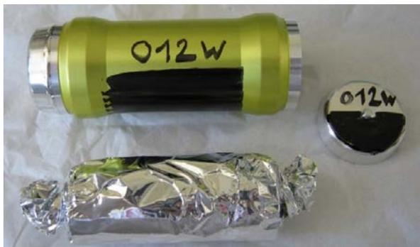
Fig. 1:  $^{166}\text{Ho}$ -MS prepared for irradiation.
