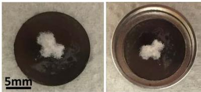
**Fig. 1:** Pelletized target for  $^{44}\text{Sc}$  production as prepared with graphite powder (*left*) and after encapsulation in the aluminum target capsule (*right*).
