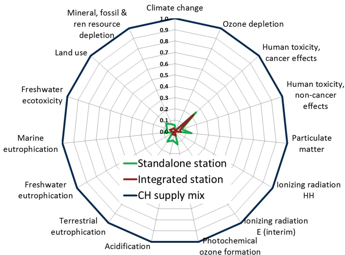
**Figure 7.14: Environmental impact of electricity generated by standalone and integrated SHP power stations, values relative to the average Swiss electricity consumption mix (=1). Impact method: ILCD 2011 Midpoint+ V1.06 / EU27 2010, equal weighting.**
