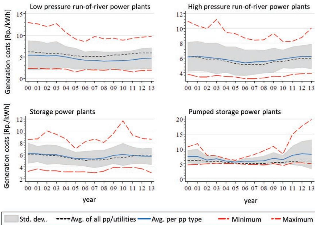
Figure 6.16: Electricity generation costs of current Swiss large hydropower plants between 2000 and 2013, split into different hydropower plant types (Filippini and Geissmann 2014); pp=power plant.
