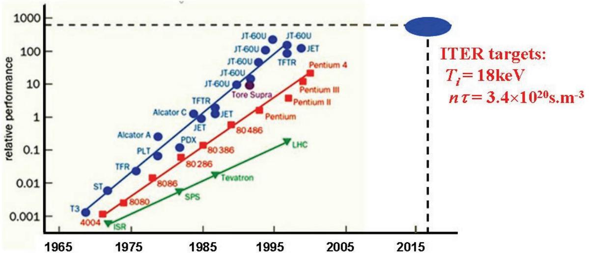
**Figure 17.11: Moore's law type comparing fusion achievement (in blue), Moore's law for semi-conductor devices (in red) and Livingstone law for accelerator (in green) (IAEA 2012a).**
