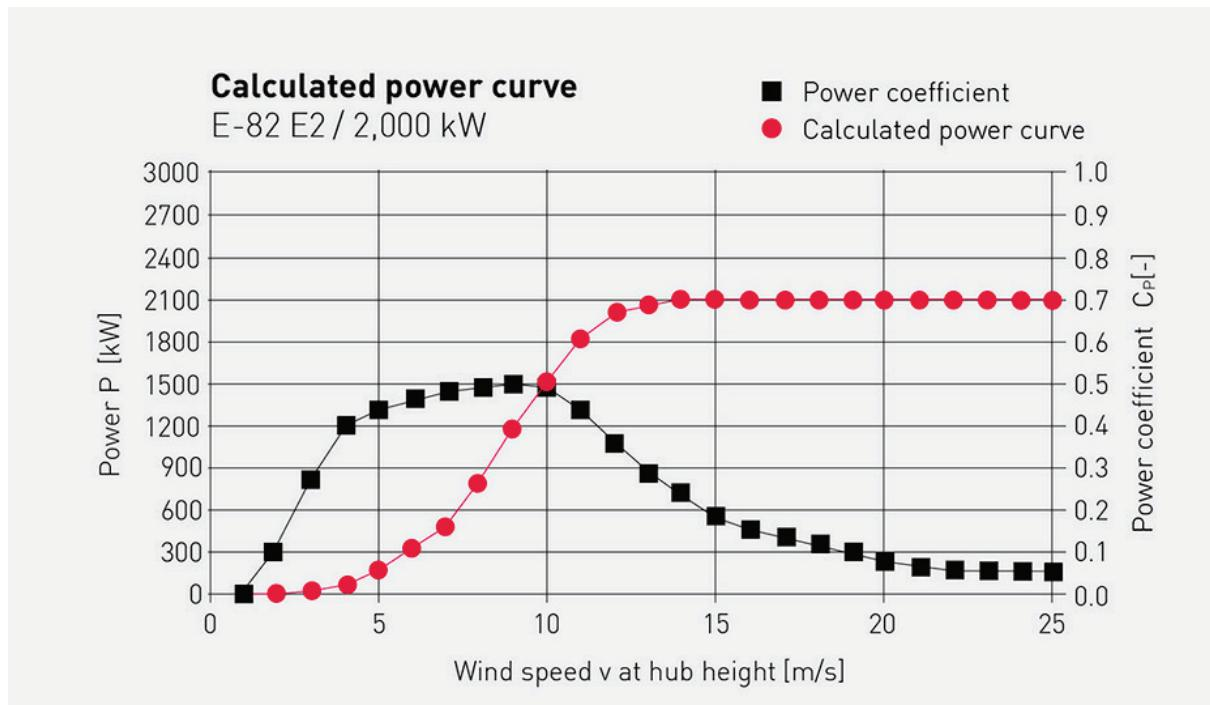
Figure 8.13: Calculated power curve and power coefficient curve for the Enercon E-82 E2 / 2000kW wind turbine.<sup>178</sup>
