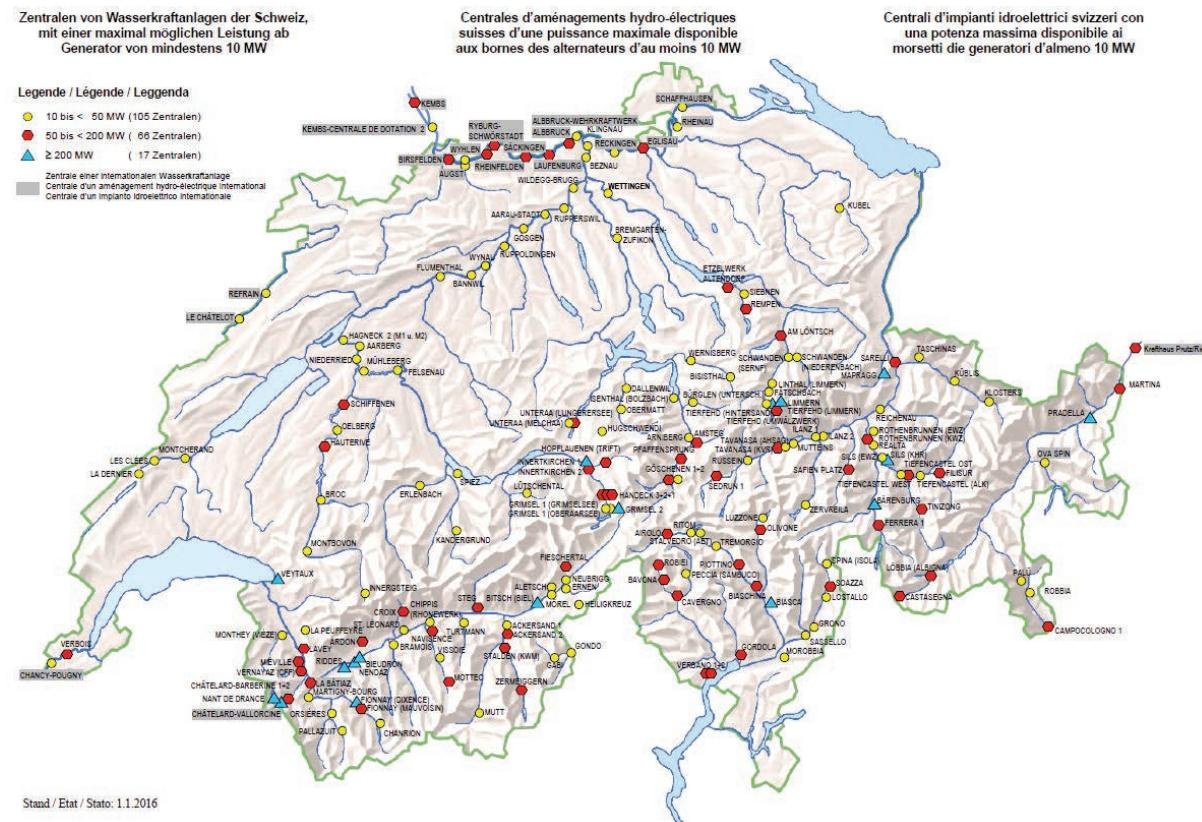
Figure 6.3: Currently operating large hydropower plants in Switzerland, as of 1<sup>st</sup> of January 2016 (BFE/SFOE 2016h).
