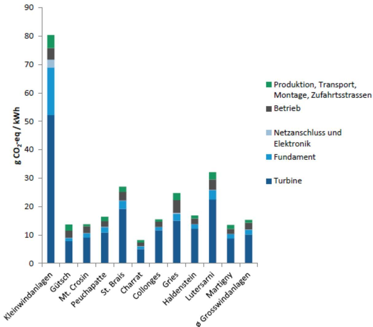
Figure 8.27: Life cycle GHG emissions of electricity from wind turbines in Switzerland. Taken from (Eymann, Stucki et al. 2015).
