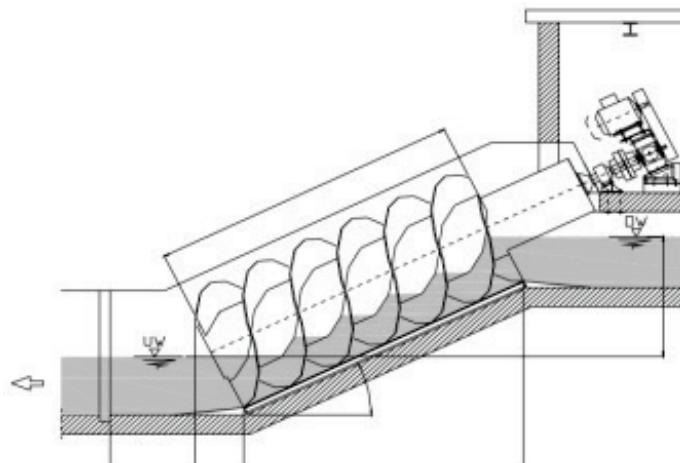
Figure 7.5: Concept of archmiedes screw turbine. Source: (BFE/SFOE 2011).
