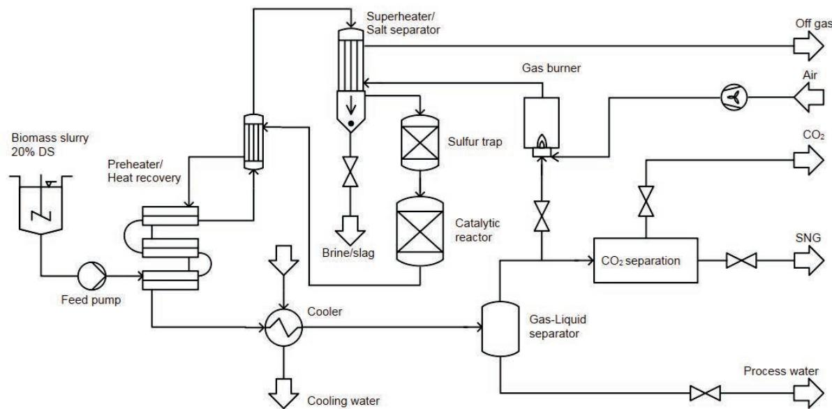
**Figure 17.1: Simplified process flowsheet of PSI's catalytic hydrothermal SNG process. DS = dry solids. SNG = synthetic natural gas.**
