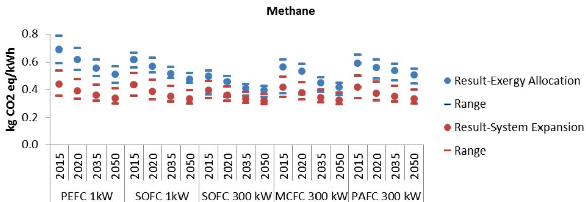
**Figure 16.9: Lifecycle GHG emissions for current and future fuel cells powered by natural gas. Burdens for heat and electricity production are allocated by exergy allocation and system expansion, though quantified per kilowatt-hour of electricity produced.**
