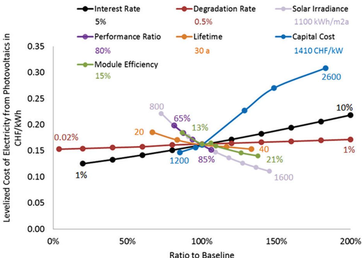
Figure 5.2 Example of sensitivity analysis: LCOE of photovoltaics.
