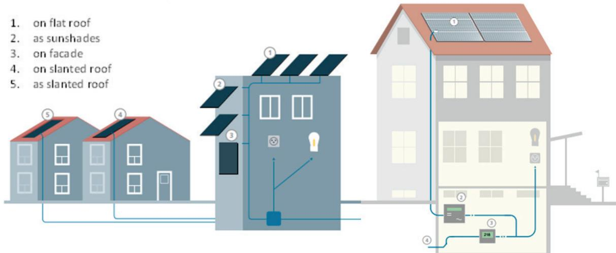
**Figure 9.16: left: Applications of building attached photovoltaics (BIPV) system; right: Grid-connected PV system installation (Swissolar 2014)**
