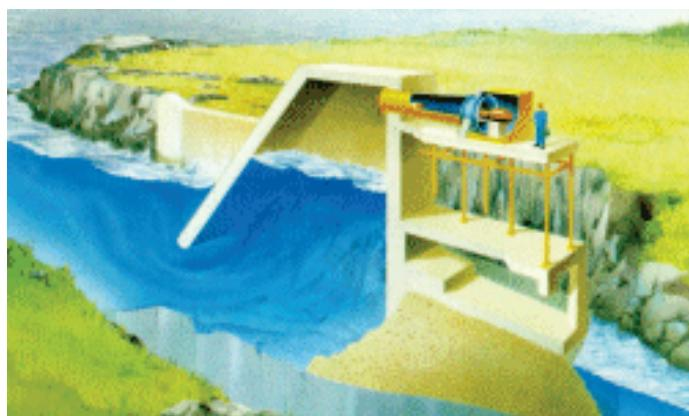
**Figure 12.4: Cutaway Diagram of Oscillating Water Column Design at Islay.<sup>299</sup>**
