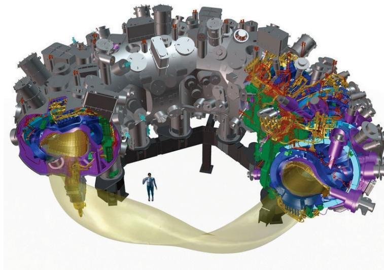
**Figure 17.9:** Schematic of a stellarator, the German Wendelstein 7-X, which was inaugurated in 2016. (Picture Courtesy IPP).
