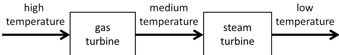
**Figure 15.2 Basic principle of a combined cycle power plant.**
