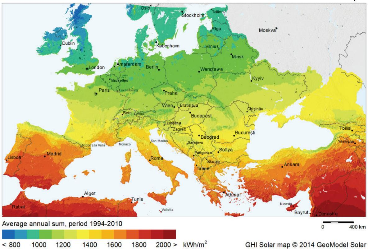
**Figure 9.25: Average European Global Horizontal Irradiation, 1994-2010 (SolarGIS 2014).**
