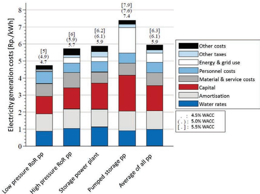
Figure 6.17: Breakdown of average generation costs of current Swiss large hydropower plants in 2013, split into four different categories (Filippini and Geissmann 2014); RoR=run-of-river, pp=power plant.
