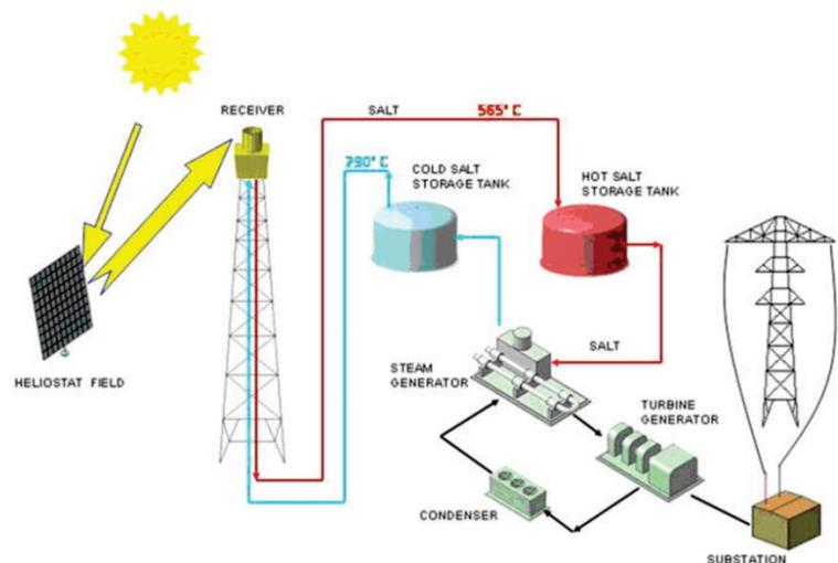
**Figure 13.9: Solar tower power plant with two tank thermal energy storage (TES) using molten salt (Ortega, Burgaleta et al. 2008).**
