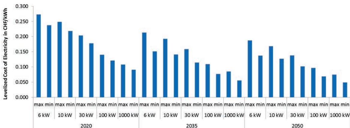
**Figure 9.37: Future leveled costs of electricity from PV power in Switzerland: minimum and maximum values, 2020-2050.**
