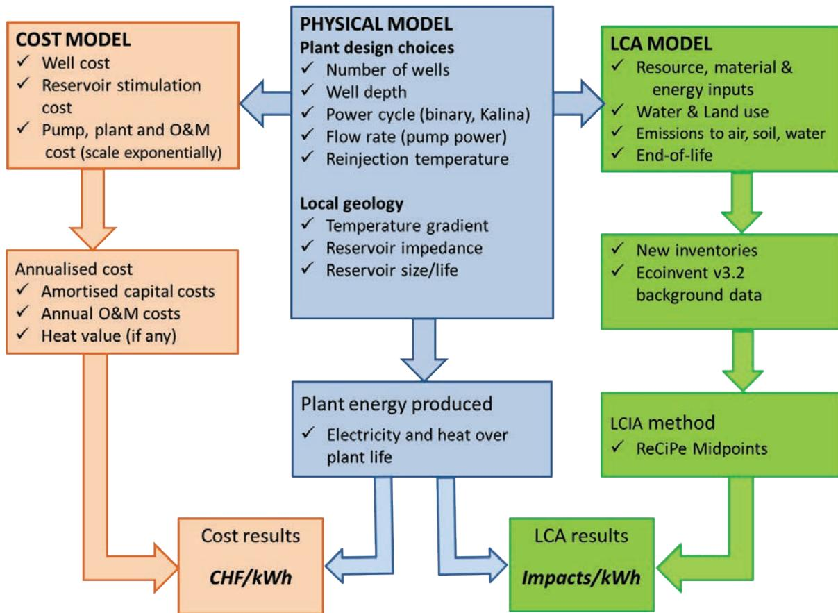
**Figure 11.5: Scheme of the PSI deep geothermal physical model with the coupled cost and LCA parameters (adapted from (Hirschberg, Wiemer et al. 2015))**
