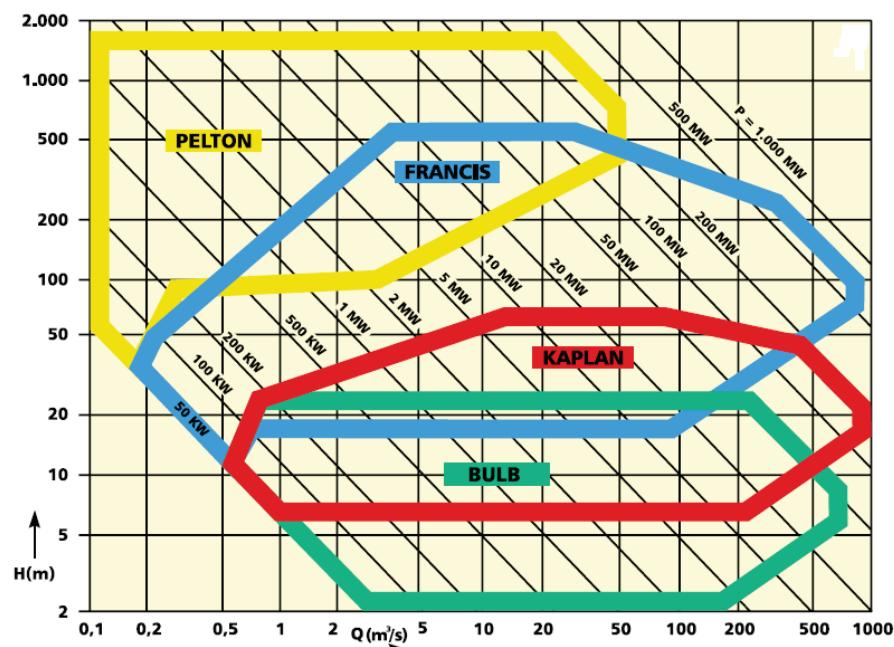
**Figure 7.4:** Optimal efficiency regime, as a function of flow rate and head, for different turbine types.<sup>140</sup>
