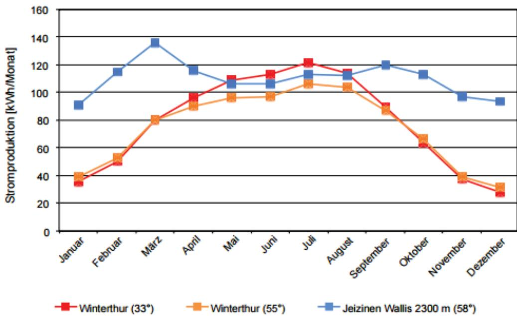
Figure 9.23: Comparison of electricity production from PV systems installed in the Swiss Plateau and the Alps: PV system of 1 kWp power, with 33° and 55° inclined installation in Winterthur (Swiss Plateau), and 58° inclined installation in the Alps at an altitude of 2300 m; Solar irradiance in the Alps is on average about 1320 kWh/m<sup>2</sup> year (WWF 2016).
