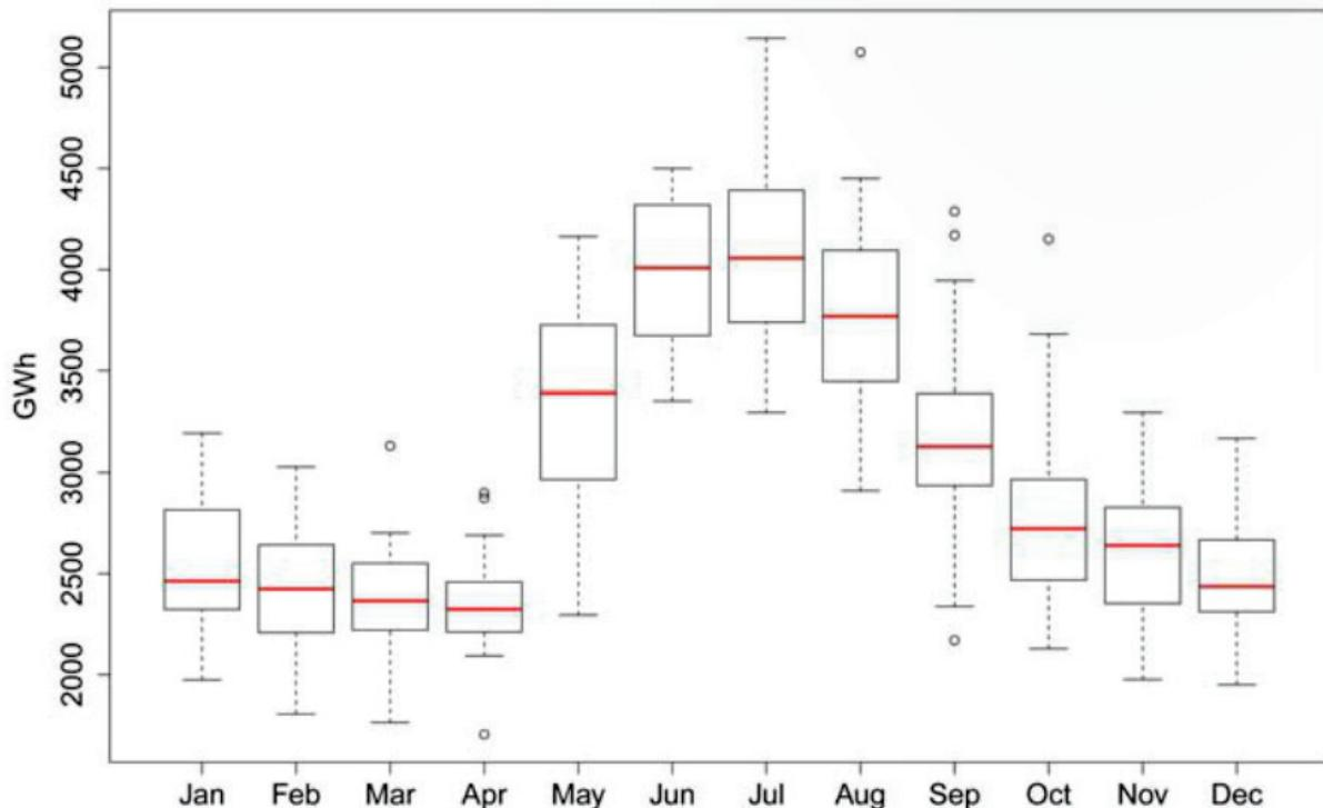
Figure 6.4: Average monthly hydropower generation 1990-2013 (Piot 2014).
