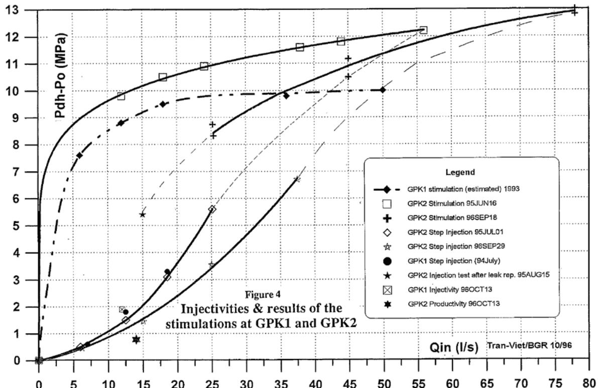
Figure 11.6: Behavior of pressure vs. injection rate at two experimental wells in Soultz-Sous-Forêts (GPK1, GPK2) shown over several years (Gerard, Baumgärtner et al. 1997). For a certain range, the injectivity improved after applying high pressures to the underground.
