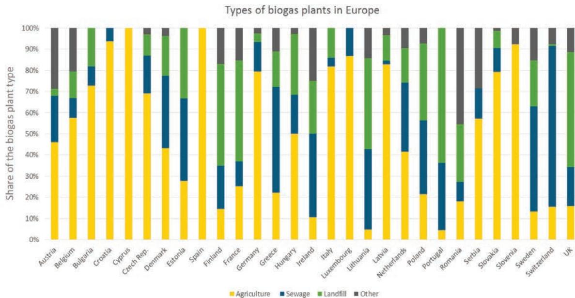
**Figure 10.10: Fraction of biogas plants by feedstock category across Europe. Source: (Štambaský, Prządka et al. 2015).**
