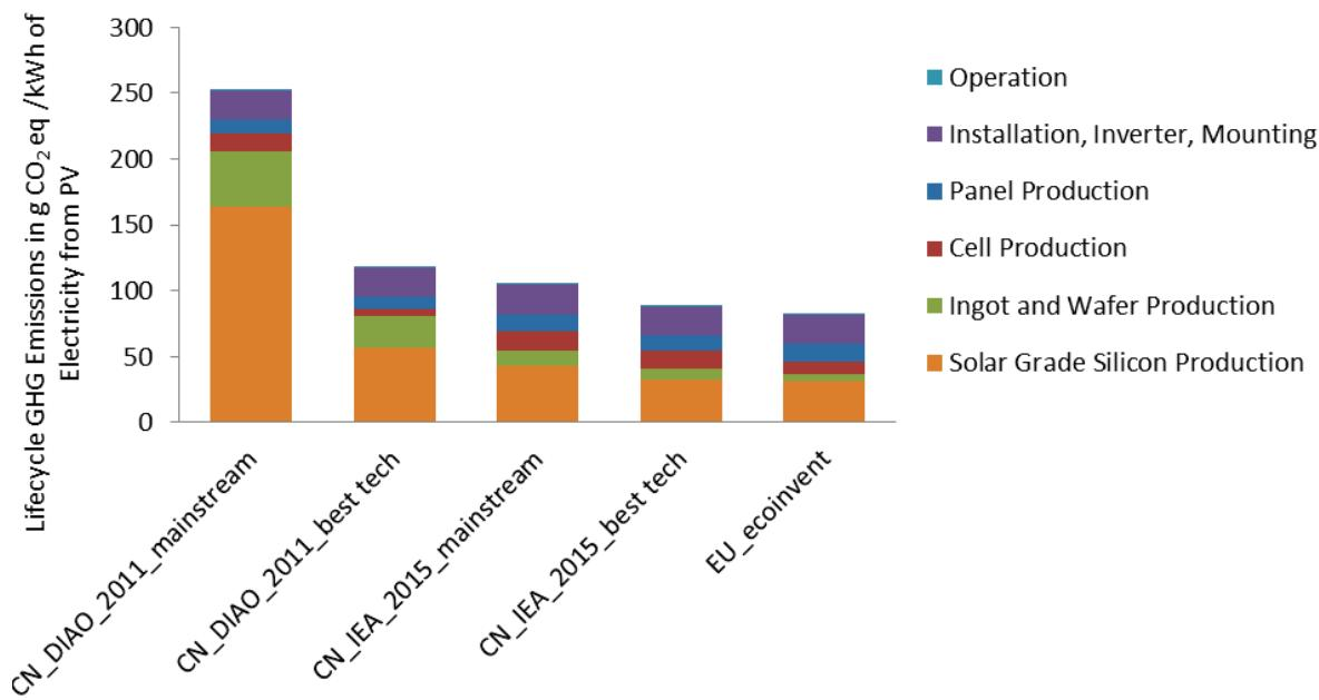
**Figure 9.42: Comparison of GHG emissions based on various sources of Chinese manufactured PV life cycle inventory input (Diao and Shi 2011, Frischknecht, Itten et al. 2015); results based on LCI datasets constructed by PSI referring to the inventory data published, using ecoinvent version 3 (ecoinvent 2014b) as background database.**
