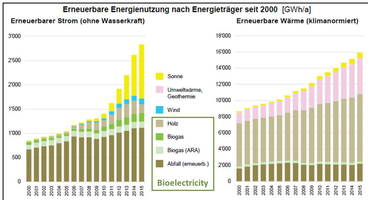
Figure 10.24: Electricity and heat production from renewable resources in Switzerland in the past 15 years.
