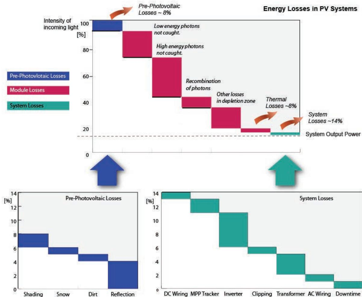
Figure 9.18: Energy losses in PV system: factors reducing the system efficiency (GreenRhinoEnergy 2015).
