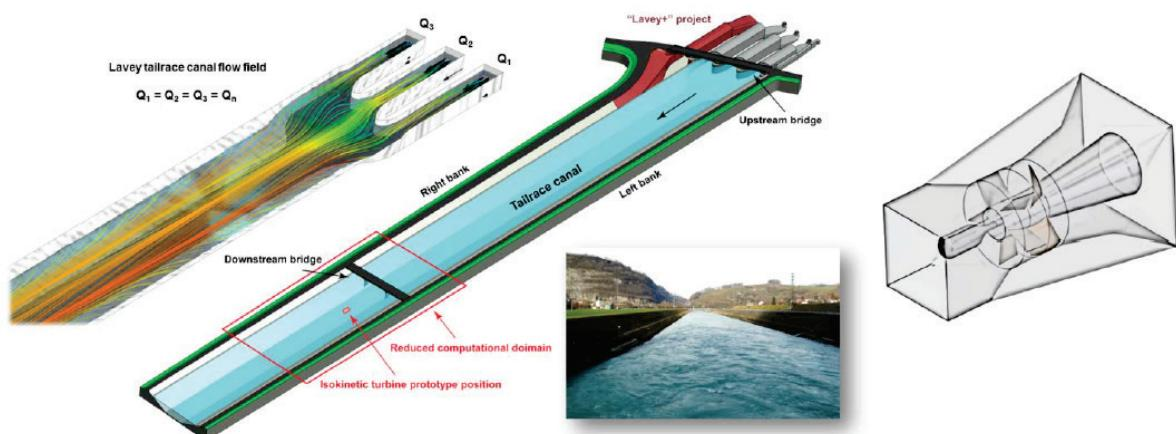
Figure 7.6: Concept of an Isokinetic turbine. Source: <http://www.hevs.ch>
