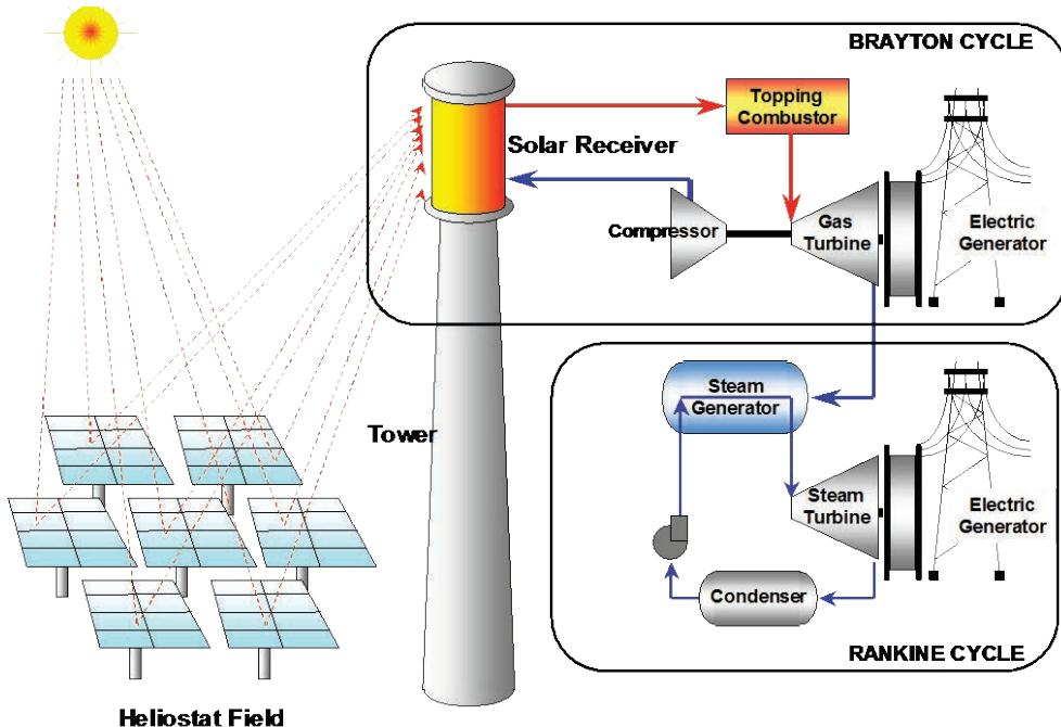
**Figure 13.11:** Highly efficient, solar-driven integrated solar combined cycle (ISCC) power plant. Source: ETHZ/PSI.
