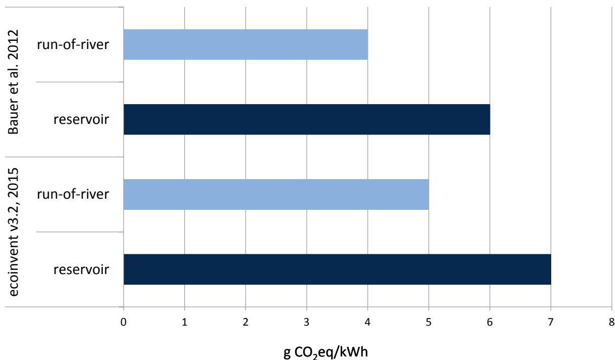
**Figure 6.20:** Life cycle GHG emissions (GWP 100a) due to electricity production at different hydropower plant types in Switzerland (Bauer, Frischknecht et al. 2012, ecoinvent 2015).
