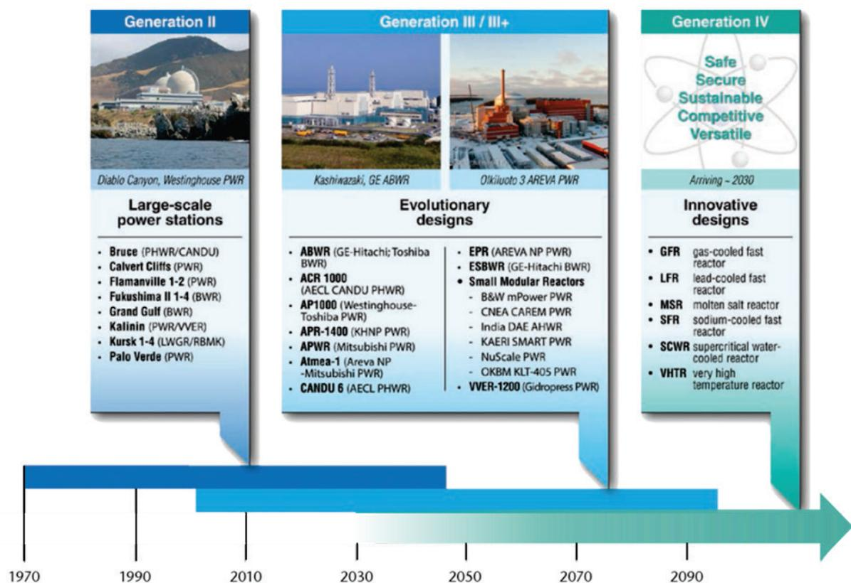
Figure 14.1: Evolution of fission reactor technology; adapted from (OECD/NEA/IEA 2015).
