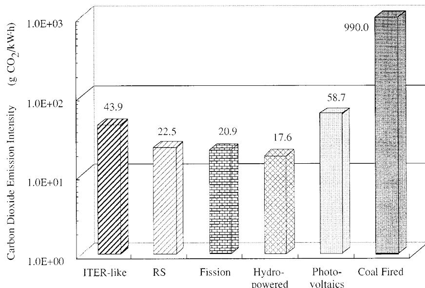
**Figure 17.16: CO<sub>2</sub> emission of a fusion reactor of tokamak type (ITER - like or Reversed Shear RS) (Tokimatsu, Hondo et al. 2000).**
