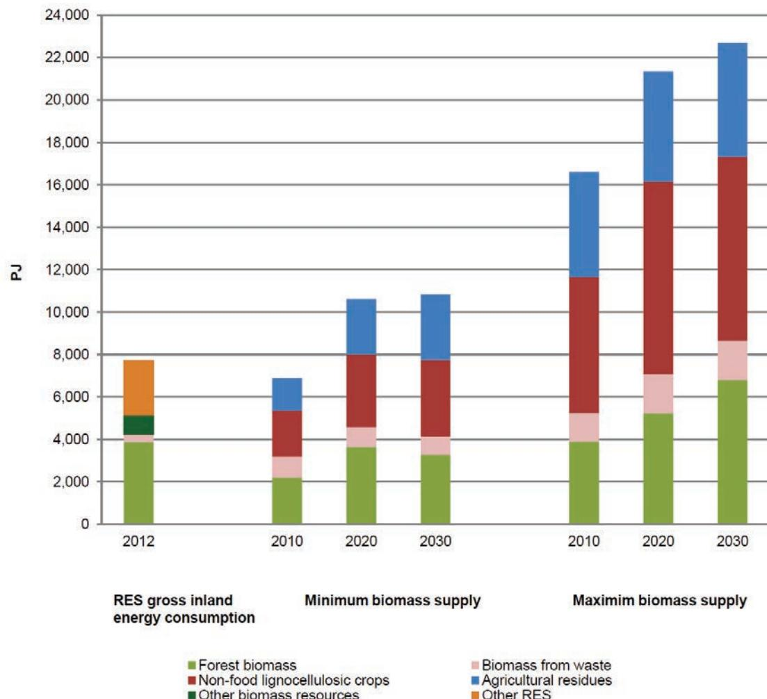
**Figure 10.12: Minimum and maximum estimation values of biomass potential supply for bioenergy use in the EU.** Source: (Khawaja and Janssen 2014).
