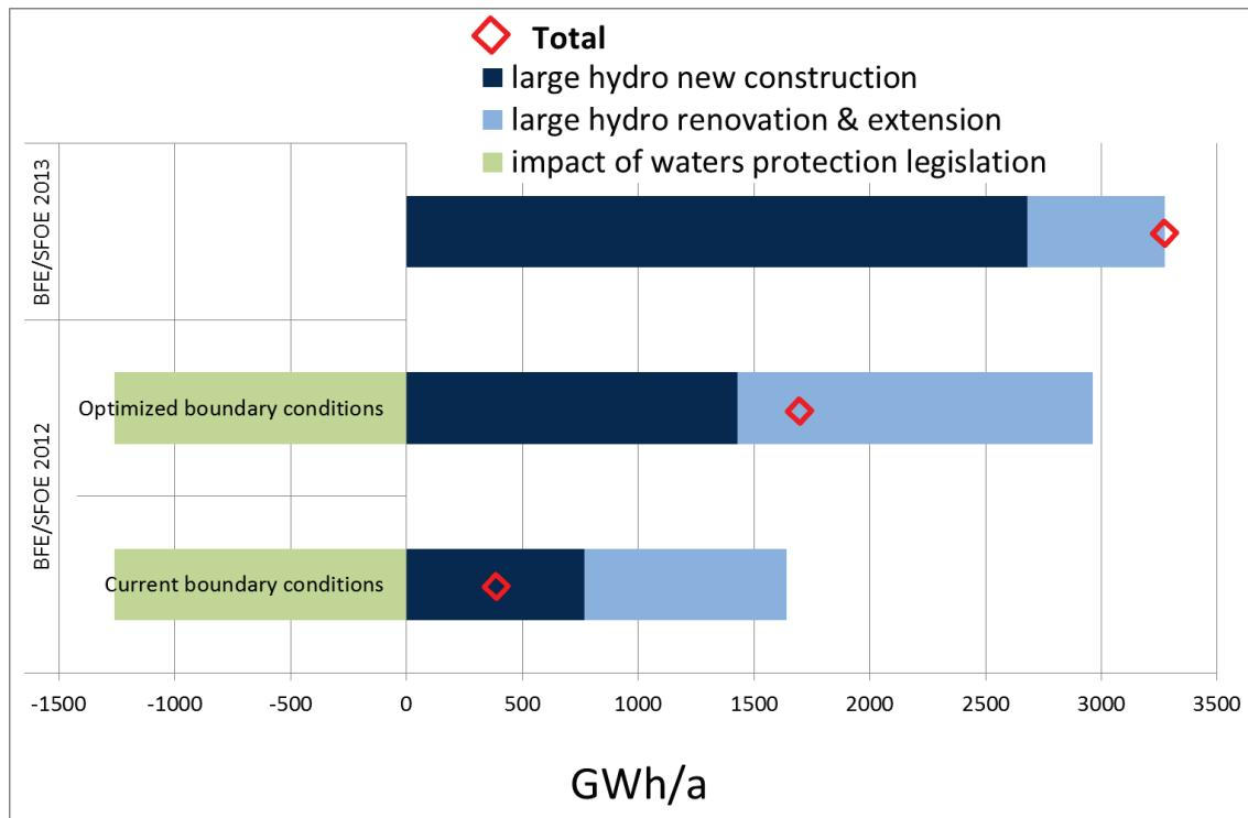
**Figure 6.11: Overview of estimated additional large hydropower potential in Switzerland according to latest evaluations, relating to an expected annual generation of 35.8 TWh/a as of 1<sup>st</sup> of January 2012 (BFE/SFOE 2012b, BFE/SFOE 2013c).**
