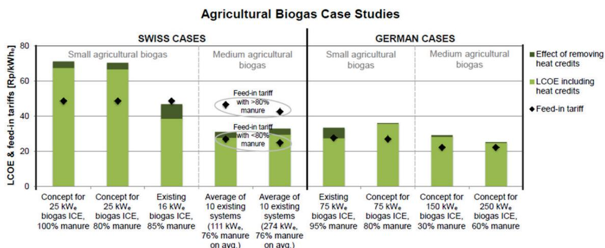
**Figure 10.39: Comparison of the agricultural case studies from Section 10.5.2 with an estimate of the feed-in tariffs that they would receive. Feed-in tariffs in Switzerland are estimated using the online feed-in tariff calculator<sup>229</sup>. Feed-in tariffs in Germany are from (Bakx, Boéchat et al. 2014, Anspach and Bolli 2015, Hari 2015, Stinner, Stur et al. 2015, FNR 2016). Cost structure information is shown in Figure 10.33 and detailed in the appendix of this chapter.**
