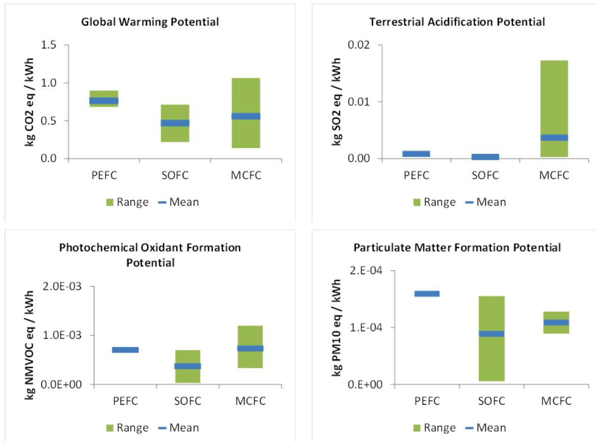
**Figure 16.13: Literature review results for environmental burdens (sources: Table 16.2, environment). The blue line represents the mean of values found in the literature, while the green bar represents the range of values published. Where no green bar is present, this is because there was only one value found in the literature. No values were found for PAFC fuel cells.**
