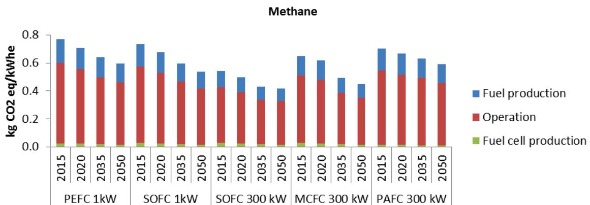
**Figure 16.7: Lifecycle GHG emissions for current and future fuel cells powered by natural gas. Burdens for heat and electricity production are unallocated, though quantified per kilowatt-hour of electricity produced.**
