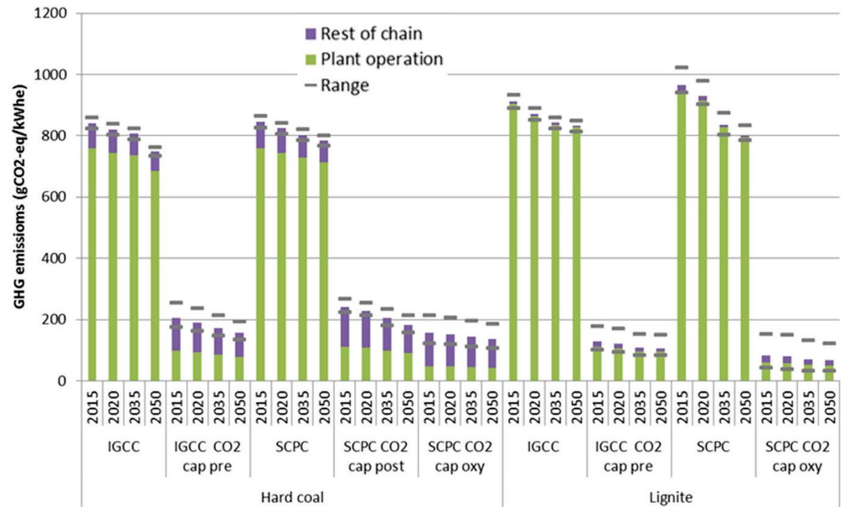
Figure 15.21: Estimated greenhouse gas emissions of coal power plants until 2050.
