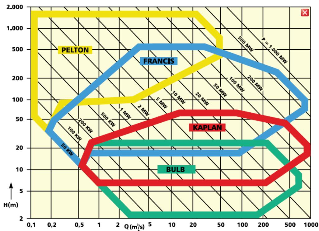
Figure 6.6: Application of different turbine technologies, depending on useable water head and flow rate.<sup>130</sup>
