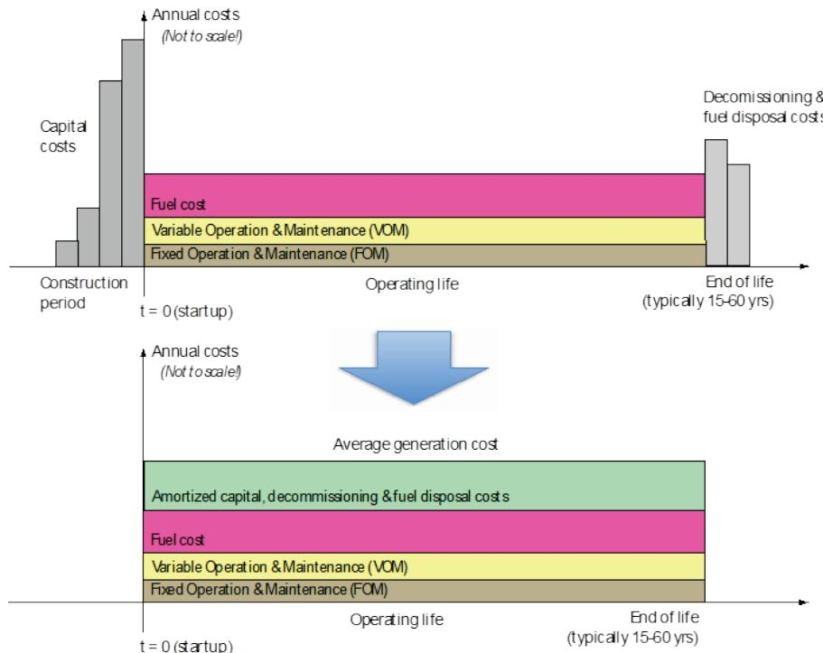
**Figure 5.1: Scheme of LCC methodology, resulting in average generation costs per kWh of electricity, equal to “Levelized Cost of Electricity - LCOE”.**
