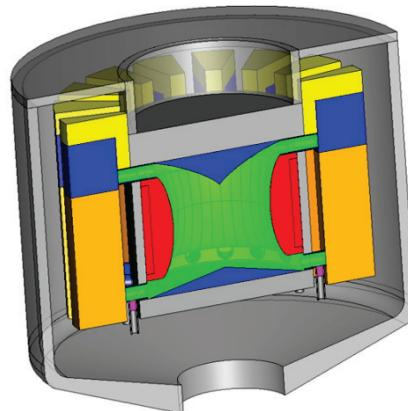
**Figure 14.3: Lay out of conceptual Molten Salt Fast Reactor (MSFR), reference design of the EU SAMOFAR project, with the fluoride-based fuel salt in green and the fertile blanket salt in red (GIF 2014).**
