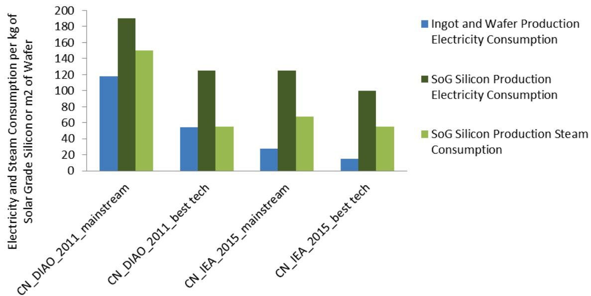
**Figure 9.43: Comparison of electricity and steam consumption in manufacturing of wafer and SoG silicon in China based on various sources (Diao and Shi 2011, Frischknecht, Itten et al. 2015).**
