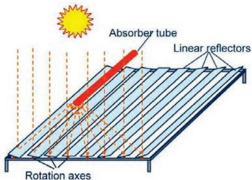
Figure 13.7: Schematic of Linear Fresnel Reflector system (SolarPACES 2016a).
