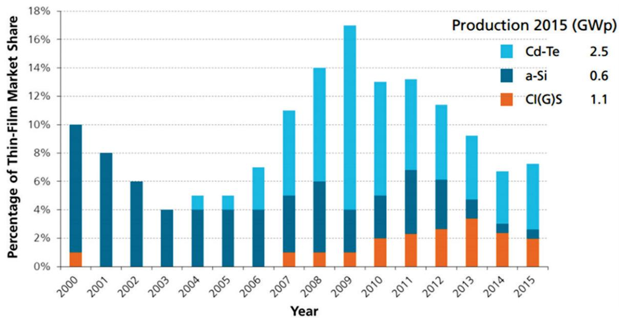
Figure 9.12: Thin-film PV market share from 2000 to 2015 (Fraunhofer 2016).
