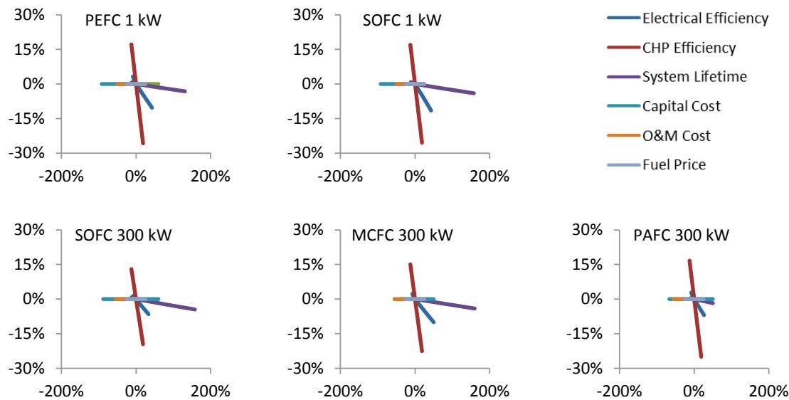
**Figure 16.12: Greenhouse gas sensitivity analysis results calculated with system expansion allocation. The x axis shows the variation in input parameters, while the y axis shows the variation in results.**
