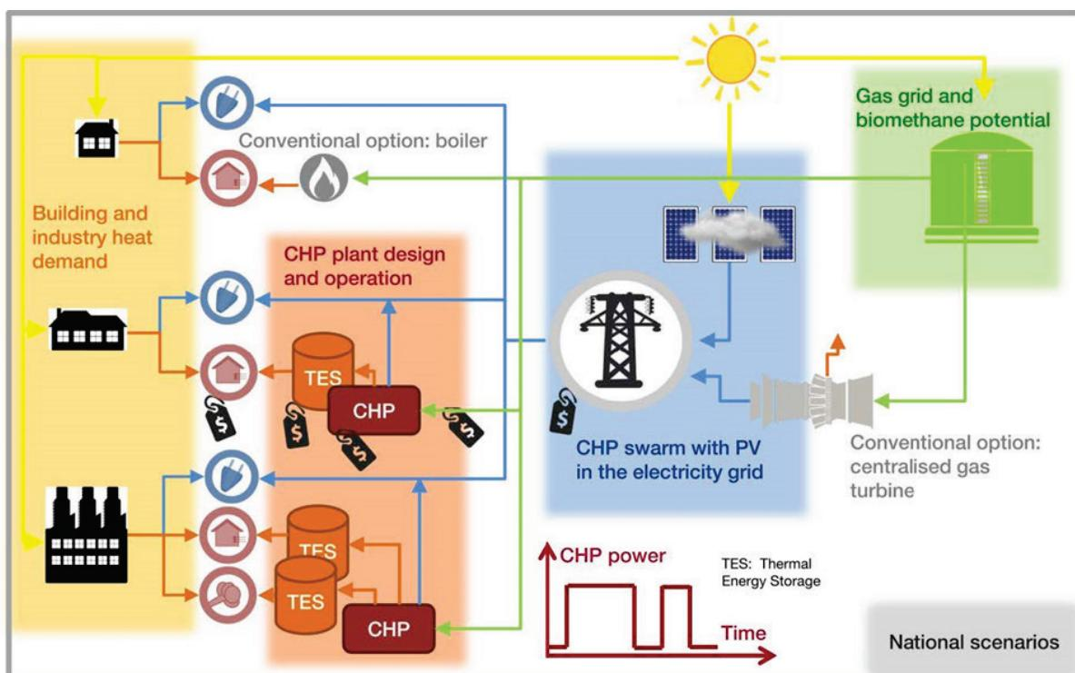
**Figure 10.47: Operational strategy of the biomass swarm. Centralised swarm controller, local storage of heat and balancing the electrical grid on demand (Vögelin, Georges et al. 2016).**
