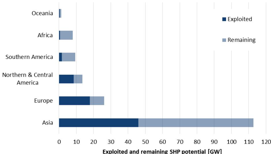
**Figure 7.9: Global distribution of used and unused SHP potential.** Source: (Liu, Masera et al. 2013).
