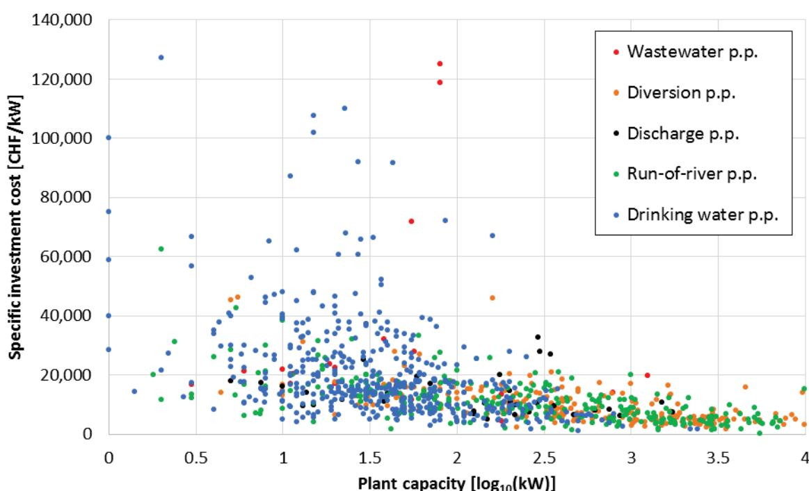
**Figure 7.11: Specific investment cost as a function of installed capacity for different power plant types (BFE/SFOE 2016b).**
