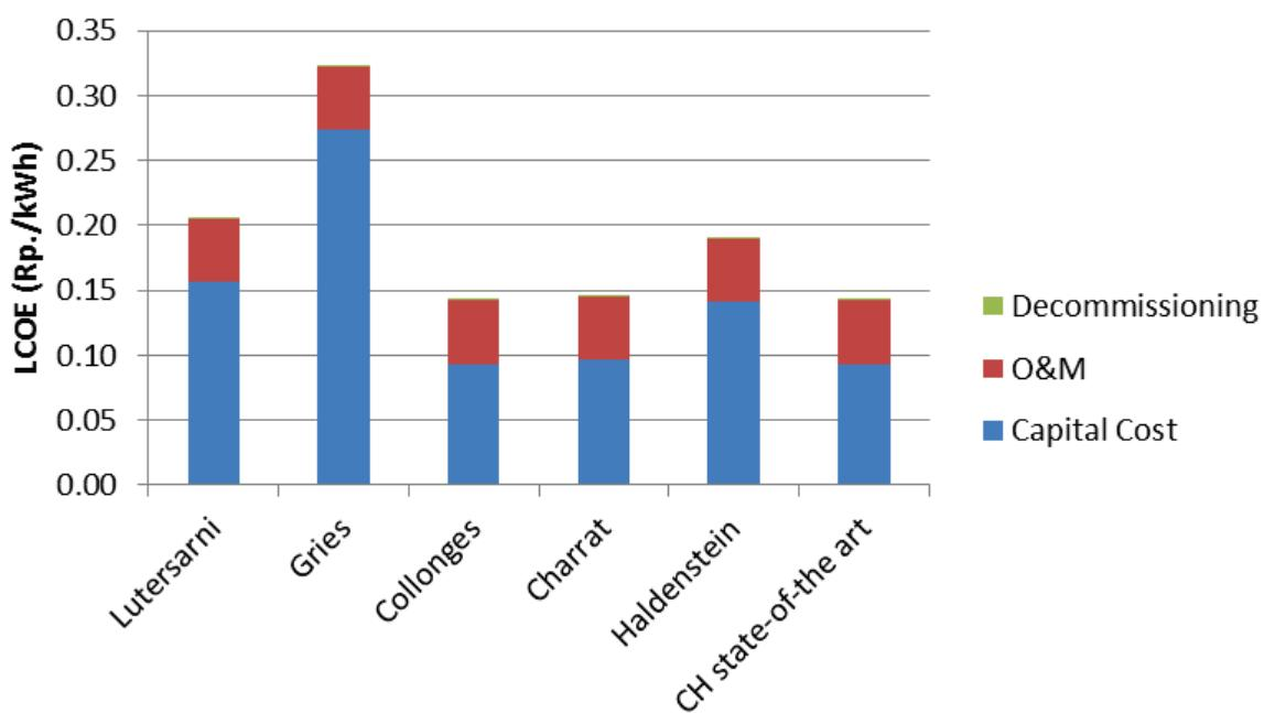
**Figure 8.23: LCOE of Swiss case studies for selected locations in Switzerland, including a theoretical average Swiss case and a state-of-the-art Swiss case, calculated with an annual degradation rate of 1.2%.**
