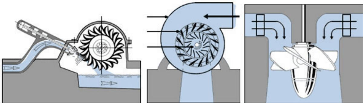
**Figure 7.3:** Schematic representation of a Pelton (left), Francis (middle) and Kaplan (right) turbine. Source: (Hirschberg, Bauer et al. 2005).
