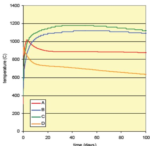
**Figure 17.14: Temperature evolution in reactor after shut down in case of loss of coolant after a shutdown (EFDA 2005).** The temperature does not exceed the melting temperature of structural materials.
