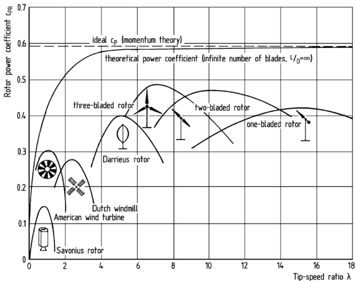
Figure 8.10: Power coefficients of wind rotors of different designs. Taken from (Hau 2013).
