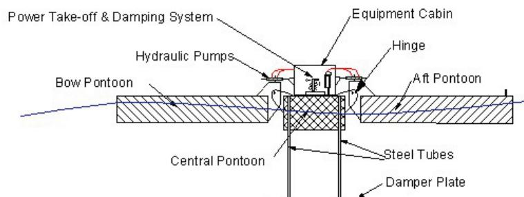
**Figure 12.9: Schematic Diagram of McCabe Wave Pump Design.**<sup>305</sup>
