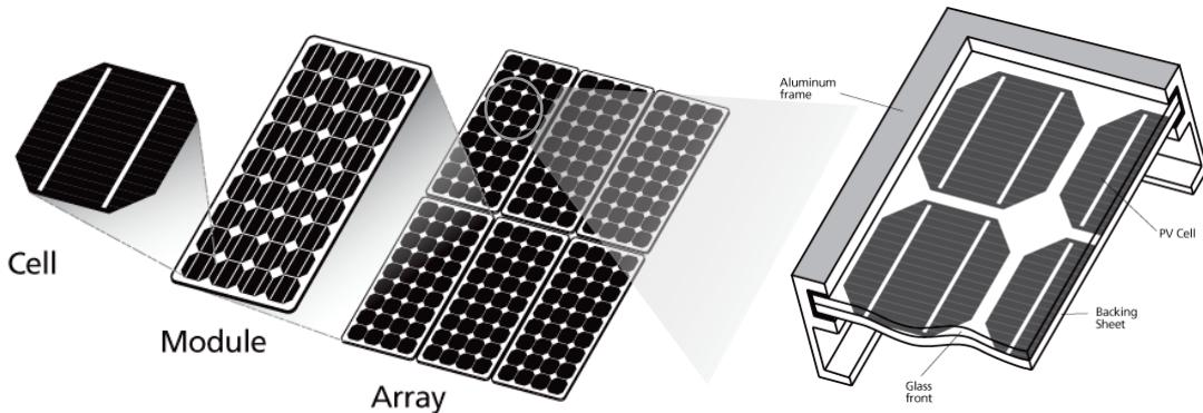
Figure 9.17: PV cell, module and array (Samlexsolar 2015).
