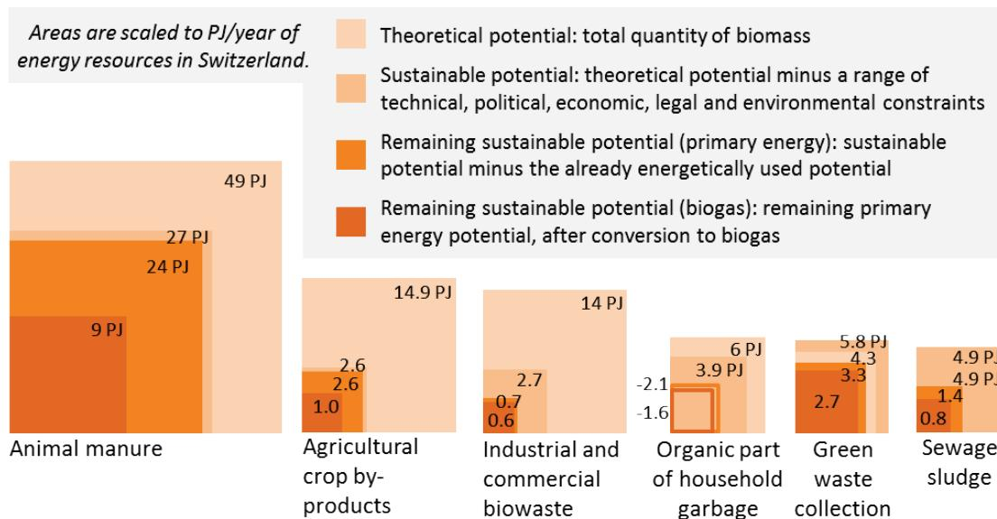
**Figure 10.18: Potentials of domestic non-woody biomass resources in Switzerland, from (Burg, Bowman et al. in preparation, status: 2.2.2017).**
