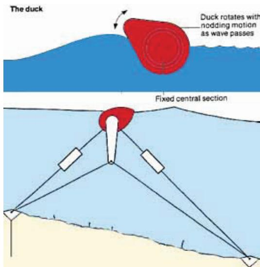
**Figure 12.7: Schematic Diagram of Salter Duck Design.**<sup>302</sup>
