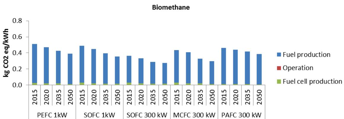
**Figure 16.8: Lifecycle GHG emissions for current and future fuel cells powered by biomethane from sewage gas. Burdens for heat and electricity production are unallocated, though quantified per kilowatt-hour of electricity produced.**
