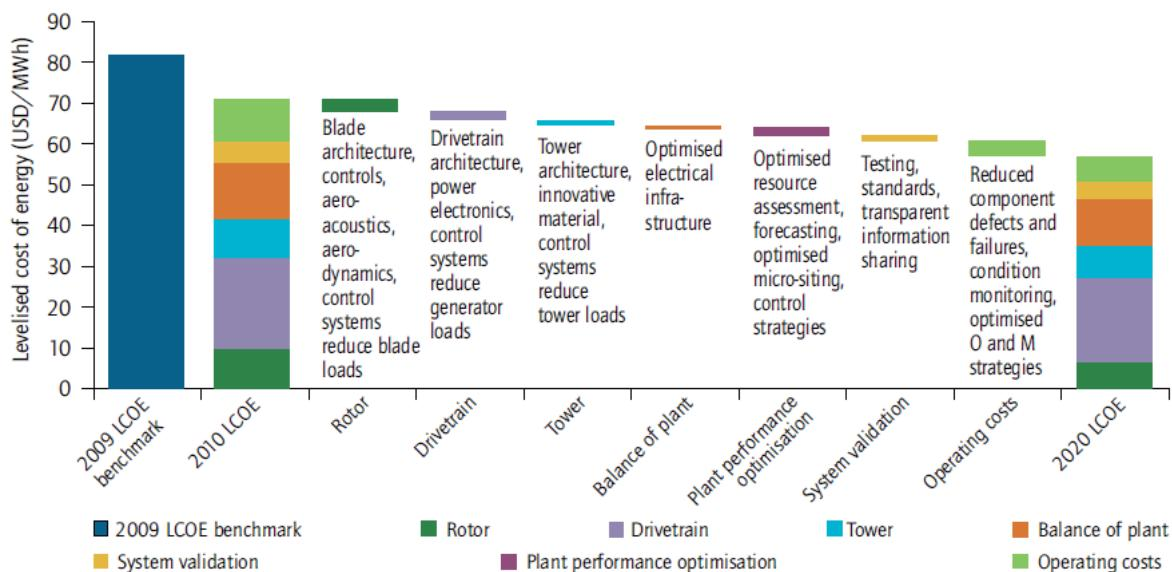
**Figure 8.25: Target for cost reductions of onshore wind power in the United States (IEA 2013a).**
