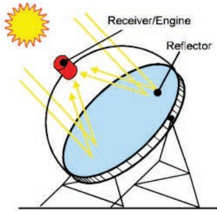
Figure 13.8: Schematic of parabolic dish concentrator system (SolarPACES 2016a).
