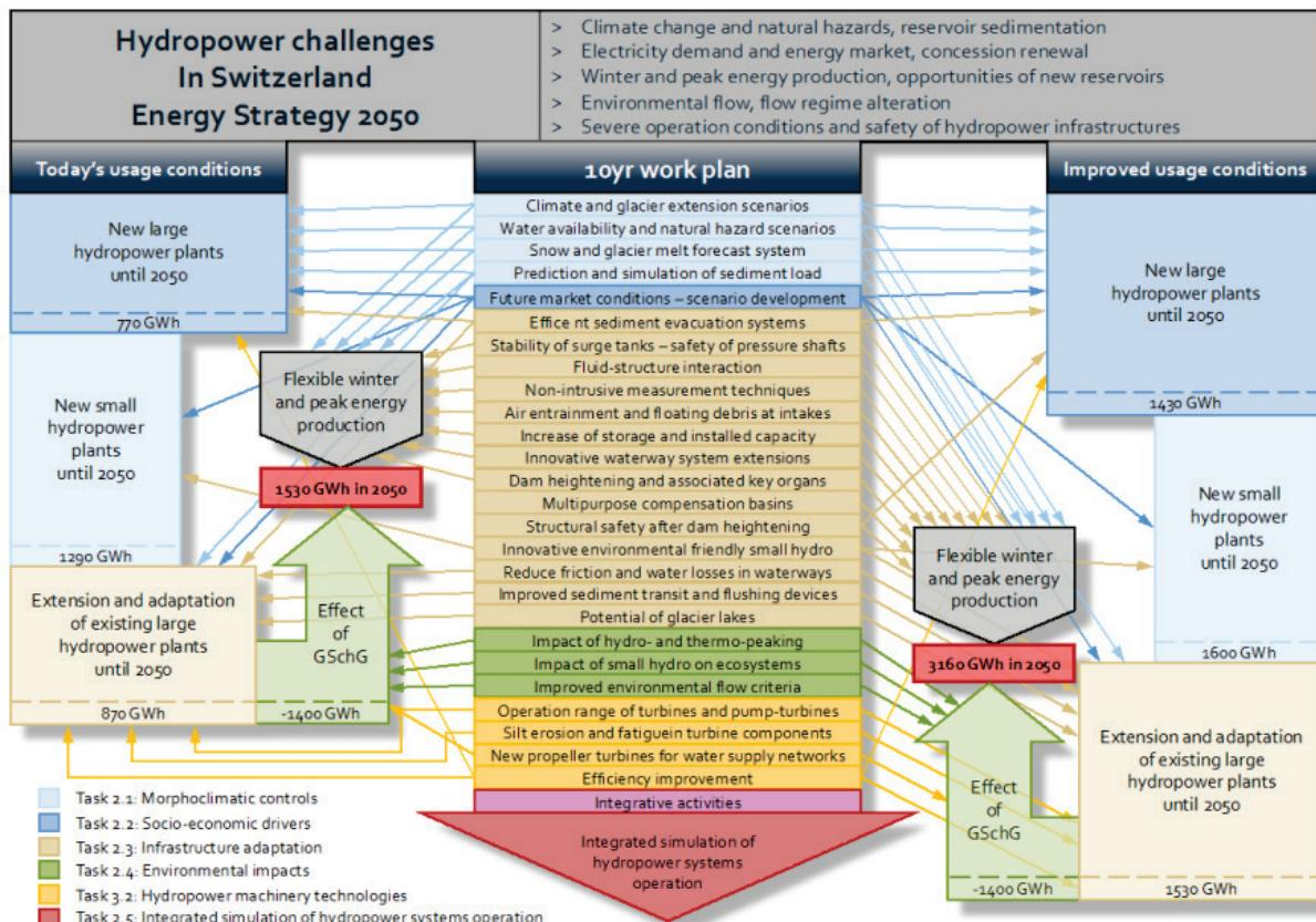
Figure 7.7: Research and development roadmap for hydropower in Switzerland. Source: (SCCER-SoE 2015)
