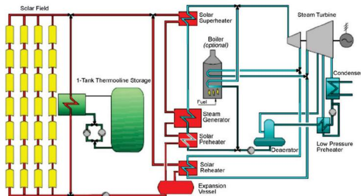
**Figure 13.12: Parabolic trough plant with one tank thermocline storage, e.g. from a packed bed (Gil, Medrano et al. 2010).**
