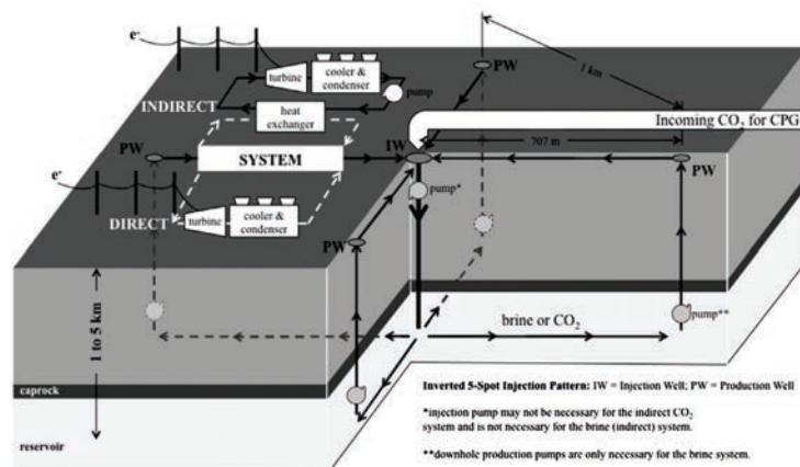
**Figure 17.5: Schematic illustrating both a direct and an indirect CO<sub>2</sub>-Plume Geothermal (CPG) system (Figure from (Adams, Kuehn et al. 2015)).**
