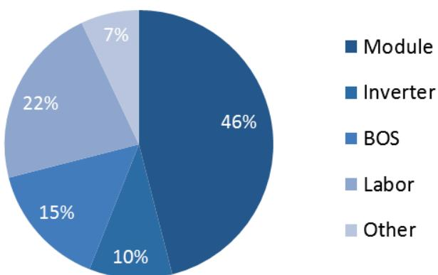
**Figure 9.31: Average breakdown of capital cost for Swiss PV systems (Perch-Nielsen, Märki et al. 2014).**
