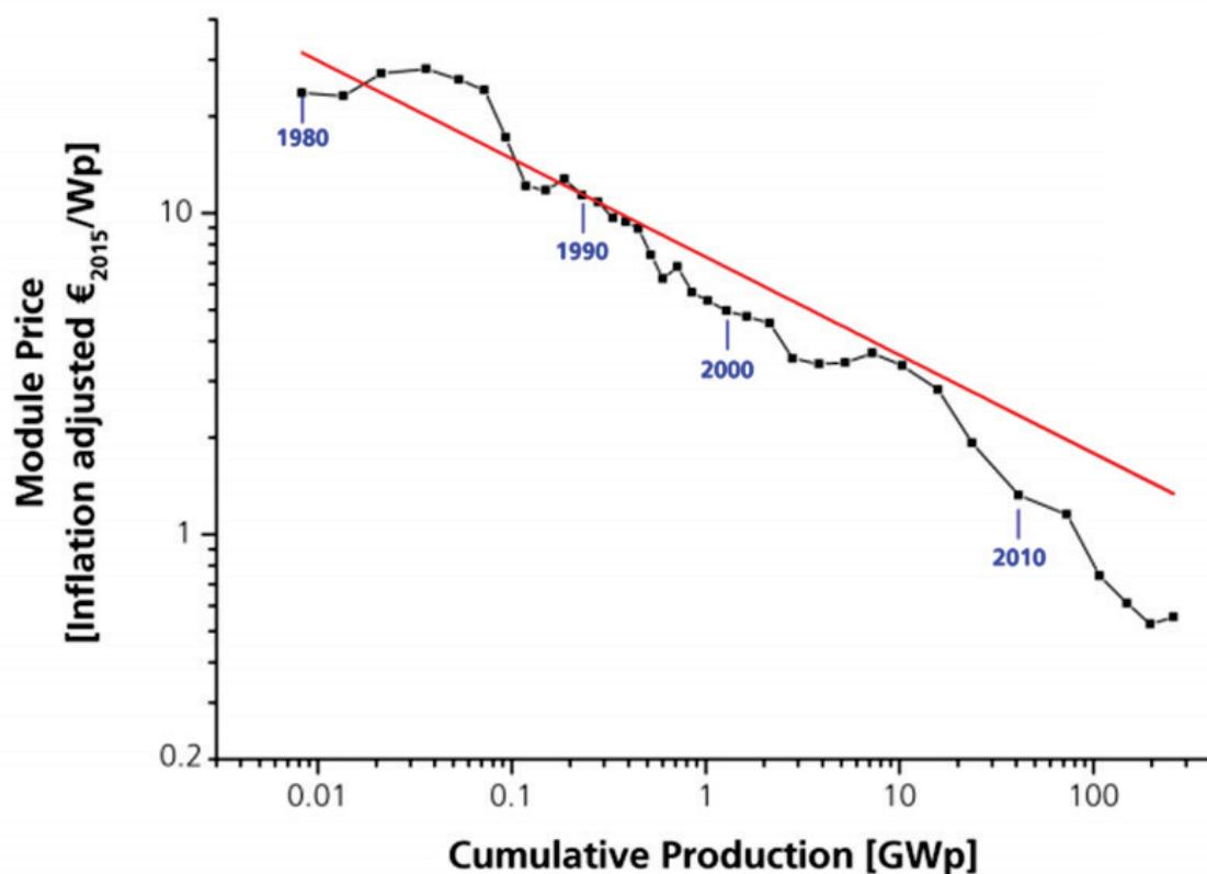
Figure 9.28: Module price learning curve from 1980 to 2015 (Fraunhofer 2016).
