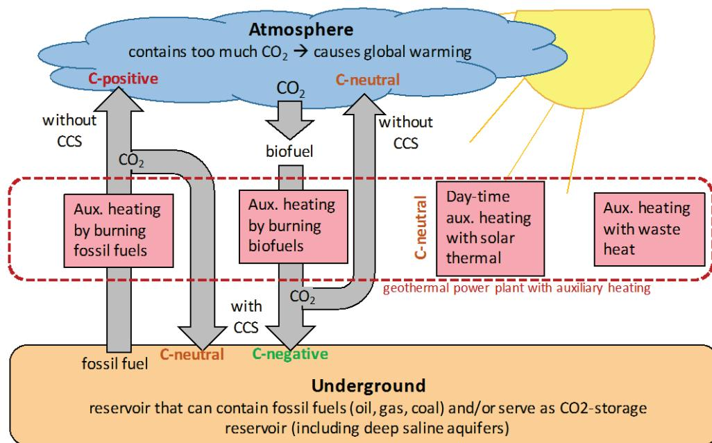
**Figure 17.7: Auxiliary heating of geothermally preheated geofluids (water, brine, CO<sub>2</sub>, etc.). Depending on the type of auxiliary, secondary heating source employed, the system may be carbon-positive, or carbon-negative.**
