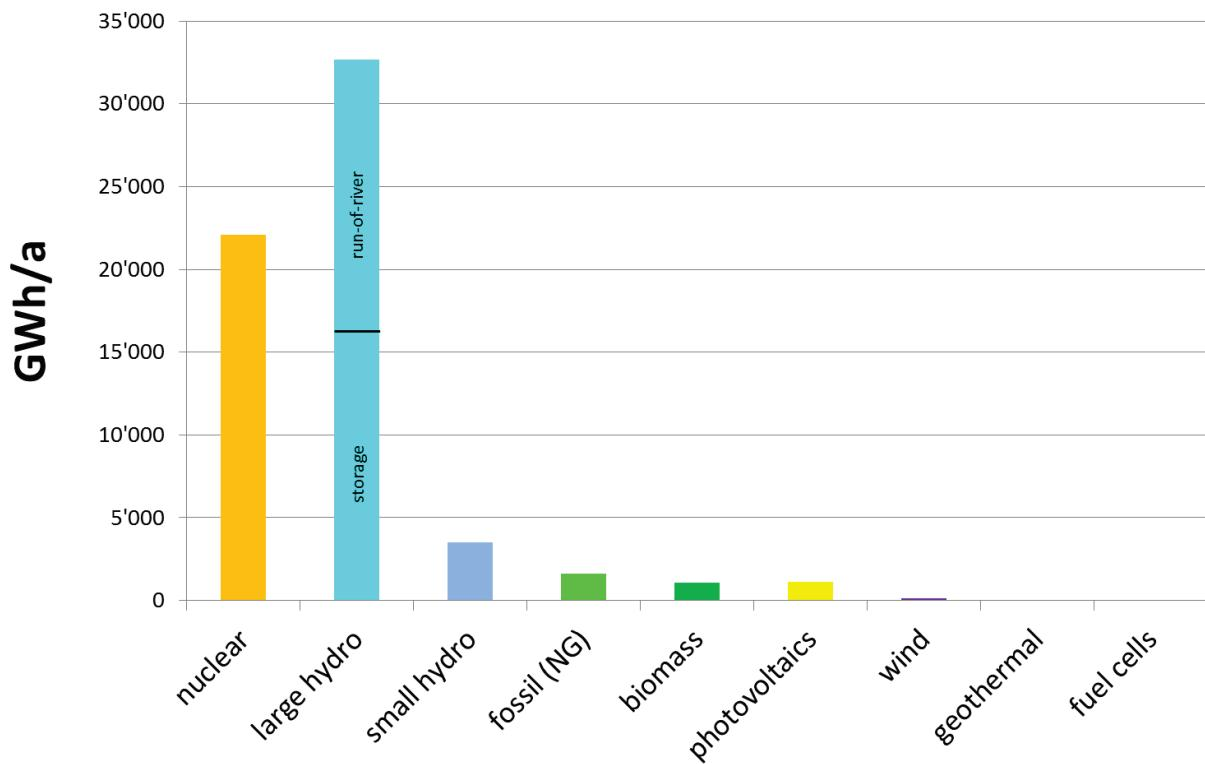
**Figure 1.1: Electricity generation in Switzerland in year 2015 (BFE/SFOE 2016e, BFE/SFOE 2016g).**
