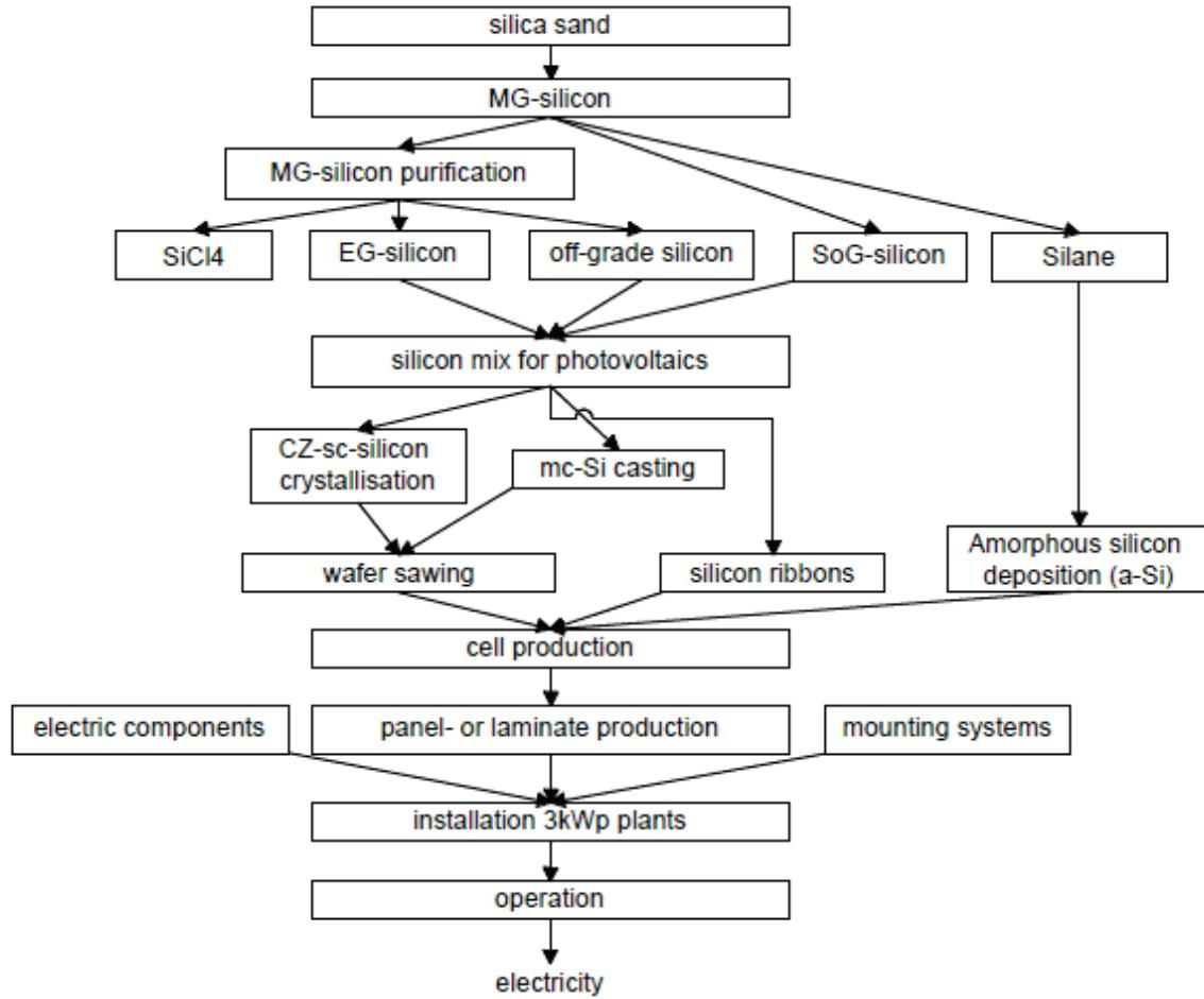
**Figure 9.39: Process system in the LCA of PV. Different sub systems investigated for the production chain of silicon cells based photovoltaic power plants installed in Switzerland. MG-silicon: metallurgical grade silicon, EG-silicon: electronic grade silicon, SoG-silicon: solar-grade silicon, a-Si: amorphous silicon (Jungbluth, Stucki et al. 2012a).**
