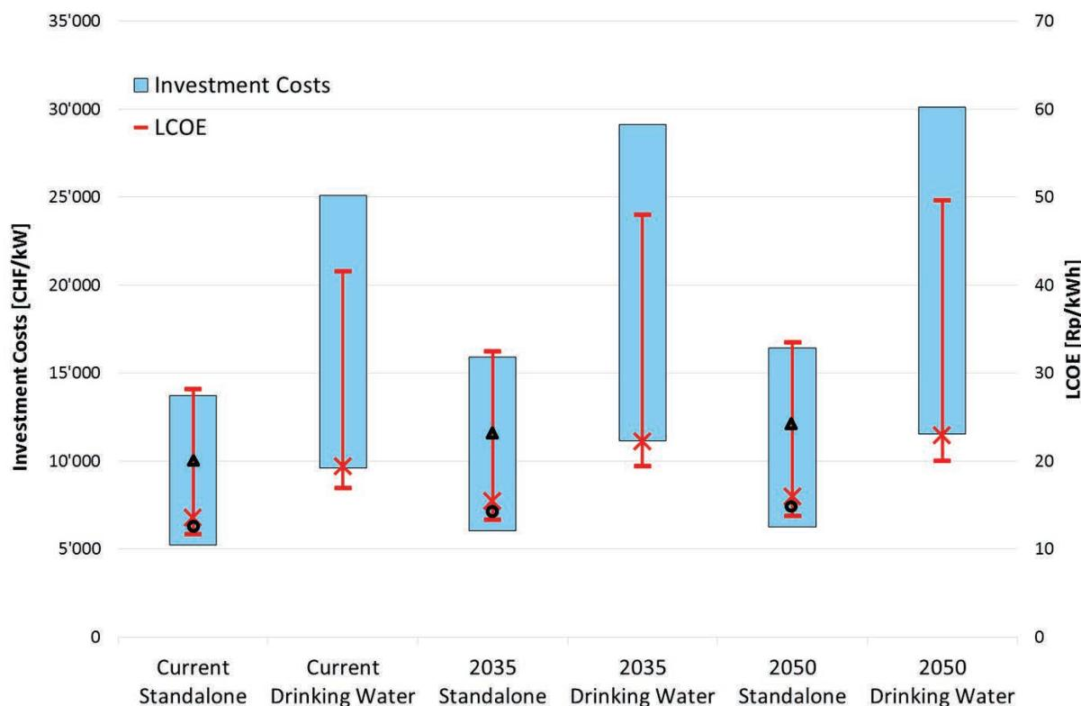
**Figure 7.12:** Range of overnight investment costs and leveled cost of electricity (LCOE) of SHP in Switzerland for current and future new constructions. Average LCOE, calculated as weighted average with annual expected electricity production, is marked as red “X”. LCOE of standalone plants <1MW are marked as black triangles; those of plants 1-10 MW are marked as black circles.
