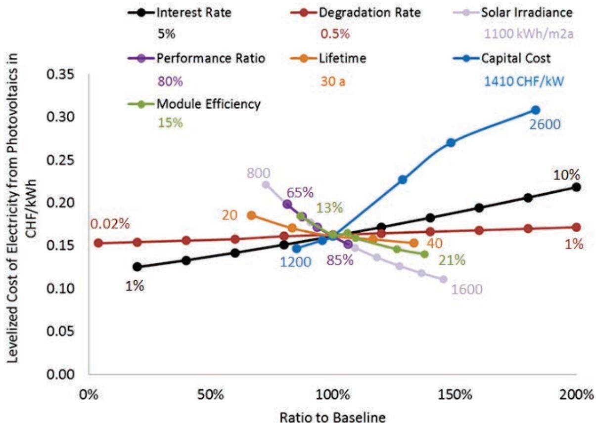
**Figure 9.33: Sensitivity analysis of current LCOE, center point represents current LCOE of a 100 kWp system.**
