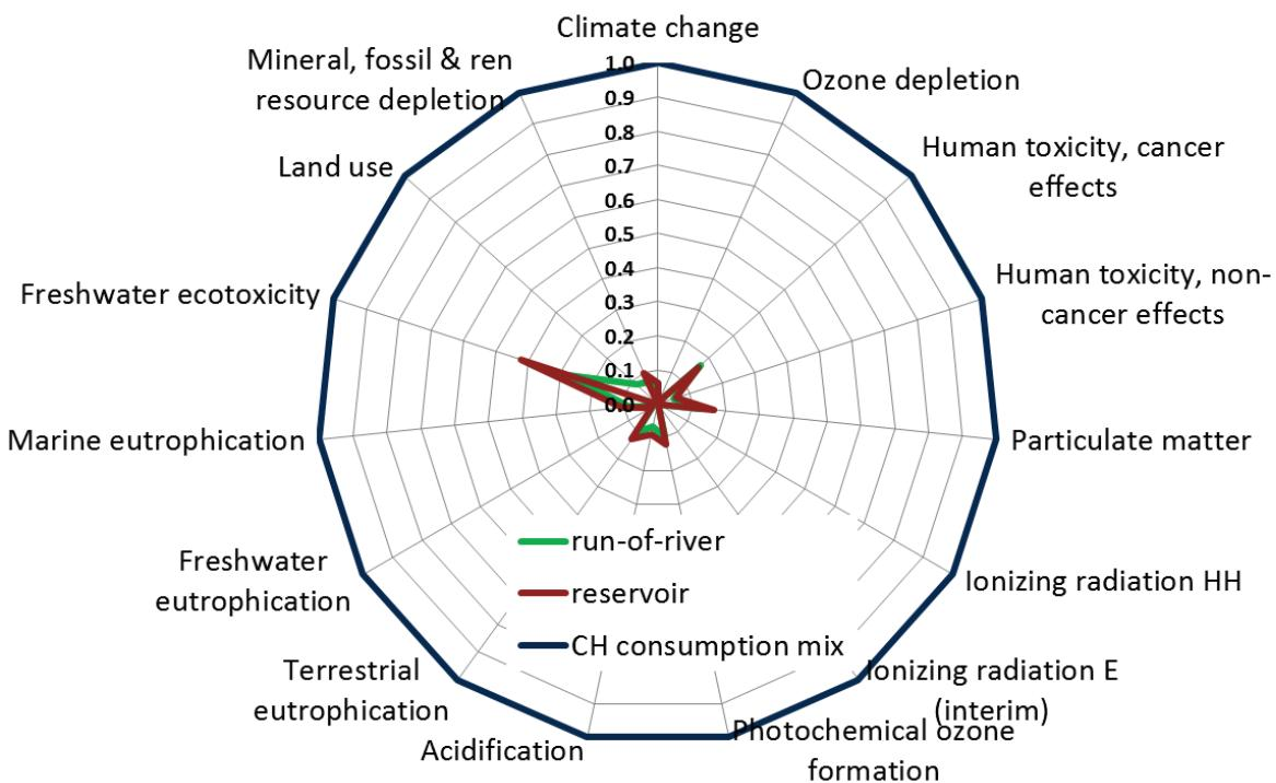
**Figure 6.21: Comparison of LCIA indicators for the average Swiss consumption mix, Swiss storage and run-of-river power plants, relative to the Swiss consumption mix (=1).**
