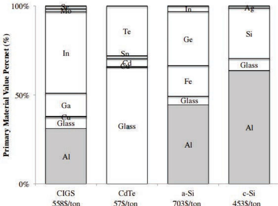
**Figure 9.21: Material value breakdown in crystalline silicon and thin-film modules (Goe 2014)**
