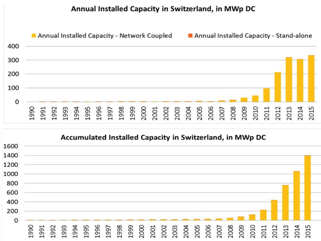
Figure 9.6: The PV Installations in Switzerland from 1990 to 2015: Annual Capacity Installed and Accumulated Capacity Installed (BFE/SFOE 2016f).
