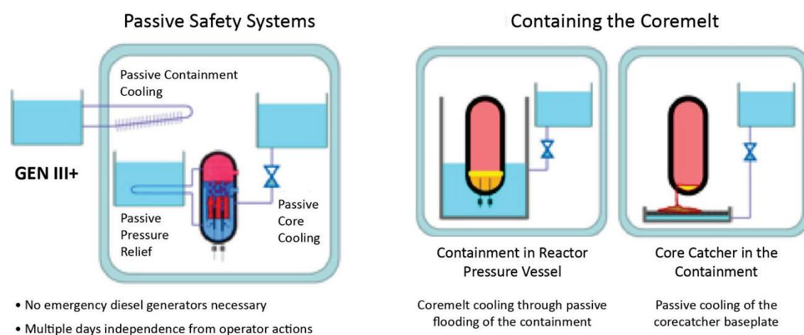
**Figure 14.2: Examples of passive safety systems and features for core melt retention in the containment of light water reactors (Hirschberg, Eckle et al. 2012)(Hirschberg, Eckle et al. 2012).**
