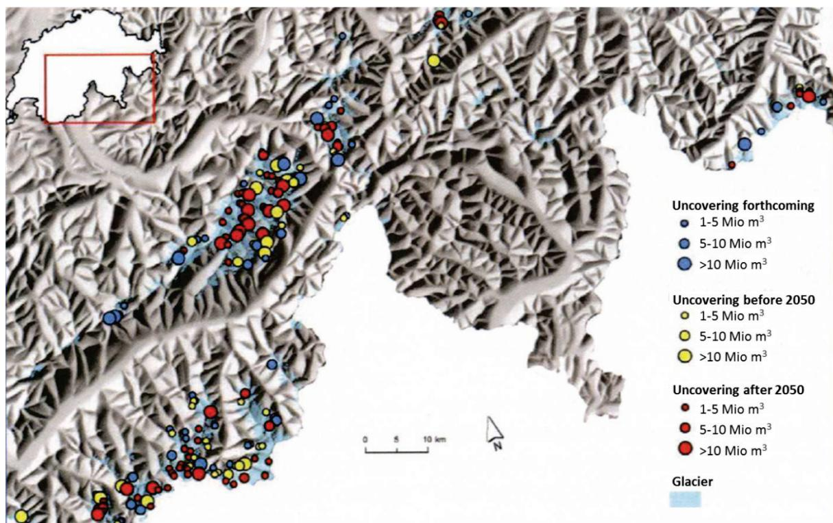
**Figure 6.15: Potential locations and sizes of new lakes in currently glaciated areas due to global warming (Haeberli, Schleiss et al. 2012).**
