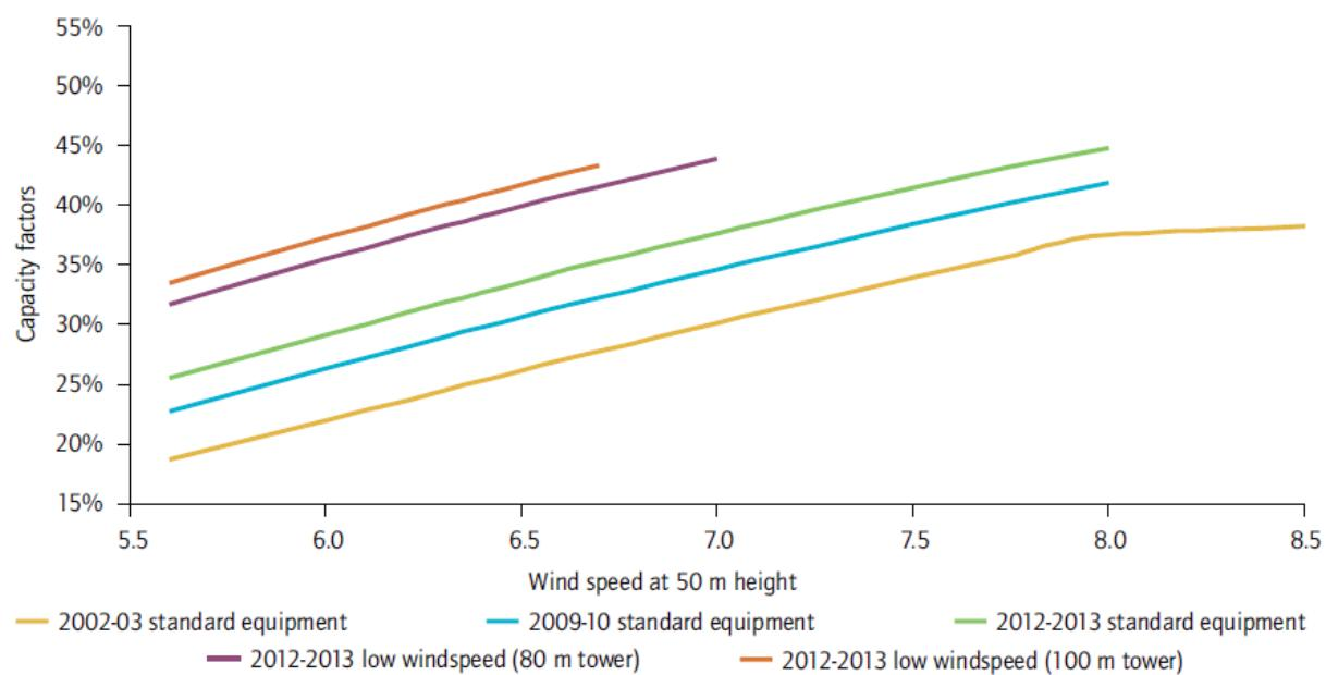
**Figure 8.16: Evolution of the wind capacity factor in the last 15 years (IEA 2013a).**
