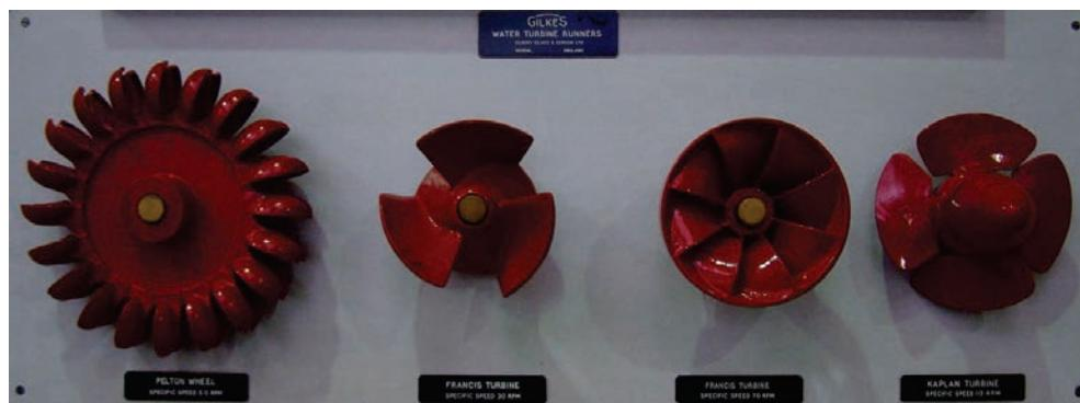
Figure 6.5: Various types of water turbine runners. From left to right: Pelton Wheel; Francis Turbine; Francis Turbine; Kaplan Turbine.<sup>129</sup>
