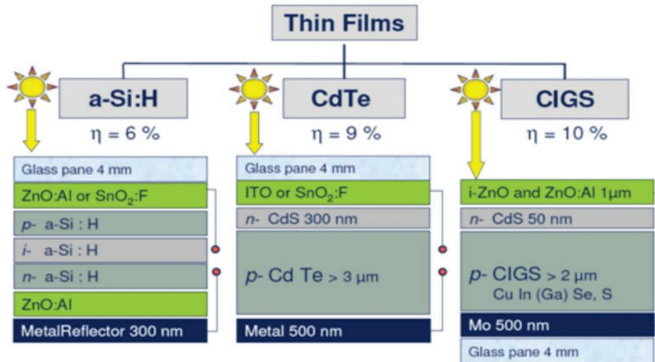
Figure 9.13: Types of thin-film solar cells and their structure (Jung 2008).
