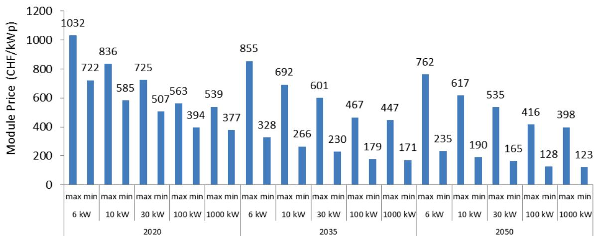
**Figure 9.34: Future estimated maximum and minimum module cost for various installation sizes in Switzerland, 2020-2050.**
