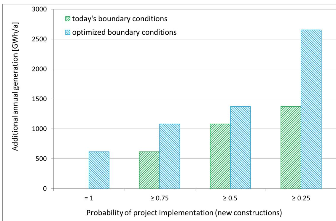
**Figure 6.12: Alternative estimation of additional electricity generation with new hydropower plant constructions, relating to an expected annual generation of 35.8 TWh/a as of 1<sup>st</sup> of January 2012 according to project specific data in Annex 2 of (BFE/SFOE 2012b).**
