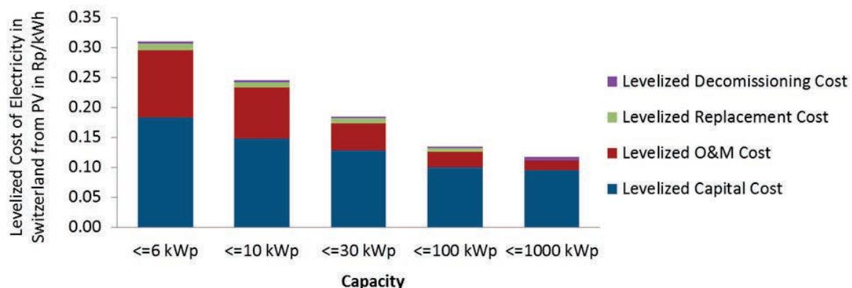
Figure 9.32: Current LCOE for Swiss PV systems at various sizes, under average performance (generation, efficiency).
