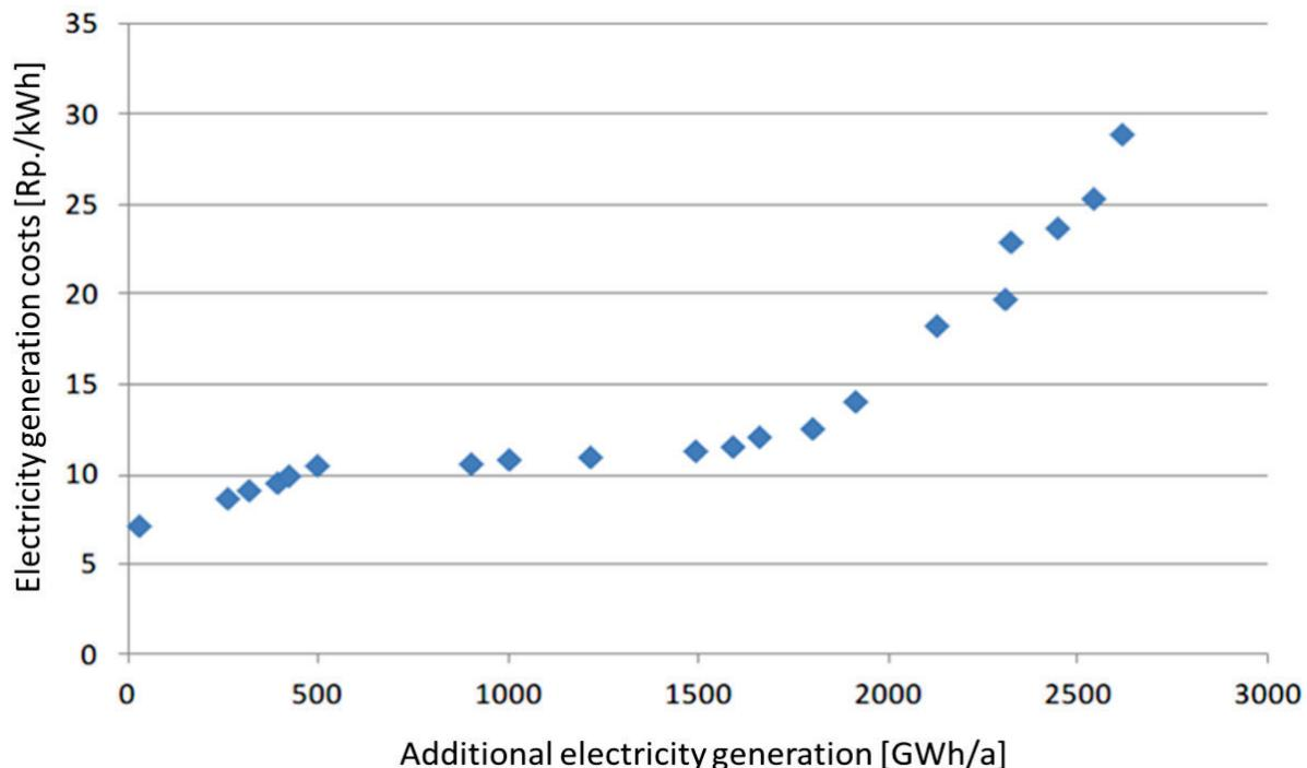
**Figure 6.19: Cumulative additional large hydropower electricity production ranked according to increasing generation costs (BFE/SFOE 2013c).**
