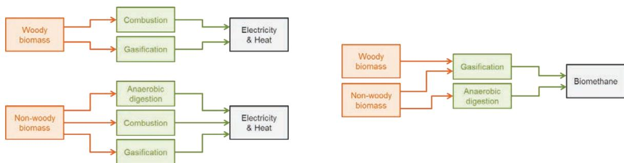
**Figure 10.1: Broad overview of conversion pathways from biomass resources to electricity.**
