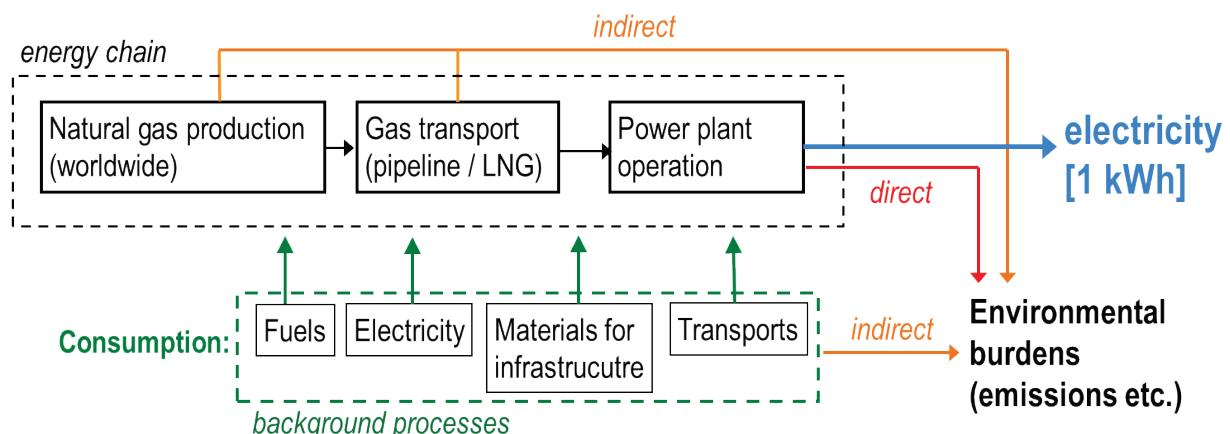
**Figure 5.11: Schematic representation of the LCA process model for electricity generation with a natural gas power plant; [1 kWh] indicates the functional unit of the LCA.**
