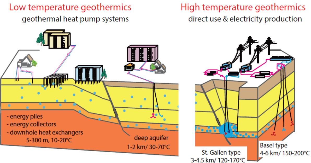
Figure 11.1: Different types of systems using geothermal energy. Taken from (Hirschberg, Wiemer et al. 2015).
