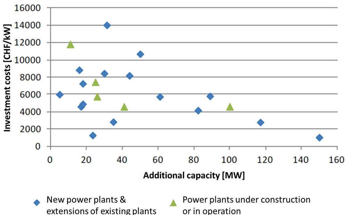
Figure 6.18: Specific investments costs of new large hydropower plants, as analyzed in (BFE/SFOE 2013c).
