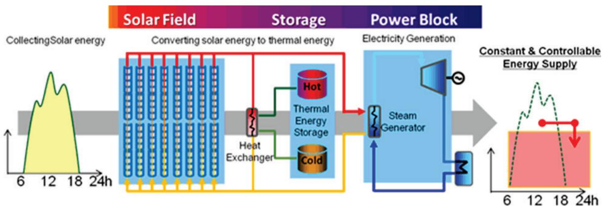
Figure 13.4: Schematic of a CSP system consisting of solar field, storage system and power block (Chiyoda 2016).
