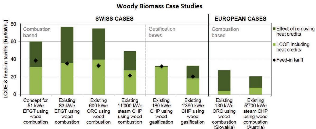
**Figure 10.40: Comparison of the wood sector case studies from Section 10.5.3 with an estimate of the feed-in tariffs that they would receive. Feed-in tariffs in Switzerland are estimated using the online feed-in tariff calculator<sup>229</sup>. Cost structure information is shown in Figure 10.34 and detailed in the appendix of this chapter.**
