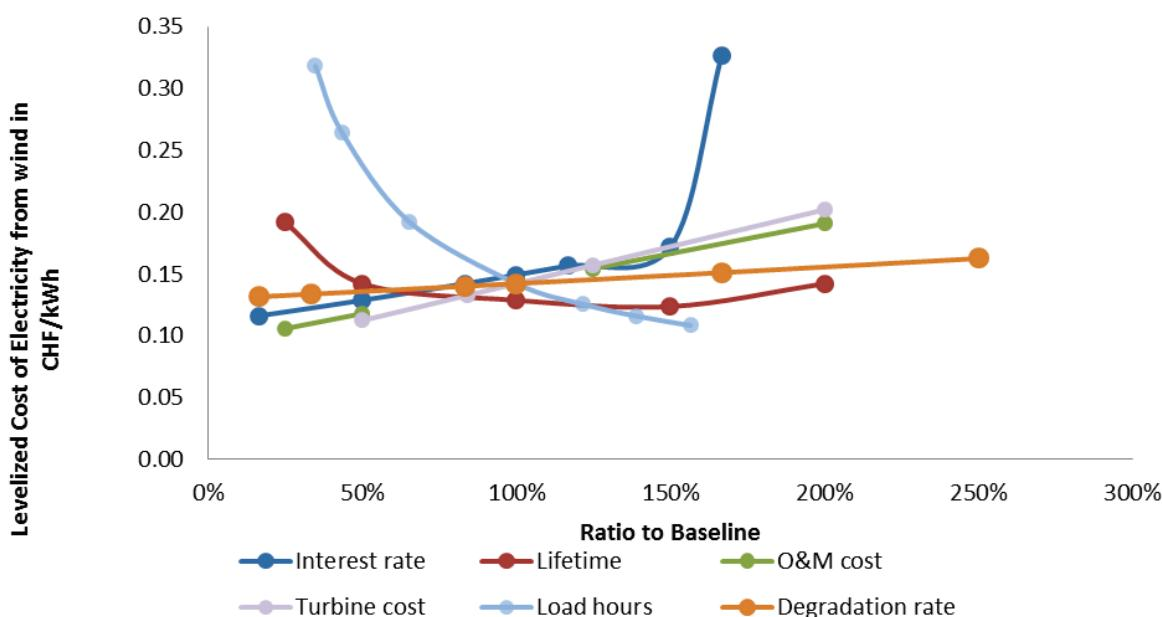
**Figure 8.24: Sensitivity analyses of key cost factors in LCOE of wind power. Results for decommissioning costs are not shown in the graph (see explanation in the text).**
