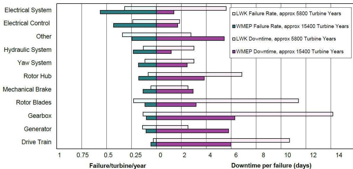
Figure 8.18: Failure types and related downtime of wind turbines. Taken from (Sheng 2013). Data are taken from two European databases with a sample of 5800 and 15400 turbine years, respectively, over 13 years of operation. The databases closed in 2006, so that the data are at least 10 years old.
