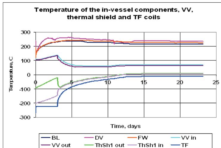
**Figure 17.13: Temperature evolution in ITER in case of loss of coolant after a shut down.**<sup>388</sup>
