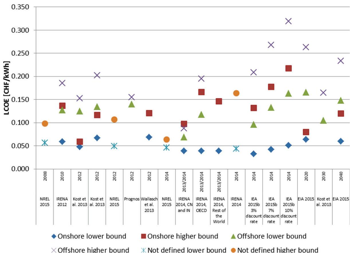
**Figure 8.20: Literature review on LCOE of wind power. Costs are converted to and given in CHF/kWh. 1USD=0.976CHF; 1EUR=1.092CHF. The x-axis shows the source and the year for which the values are given. Not all references differentiate between on- and offshore turbines, so that the corresponding values are provided under the category “not defined”, i.e. it is unknown whether they represent on- or offshore conditions.**
