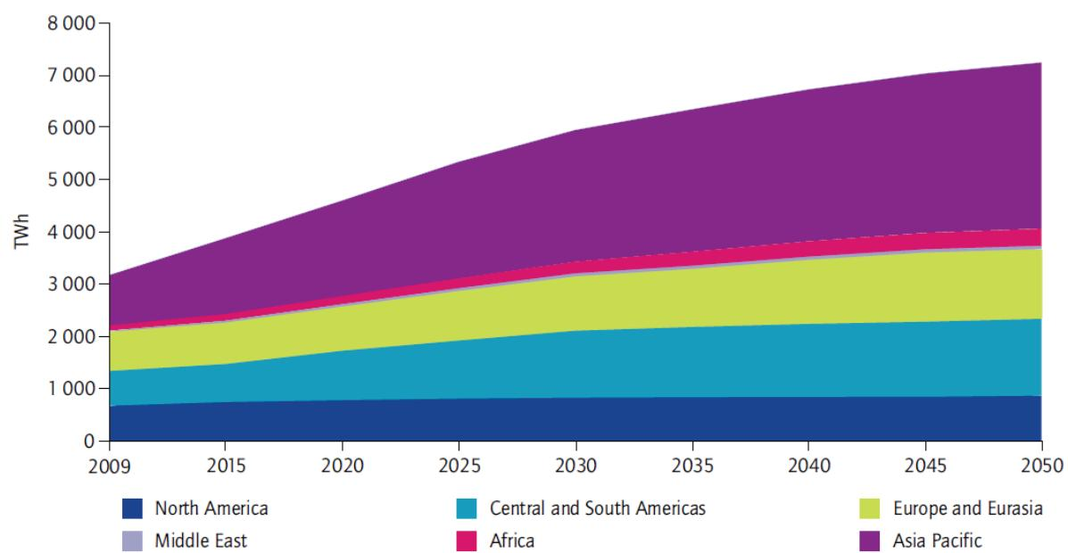
Figure 6.9: Hydroelectricity generation till 2050 in the Hydropower Roadmap vision (OECD/IEA 2012).
