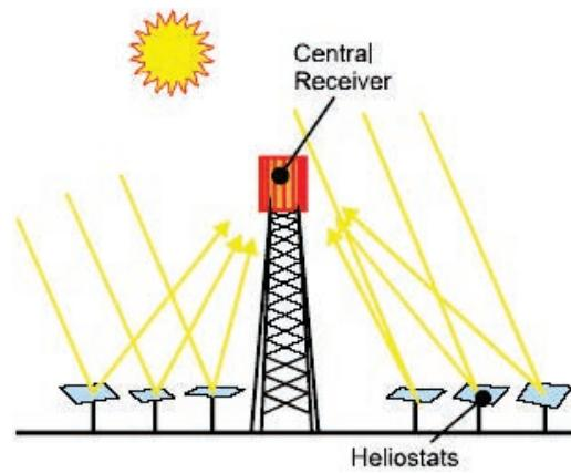
Figure 13.6: Schematic of central receiver or solar tower system (SolarPACES 2016a).
