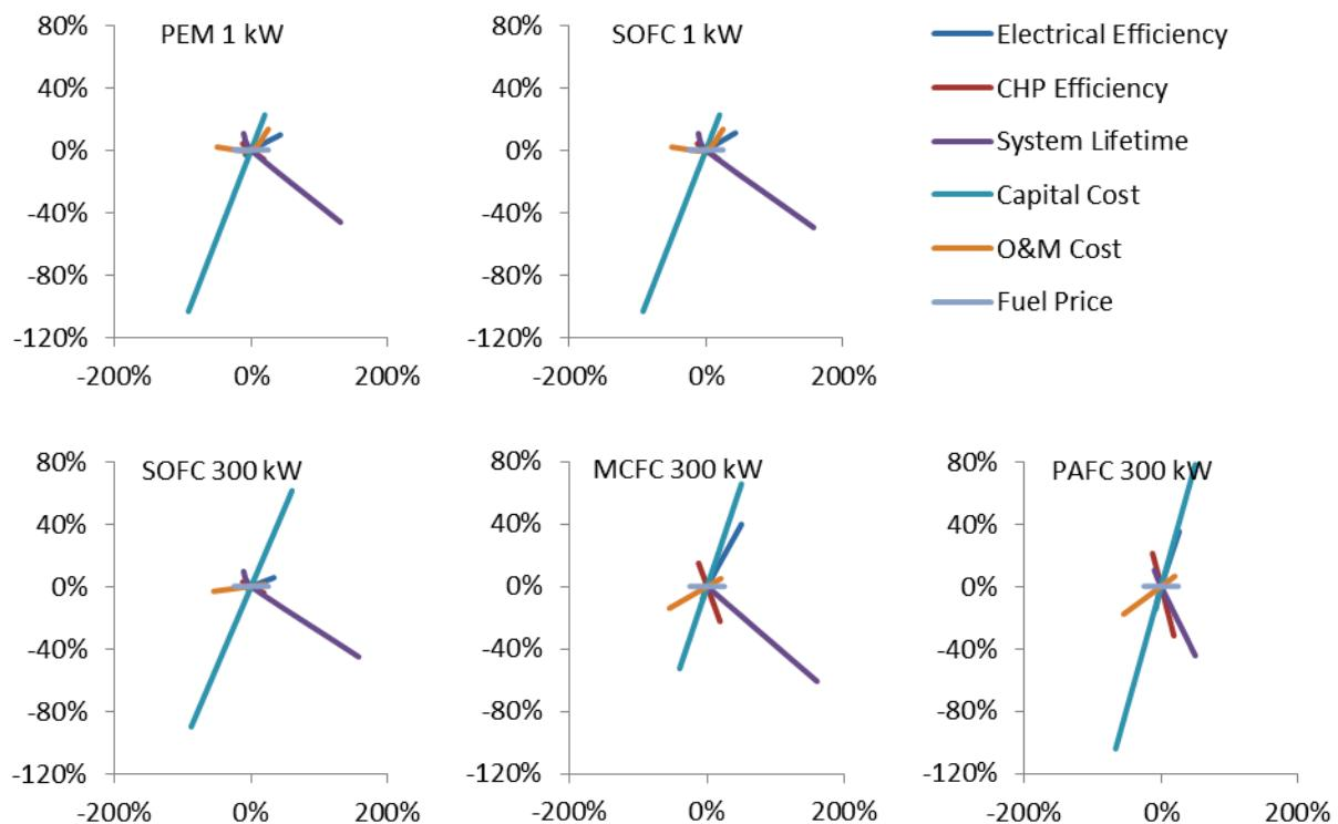
**Figure 16.6: Cost sensitivity analysis results. The x axis shows the variation in input parameters, while the y axis shows the variation in results.**
