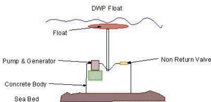
**Figure 12.10: Schematic Diagram of Seabed Piston Pump Design.**<sup>306</sup>
