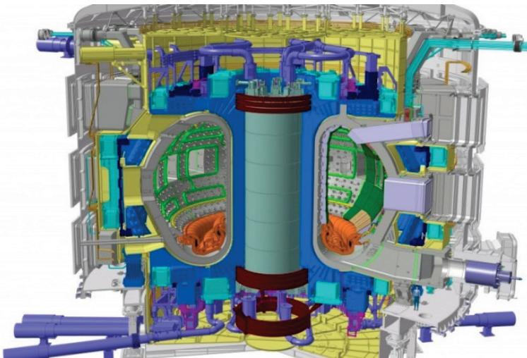
**Figure 17.8:** Schematic of a tokamak , ITER. The scale of a man is shown on the right. The plasma is a D shaped doughnut filling the central volume.<sup>384</sup>
