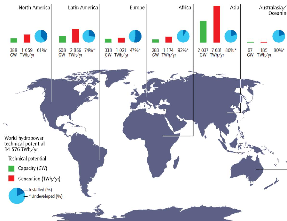
Figure 6.8: Regional technical hydropower potential and percentage of undeveloped technical potential (2009) (OECD/IEA 2012).
