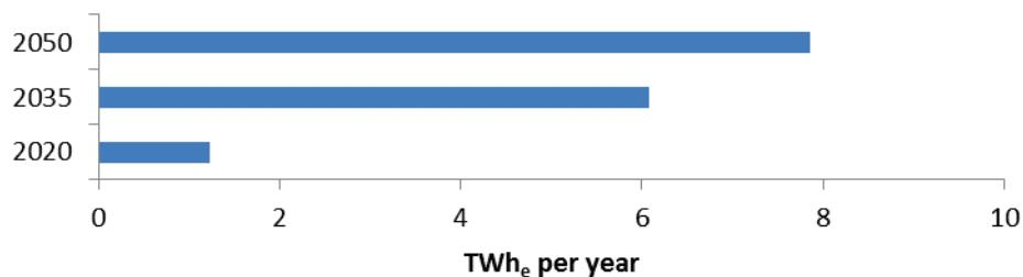
**Figure 16.3: Economically realizable electricity generation potential from small combined heat and power plants.**
