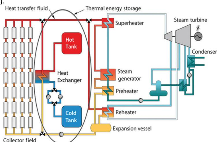
**Figure 13.10: Parabolic trough plant with two tank indirect heat storage (Siegel 2012).**
