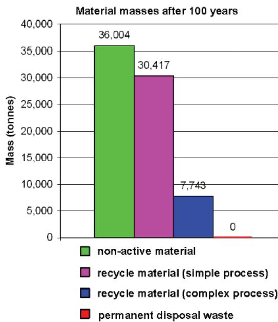
**Figure 17.15: Classification of the waste of a fusion reactor after 100 years of intermediate storage. Please note the zero amount of waste, which requires permanent disposal (EFDA 2005).**
