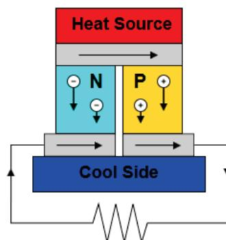
**Figure 17.17: Scheme of a thermoelectric circuit composed of materials of different Seebeck coefficient (p-doped and n-doped semiconductors), configured as a thermoelectric generator.<sup>391</sup>**
