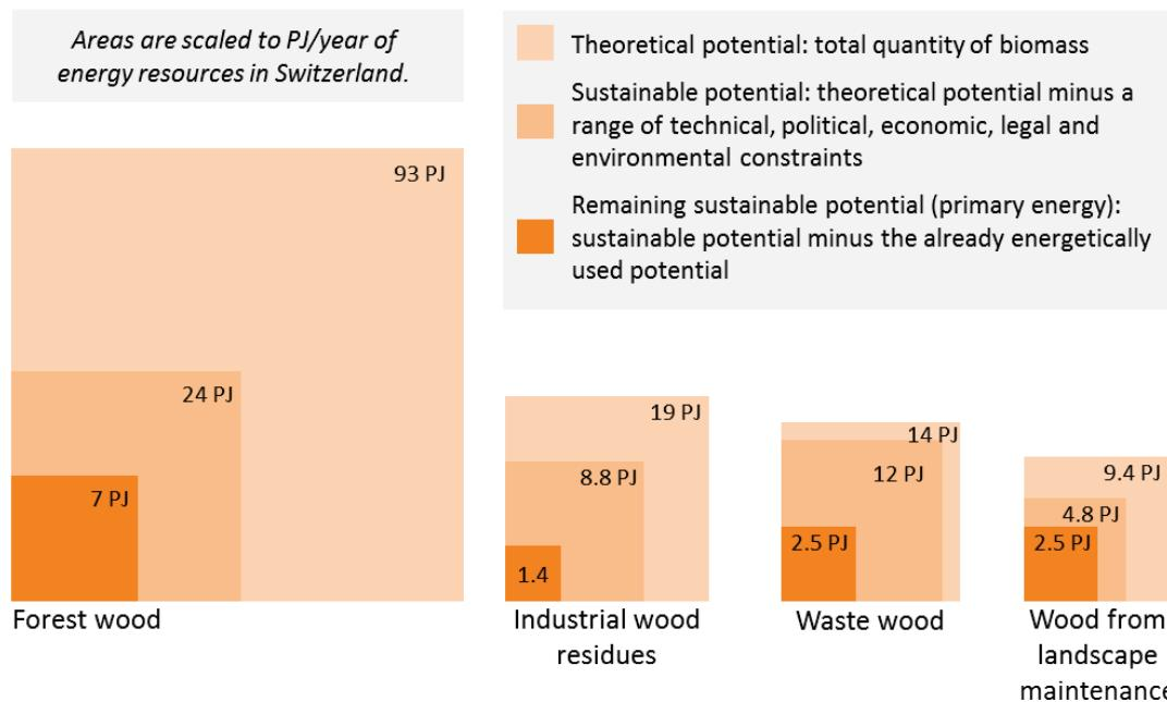
**Figure 10.16: Potentials of domestic woody biomass resources in Switzerland, from (Erni, Thees et al. in preparation, status: 16.11.2016)<sup>211</sup>.**
