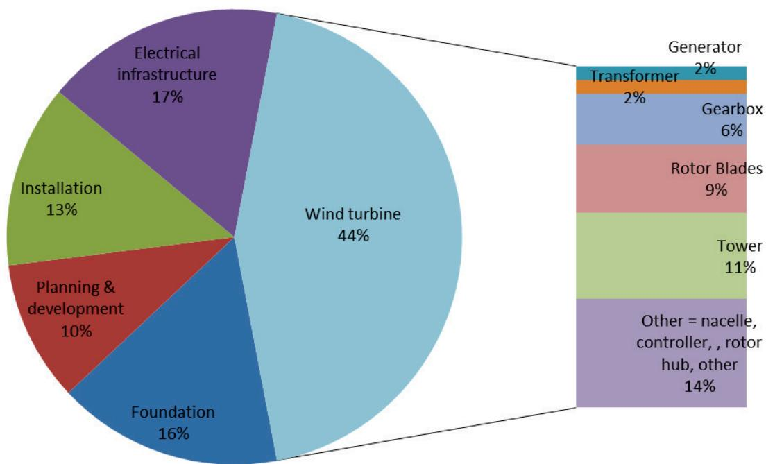
**Figure 8.22: Capital cost breakdown for a typical offshore wind power system and turbine (IRENA 2012c).**
