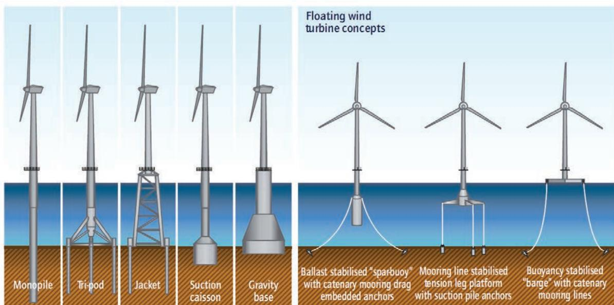
**Figure 8.15: Types of fixed-bottom and floating offshore support structures. Taken from (IEA 2013a).**
