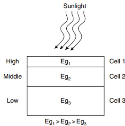
**Figure 9.14: Operation of a three-layer multi-junction PV (Lamont 2013).**
