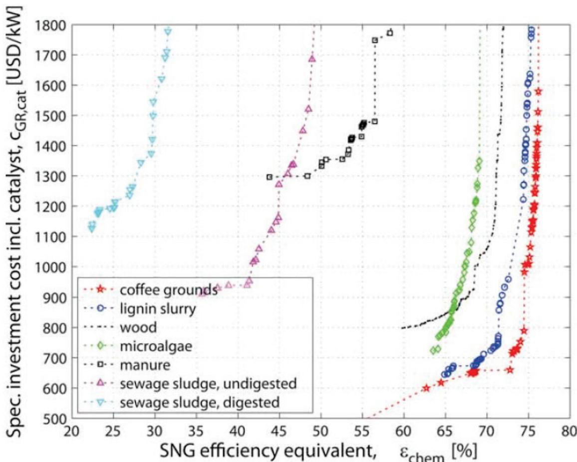
**Figure 17.4: Specific investment cost and overall process efficiency without power recovery from the high pressure vapor phase for PSI’s catalytic hydrothermal methanation process.** Reproduced from (Gassner, Vogel et al. 2011) with permission.
