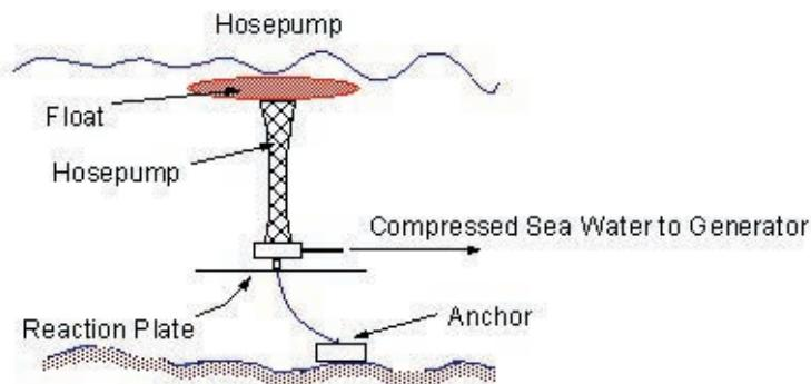
**Figure 12.11: Schematic Diagram of Hosepump Pump Design.**<sup>307</sup>
