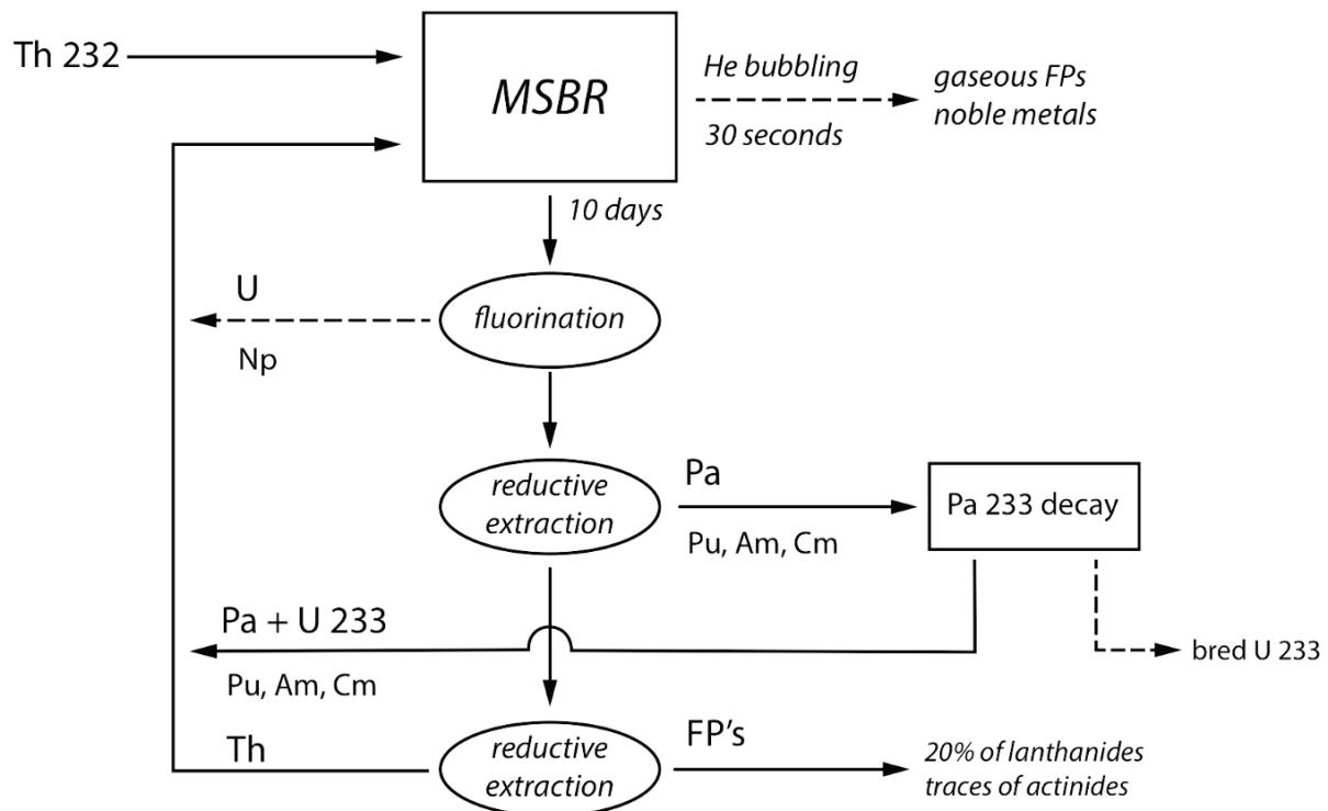
**Figure 14.4: Simplified diagram of the continuous reprocessing of the MSBR concept of ORNL.**
