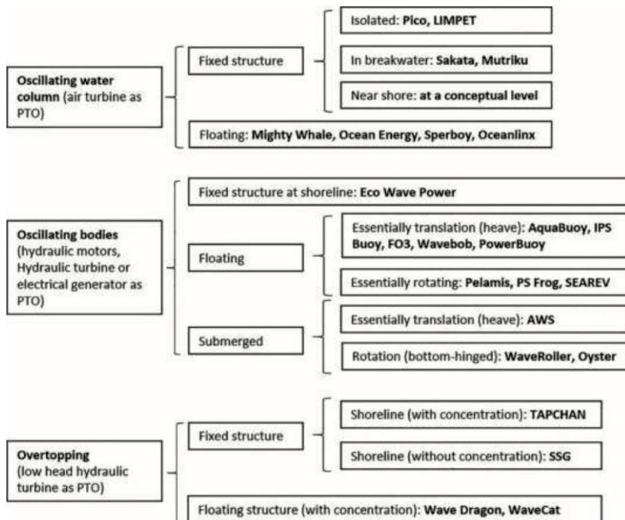
Figure 12.2: Classification of wave power devices by type of power absorber.
