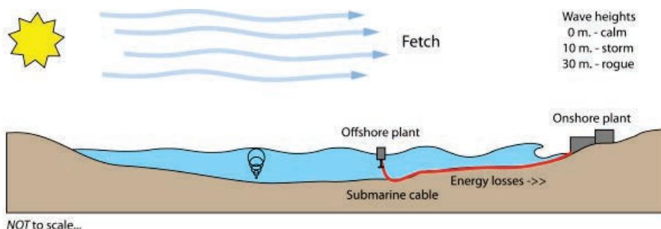
**Figure 12.1: Schematic diagram of wave power fundamentals (Source: PSI).**
