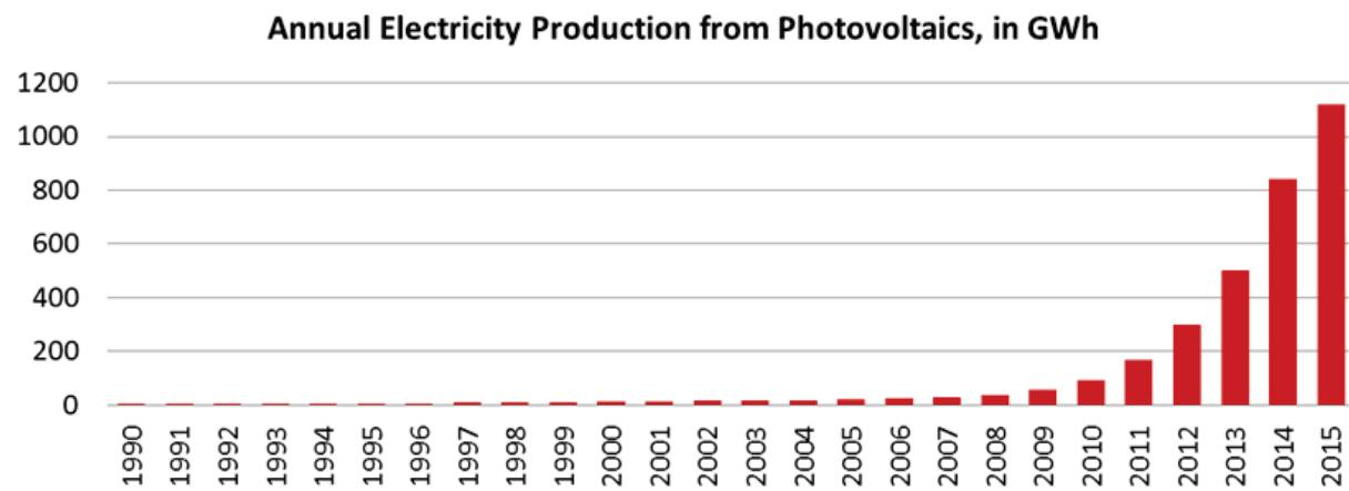
Figure 9.7: Annual generation of electricity from PV in Switzerland 1990-2015 (BFE/SFOE 2016f).
