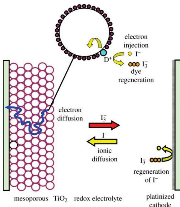
**Figure 9.15: Working principal of dye-sensitized solar cells (Peter 2011).**
