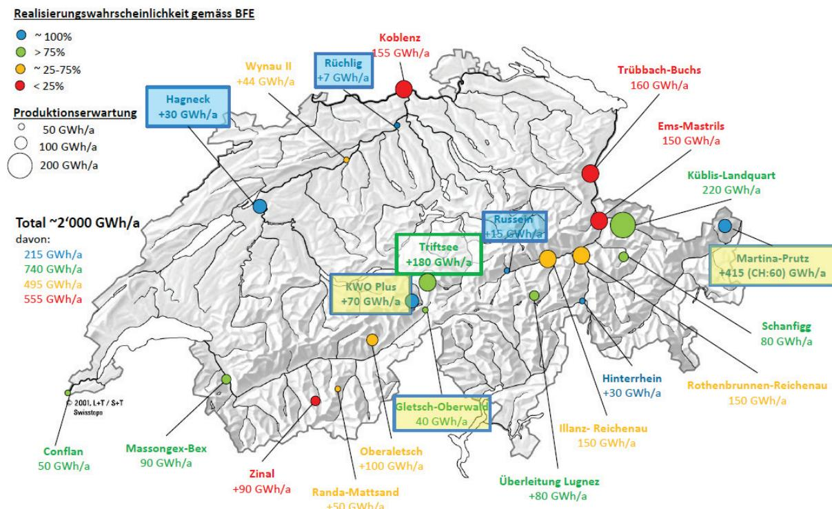
Figure 6.13: Locations and expected (increase in) annual production of specific potential future hydropower projects (Boes 2016).
