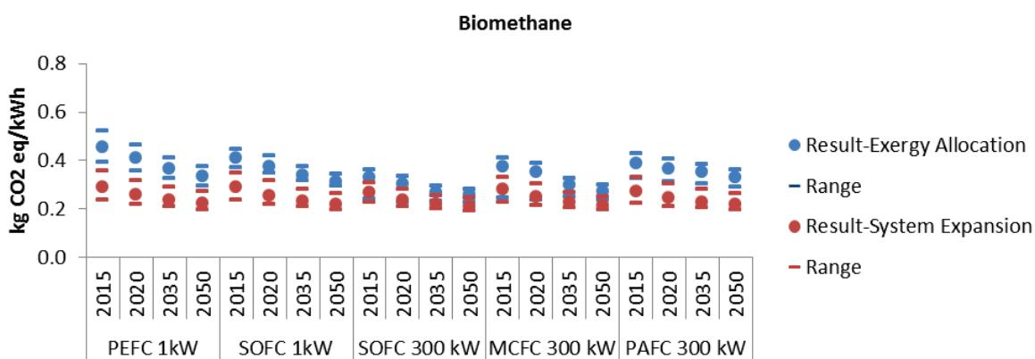
**Figure 16.10: Lifecycle GHG emissions for current and future fuel cells powered by biomethane from sewage gas. Burdens for heat and electricity production are allocated by exergy allocation and system expansion, though quantified per kilowatt-hour of electricity produced.**
