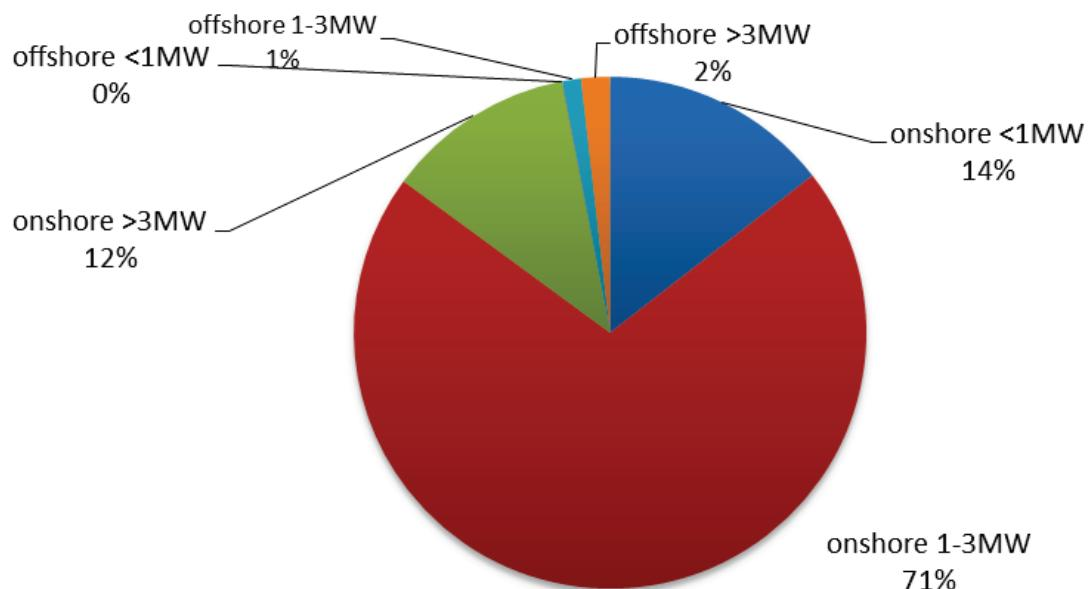
**Figure 8.12: Installed capacity of wind power worldwide in turbine size classes, separated into onshore and offshore installations. Based on (Pierrot 2015) with data for the end of 2014.**
