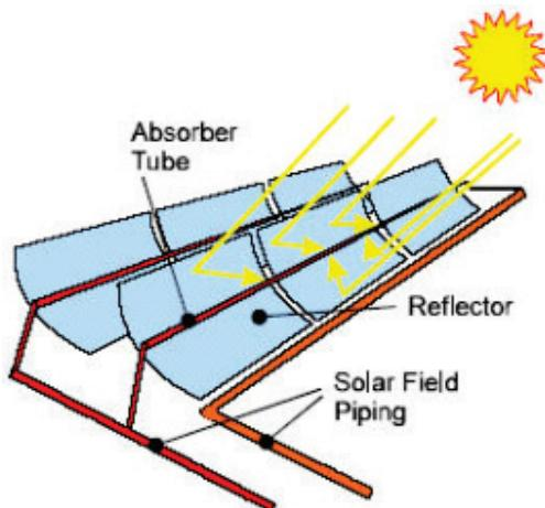
Figure 13.5: Schematic of parabolic trough concentrator (SolarPACES 2016a).
