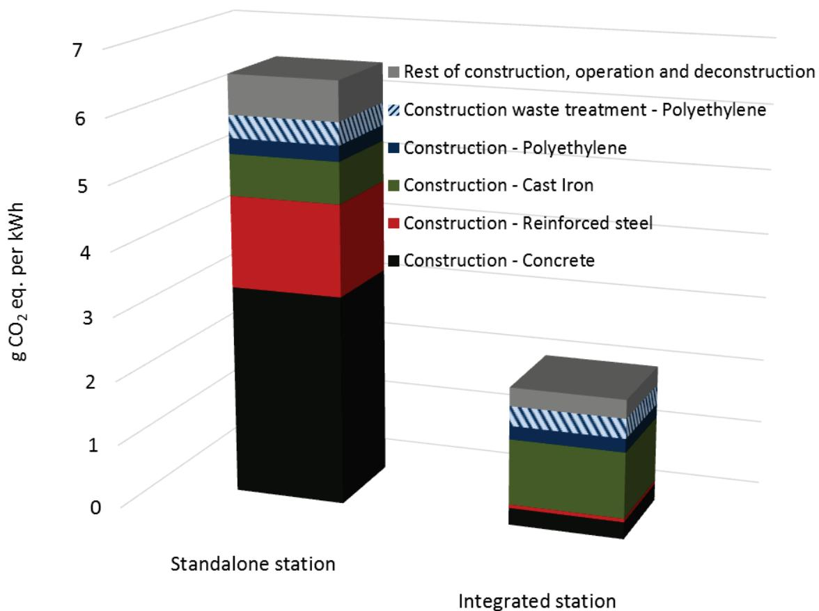
**Figure 7.13: CO<sub>2</sub> equivalent assigned to the process of providing 1 kWh high voltage with small hydropower in Switzerland. Impact assessment method: IPCC GWP 100a.**
