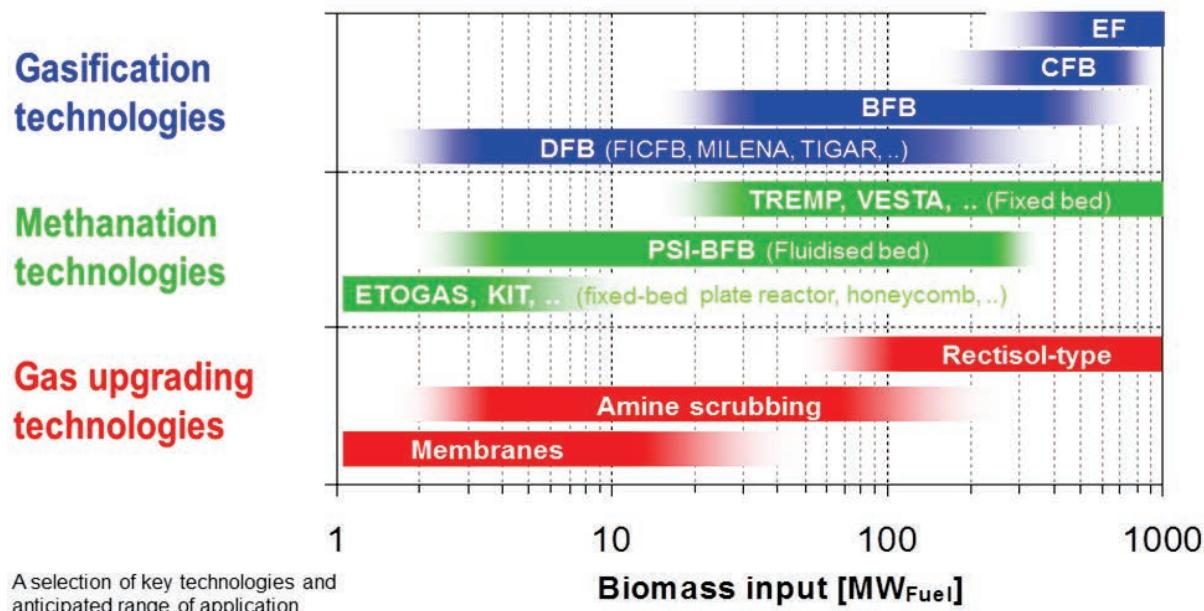
**Figure 10.3: A selection of key technologies for biomethane production from woody biomass (Biollaz, Schildhauer et al. 2015).**
