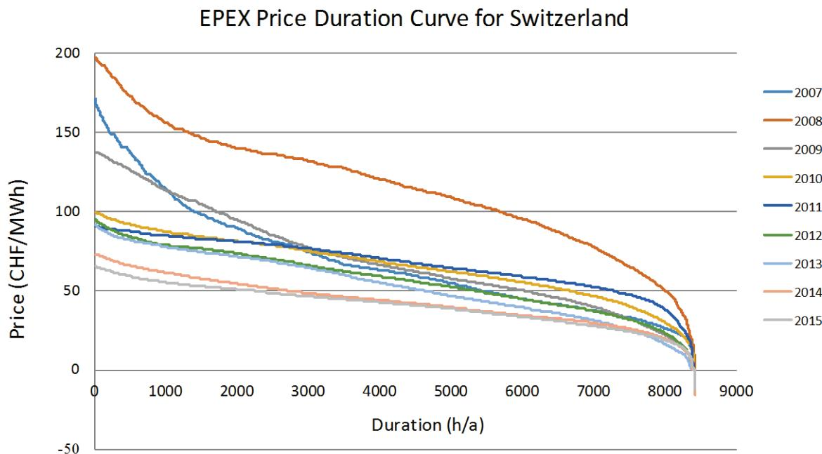
**Figure 14.12: European Power Exchange (EPEX) energy spot prices for Switzerland.<sup>362</sup>**
