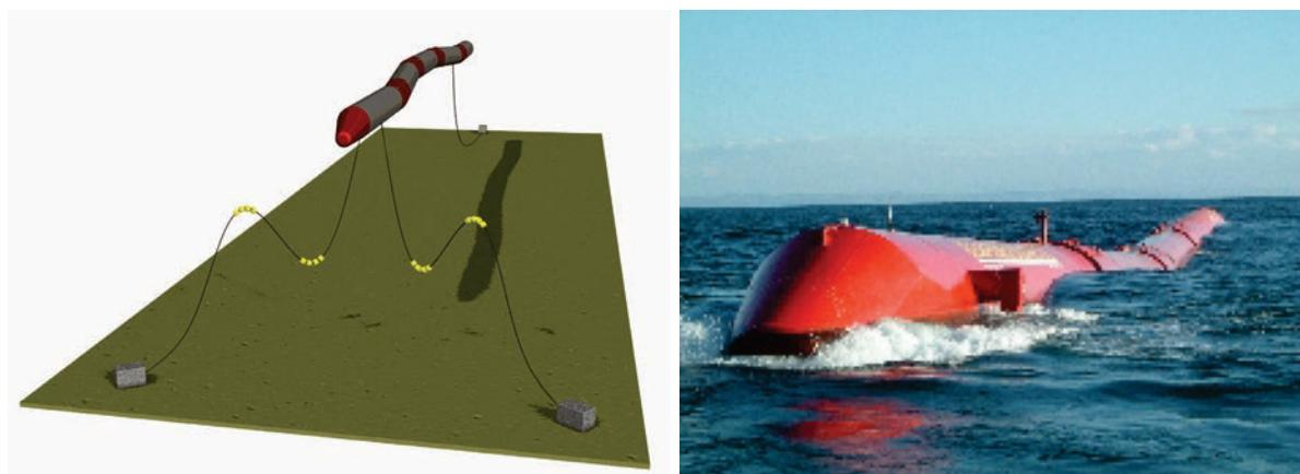
**Figure 12.8: Schematic Diagram of Pelamis Design<sup>303</sup> and photo of Full Size Pelamis Prototype.<sup>304</sup>**
