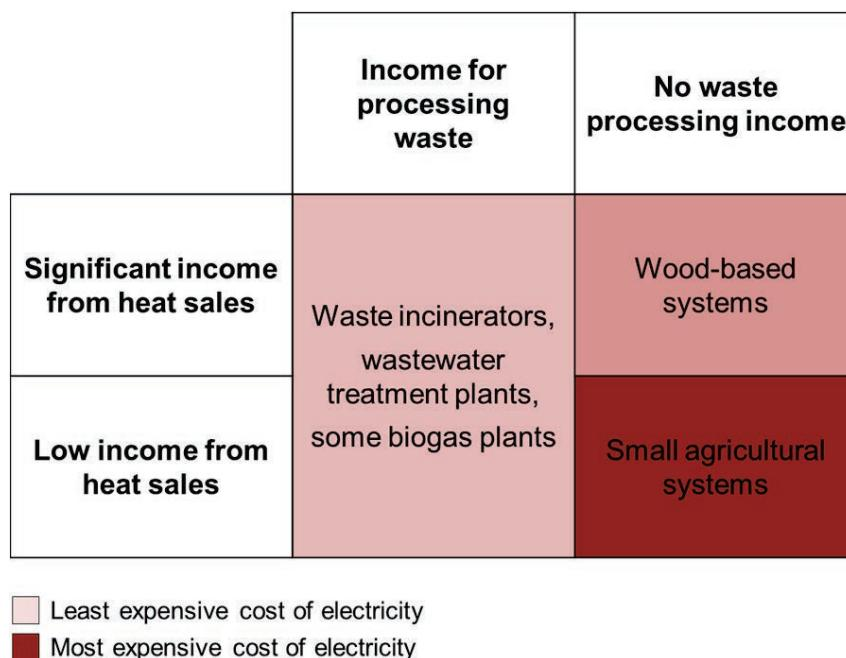
**Figure 10.32: Business models for electricity production from biomass. Darker red represents options that are generally more expensive than lighter red options.**
