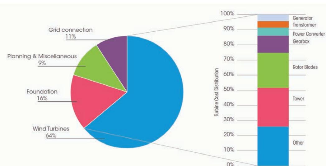
**Figure 8.21: Capital cost breakdown for a typical onshore wind power system and turbine. Taken from (IRENA 2012c).**
