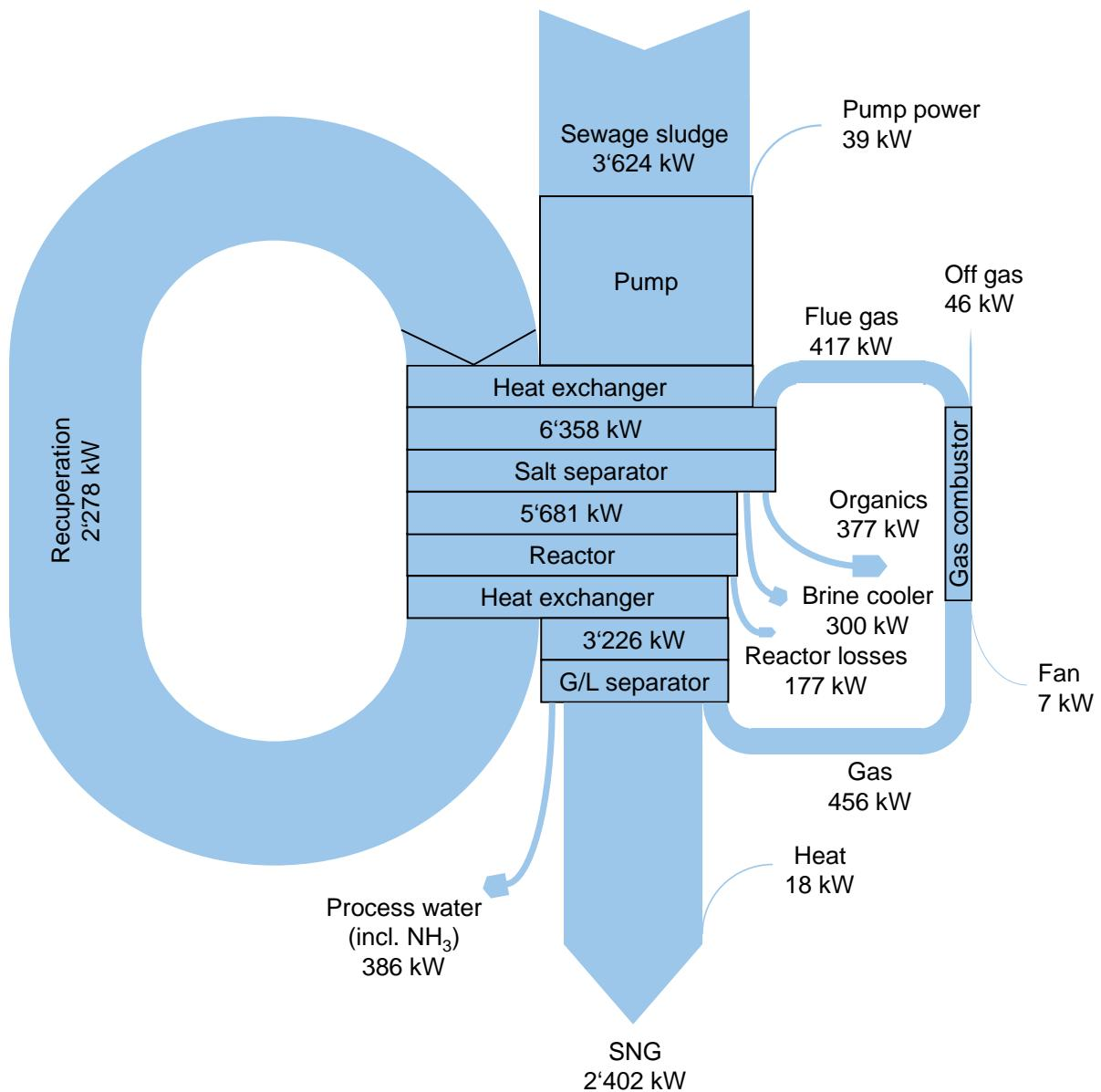
**Figure 17.2: Energy flow diagram of PSI's catalytic hydrothermal SNG process for sewage sludge as feedstock. All enthalpies were calculated at 0.1 MPa and 25°C (Vogel 2012).**
