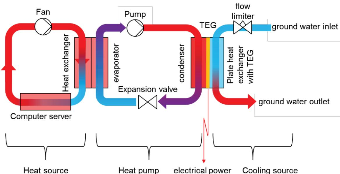
**Figure 17.18: Scheme of a simplified cooling cycle for a heat source, e.g. a server room, with thermoelectric generators (Battaglia, Widmer et al. 2016).**
