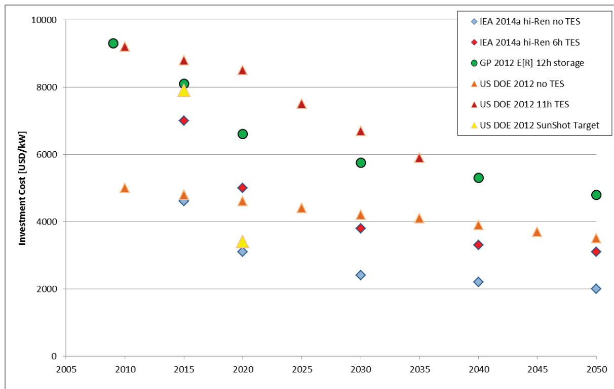
**Figure 13.16: Forecast for CSP plant investment costs according to different studies, scenarios and technologies ((IEA 2014b); (Teske 2012); (USDOE 2012)).**
