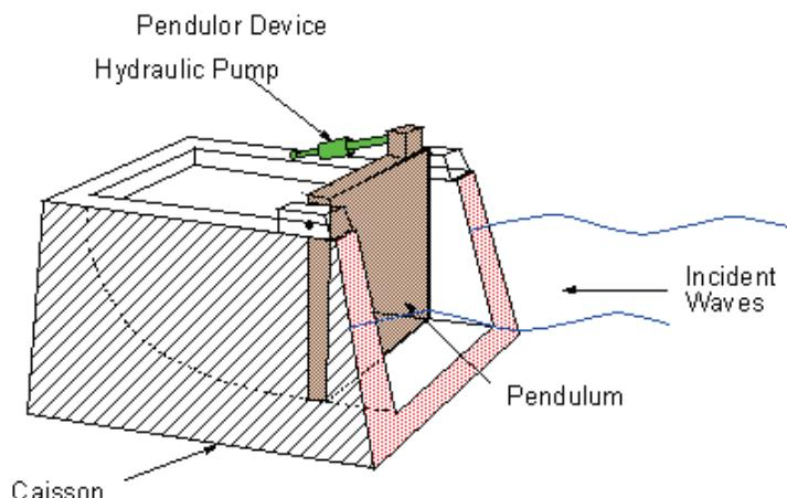
**Figure 12.5: Schematic Drawing of Pendulor Design.**<sup>300</sup>
