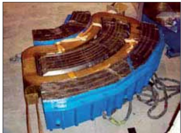
Figure 1: 90° bending magnet (delivered by Sigmaphi).
