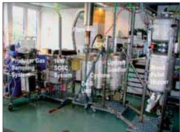
Figure 1: B-IGFC system scale test setup at PSI.
