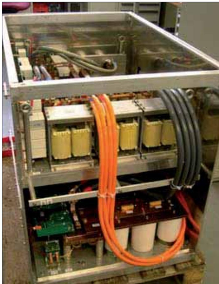
Figure 3: **The heart of the 90°-dipole PS with the filters (upper level) and the 4-quadrant converter (lower level) packed into a radio frequency proof housing.**
