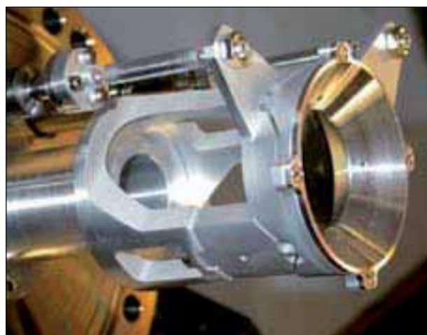
Figure 2: **The Gimbal mount can position optical devices with high precision.**
