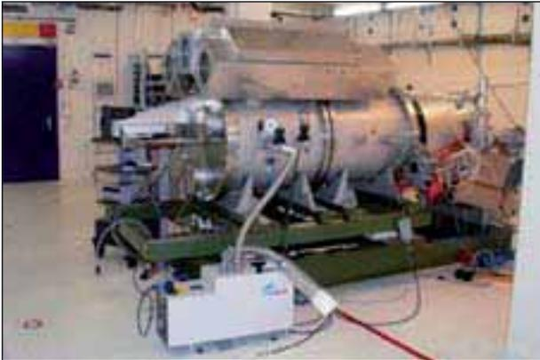
Figure 3: **500 kV High Gradient Pulser installed in the LEG test bunker.**
