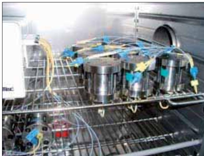
Figure 2: Diffusion pressure cells.
