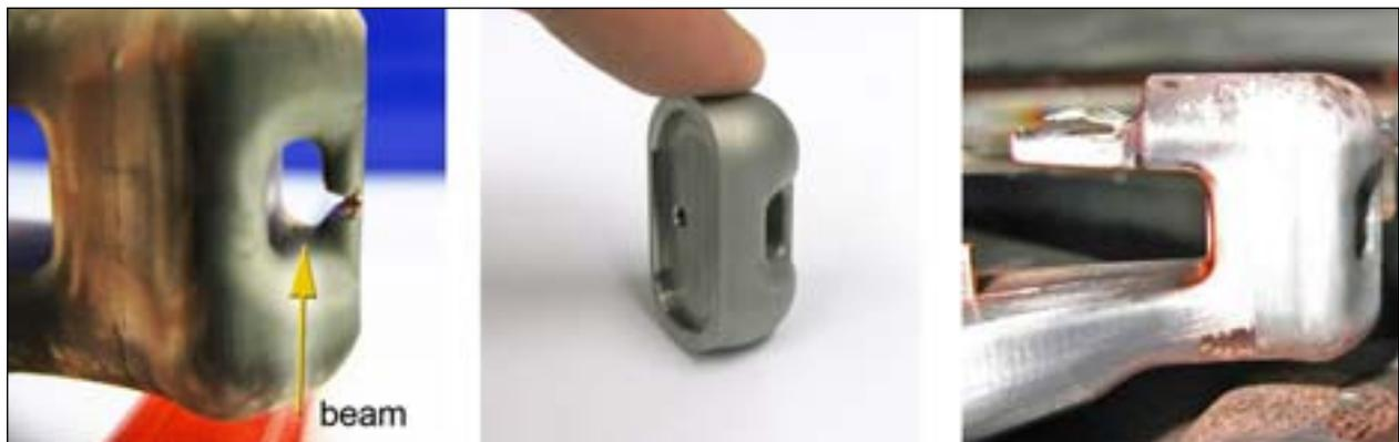
Figure 6: Damage of the puller nose due to loss of material by sputtering (left) has been decreased by applying a tungsten nose tip (middle) that does not show any degradation after 3 months of operation (right).
