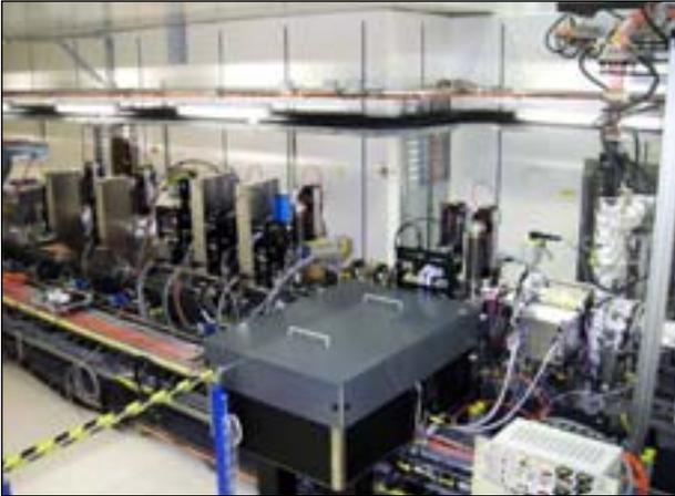
Figure 2: **Electron source and the first few metres of transport line in the injector tunnel.**
