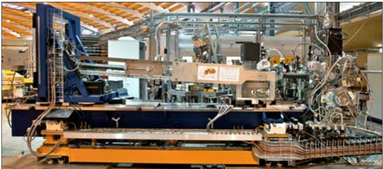
Figure 1: SAXES RIXS spectrometer at the ADRESS beamline.
