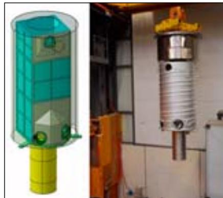
Figure 2: **Finished setup of the UCN storage volume surrounded by the heat radiation shield, vertical UCN guide on the bottom and ~10 tons steel shielding on top (about 5m tall): a) design drawing, b) during transport to its final position in the UCN tank.**
