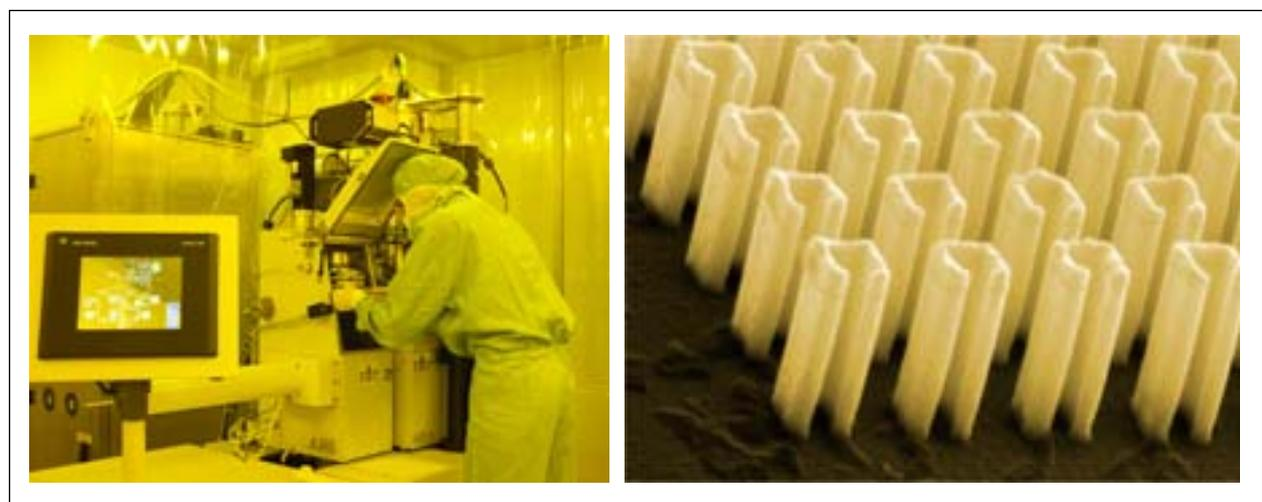
Figure 1: New ultra-high-resolution electron-beam lithography system (left). The system is used for writing complex nano structures, e.g. split-ring resonators consisting of narrow but tall gold shapes, which exhibit extraordinary optical properties (right). Line width: 60 nm, height: 1000 nm. Sample made by S. Gorelick.
