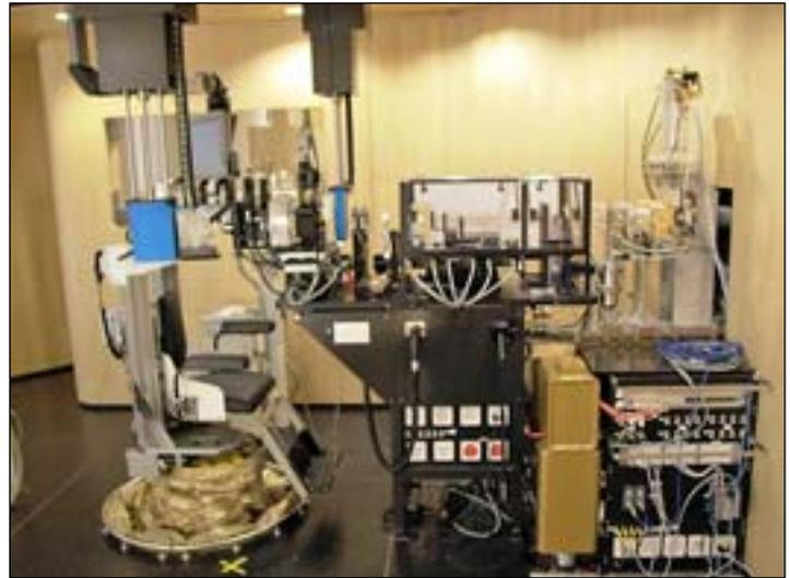
Figure 6: **The OPTIS2 nozzle. The seat is mounted on a parallel robot and the blue squares are integrated flat panels used to position the patients using X-rays.**
