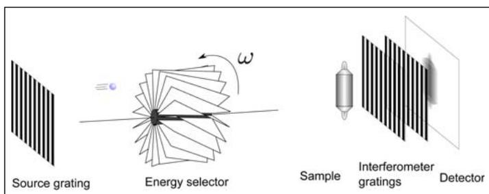
Figure 1: Schematic drawing of the interferometer setup.
