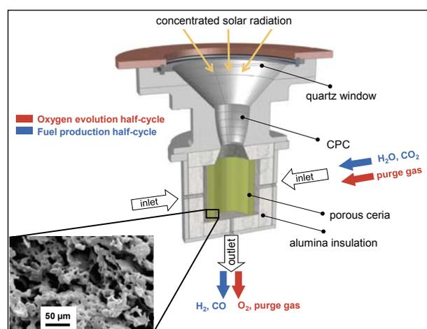
Figure 1: Schematic of the solar reactor for the two-step, solar-driven thermochemical production of fuels. Inset shows the scanning electron micrograph of the porous ceria tube after 23 cycles. The red arrow indicates ceria reduction (Eq. 1); the blue arrow indicates oxidation (Eq. 2a/2b).
