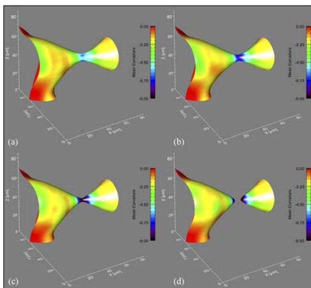
**Figure 1: A three-dimensional example of a liquid rod breaking up in an Al-15wt%Cu alloy. The interface is coloured by dimensionless mean curvature, with cooler colours (blue and black) indicating higher curvature. To reduce interfacial energy, the interface pinches off at the smallest diameter (the black-coloured interface), and the resulting cone-like shapes retract back into yellow-coloured regions of the interface.**
