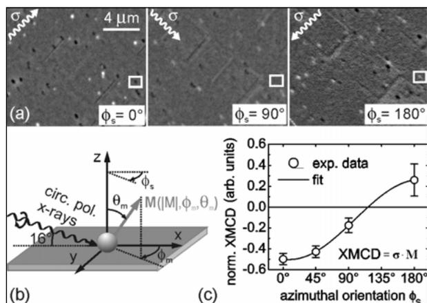
Figure 2: (a) Magnetic contrast images recorded at different azimuthal sample orientations  $\phi_s$ . (b) Experimental geometry. (c) Angle-dependent contrast of an individual particle marked by the square in (a) and the corresponding fit to the data.
