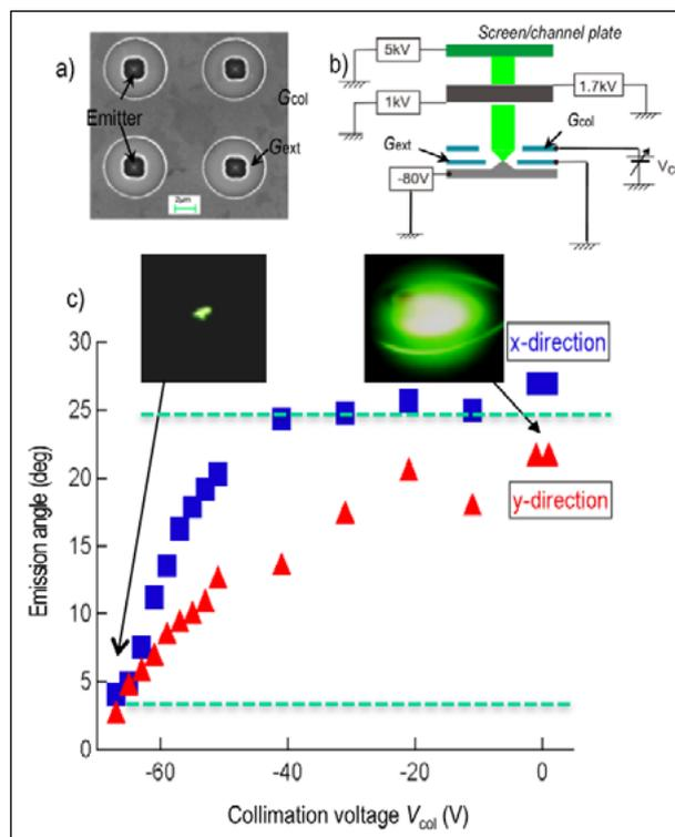
Figure 3: **(a) Scanning electron microscope image of double-gate FEA with 4 emitter tips (view from above). (b) Schematic diagram of field-emission microscopy experiment. (c) The relationship between the emission angle and the negative collimation gate bias  $V_{col}$ . Two electron beam images at  $V_{col}$ , equal to 0 V (right) and  $-67$  V (left), are also shown [10].**
