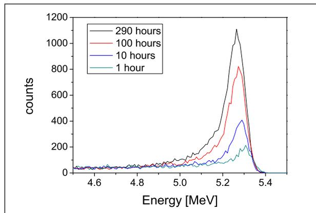
Figure 2:  $\alpha$ -spectra of the LBE grain after 1, 10, 100 and 290 h. Measurement time: 1 h each.
