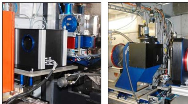
Figure 2: Pictures of the instrument boxes installed at ICON: source grating box (left) and interferometer grating box (right).
