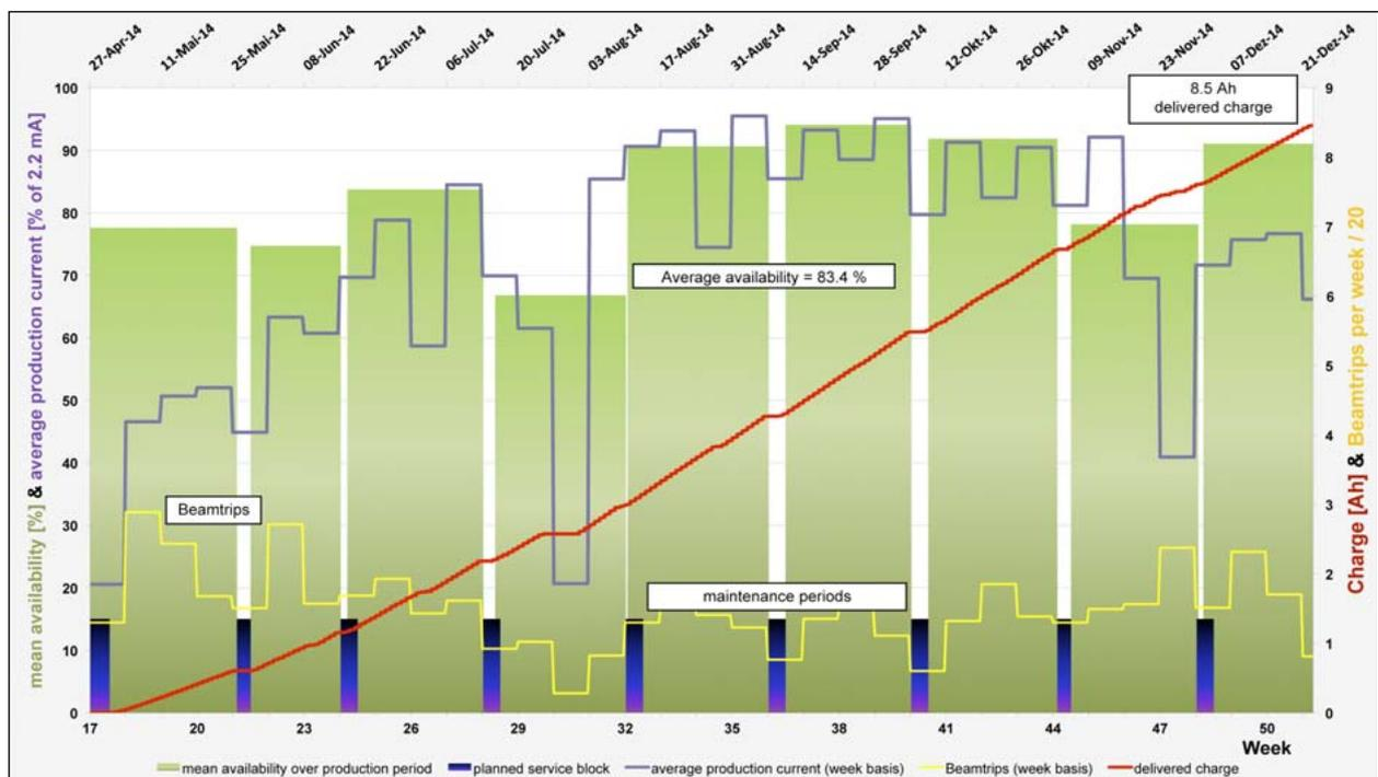
Figure 1: Operation of the Proton Facility: availability, average current, delivered charge and beam trips.
