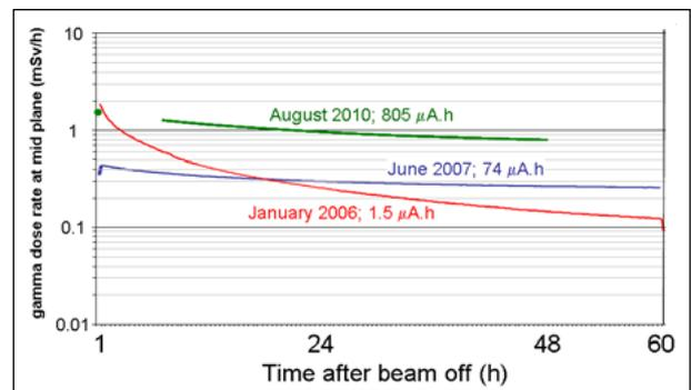
Figure 5: Measured dose rate in the mid-plane of the opened cyclotron. The 2006 measurement was performed immediately after delivering 500 nA for 1.5 hours, and thus shows a steep initial decay.
