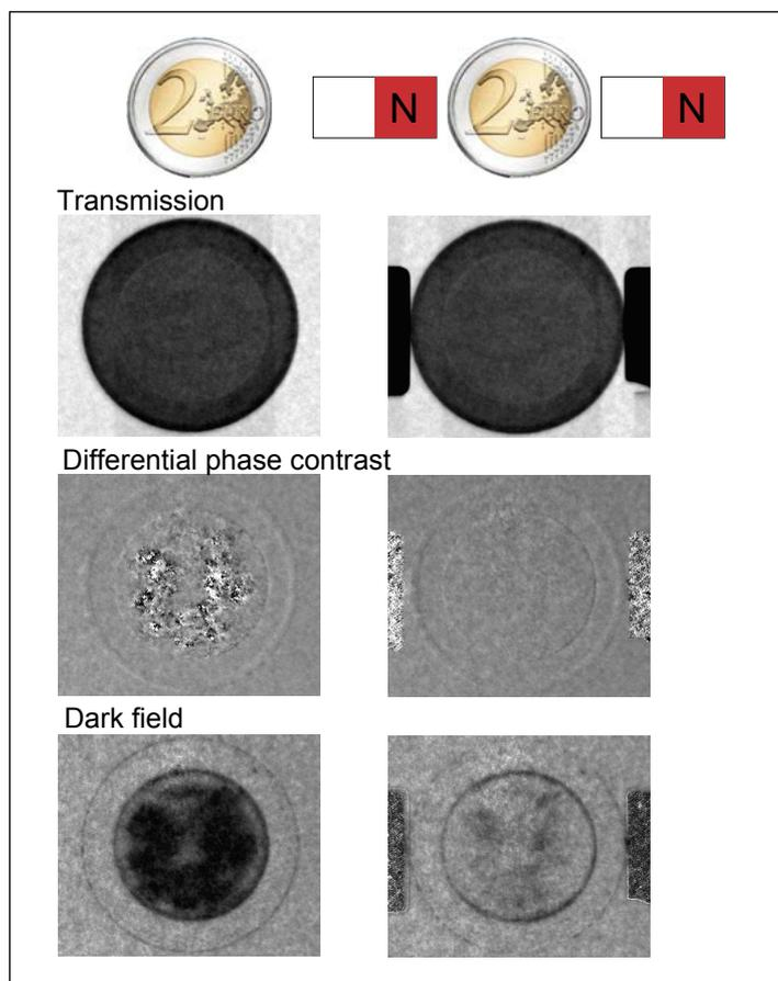
Figure 5: Demonstration of different nGI images produced when magnets are used on a 2 Euro coin.
