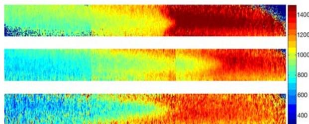
Figure 1: **Temperature distribution inside a channel-flow reactor for a methane/air flame at 3/5/10 bar (top/middle/bottom). Vertical scale is 10 times the horizontal; temperature scale: 300 K <  $T$  < 1500 K.**
