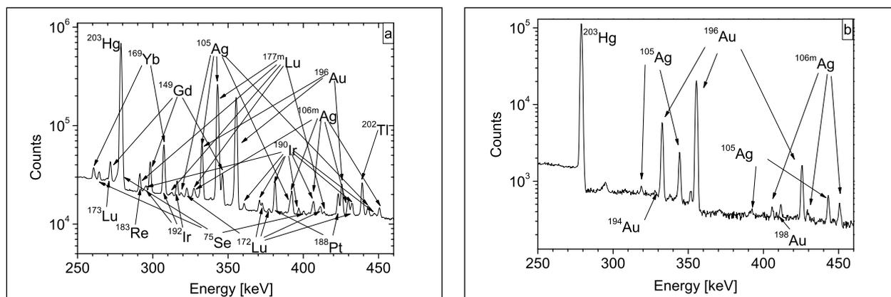
Figure 1:  $\gamma$ -spectra of Hg removed from the capsule (a) and taken from the bulk (b) (for details, see text).
