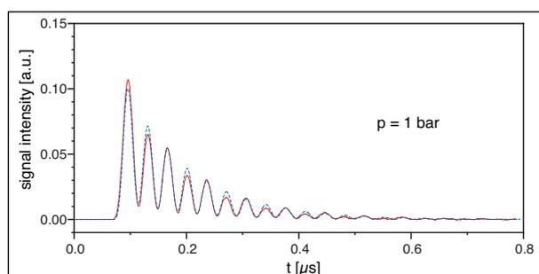
Figure 2: **Temporal evolution of LIG intensity of H<sub>2</sub>. Solid red line: experimental data; dashed blue line: simulation.**
