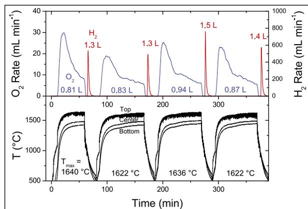
Figure 2: Thermochemical cycling of ceria (325 g) using the solar reactor with (a)  $\text{CO}_2$  and (b)  $\text{H}_2\text{O}$  as oxidant. The oxygen and fuel evolution rate, total volume of gas evolved, and maximum temperatures attained in the reactor are shown.
