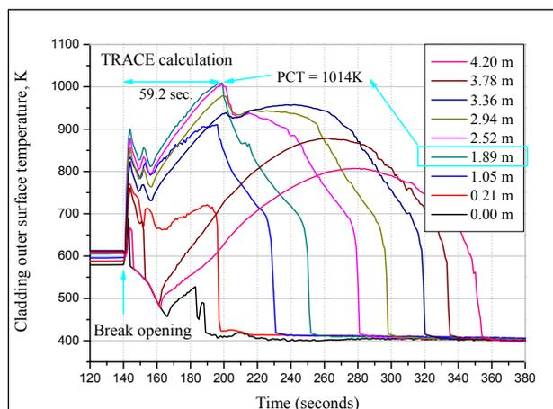
Figure 2: Results of TRACE EPR™ LBLOCA analysis.
