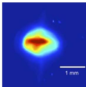
Figure 2: **Electron beam at 5.7 MeV energy, 180 pC charge; 0.55 mm.mrad emittance (10 % charge cut) with laser pulse length of 4.3 ps.**
