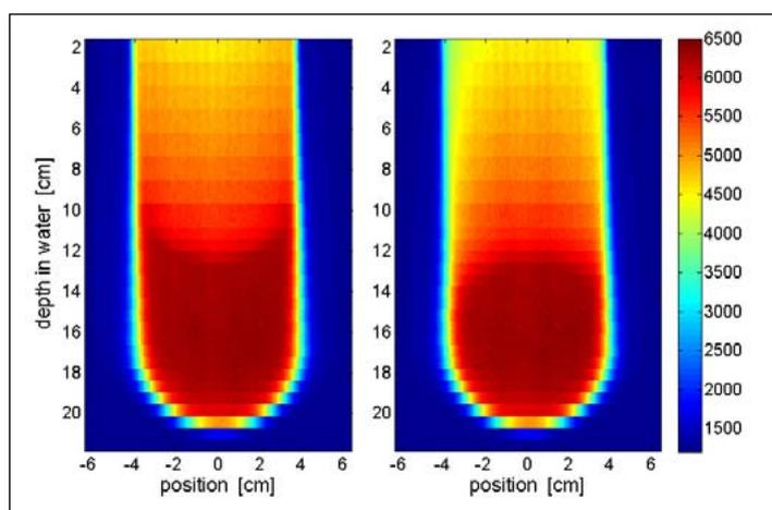
Figure 4: **Constructed images along the beam direction for the two fields, without (left) and with (right) proximal dose conformation.**
