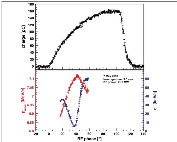
Figure 2: RF gun phase scan showing bunch charge, momentum and momentum spread as functions of the relative phase between gun RF and laser pulse.
