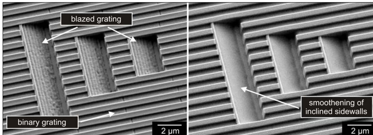
Figure 5: **Generation of an optical 3-D structure as needed for improved LED backlighting. A multi-level prism is integrated into a binary grating by electron-beam exposure and development (left). Due to local melting of the prism, the roughness is smoothed out while the outline of the complex 3-D shape is preserved (right).**
