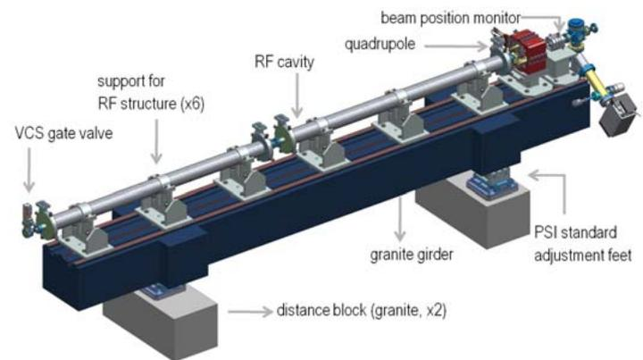
Figure 1: Linac support girder with two C-band cavities.
