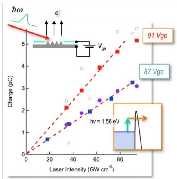
Figure 2: **Laser intensity dependence of the electron bunch charge generated from a  $1.2 \times 10^5$ -tip single-gate FEA under positive gate-emitter bias  $V_{ge}$ , irradiated by 50 fs Ti:Sapphire laser pulses [8].**
