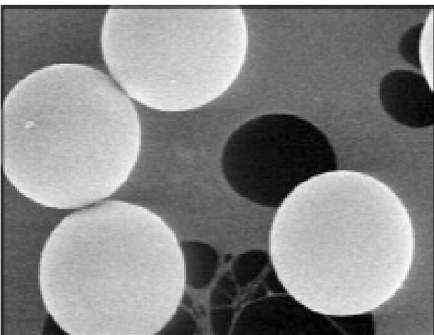
Figure 2: Electron micrographs of test aerosols: agglomerates (top) and spherical particles (bottom).
