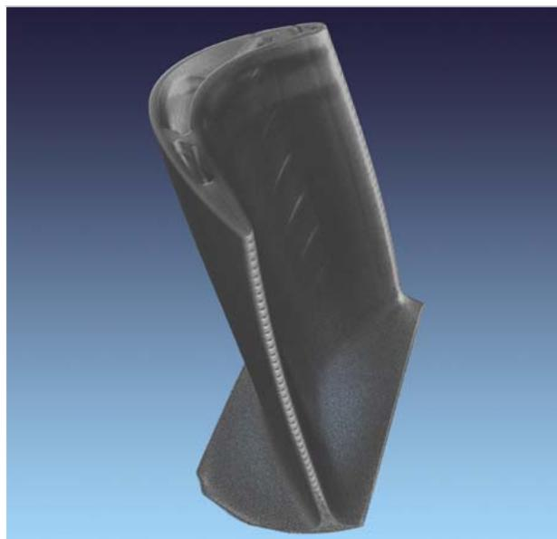
Figure 2: 3D reconstructed image of the turbine blade provided by Alstom, obtained by neutron tomography (NEUTRA, SINQ).
