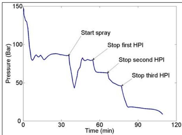
Figure 1: **Pressure response during an SLOCA, with operator actions.**
