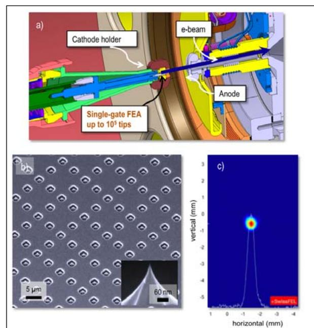
Figure 1: **(a) Schematic of FEA integration into the SwissFEL diode gun accelerator. (b) Scanning electron microscope image of a part of a 5 μm-pitch single-gate FEA with 10<sup>5</sup> emitter tips. The inset shows a single tip near the apex. (c) Scintillator screen image of a focussed field emission beam from the FEA shown in (b), accelerated to 200 keV in a 30 MV/m acceleration gradient.**
