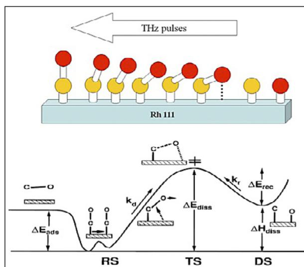
Figure 1: (Top) A schematic representation of THz-induced absorptive-dissociation of CO (yellow = C, red = O) on a Rh surface. (Bottom) A schematic energy-level diagram for the process (RS, TS and DS refer to the reactant, dissociated and transition states, respectively [2]).
