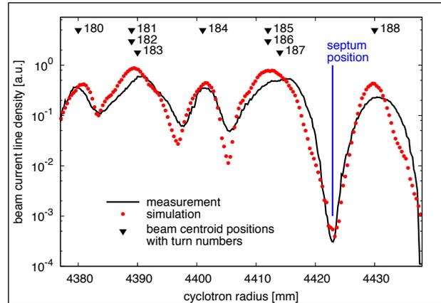
Figure 3: **Radial line density in the Ring Cyclotron.**
