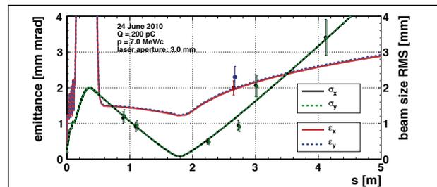
Figure 2: Measurements of emittance and beam size in the gun section (data points with error bars) in comparison to simulation results (solid and dashed lines).
