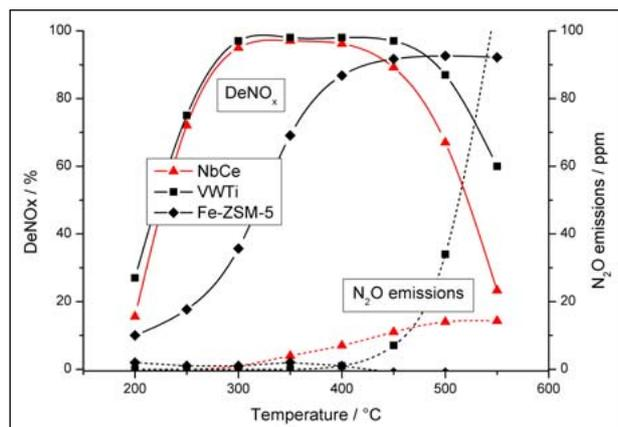
Figure 2:  $\text{NO}_x$  removal (DeNO $_x$ ) and  $\text{N}_2\text{O}$  emissions for NbCe, VWTi and Fe-ZSM-5.
