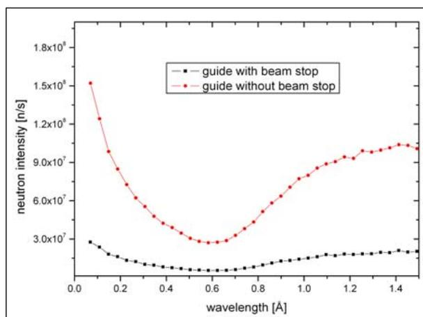
Figure 2: **Comparison of simulated background with and without beam stop for an elliptical guide setup.**
