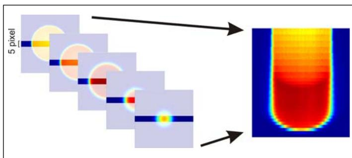
Figure 3: **Dose images (left) measured at increasing depths were combined to obtain a dose image as a function of depth (right).**
