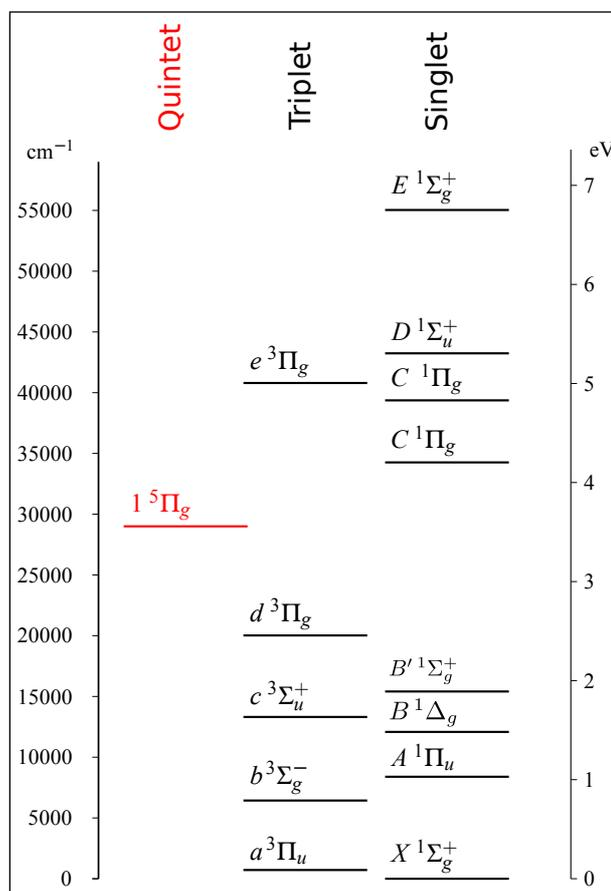
Figure 3: **Low-lying electronic states of C<sub>2</sub>. The singlet, triplet and quintet manifolds are indicated relative to the X  $1^1\Sigma_g^+$ ,  $v=0$  state. The  $1^5\Pi_g$  state is a dark state, not accessible by direct optical methods and characterized for the first time in this work.**
