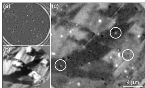
Figure 1: (a) X-ray PEEM image obtained with circularly polarized radiation at the iron  $L_3$  edge (708 eV). (b) Corresponding domain pattern of the cobalt support recorded at the cobalt  $L_3$  edge (778 eV). (c) Superposition of the images in (a) and (b).
