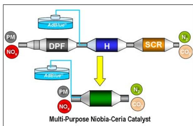
Figure 1: From three exhaust gas after-treatment components to one by means of a NbCe catalyst.
