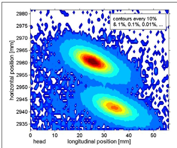
Figure 2: **Measured projections of bunches at the last two turns of Injector 2.**
