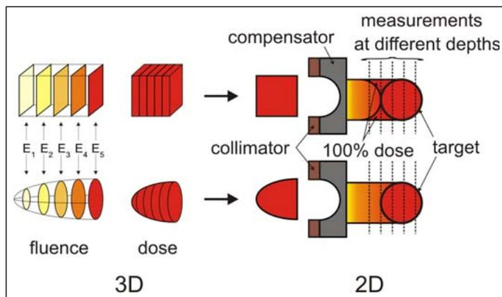
Figure 2: **Layer stacking for a spherical target; the illustration shows how shape shrinking of the more superficial layers can provide better conformity of target coverage.**
