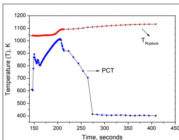
Figure 3: Results of FALCON EPR™ LBLOCA analysis.
