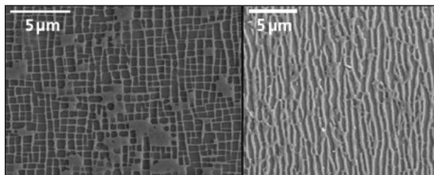
Figure 1: SEM micrographs showing, on the left, the initial microstructure of an SX Ni-based superalloy, where the cuboidal  $\gamma'$  precipitates are embedded in the  $\gamma$  matrix, and, on the right, degraded microstructure observed at the end of the manufacturing process of the turbine blade.
