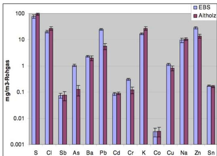
Figure 1: On-line measurement of trace elements with a liquid quench sampling system and ICP-OES at a wood-fired power station at Kleindöttingen, with regular scrap wood (“Altholz”) and also metal-loaded wood (EBS). Values are given in mg/Nm<sup>3</sup> raw gas.
