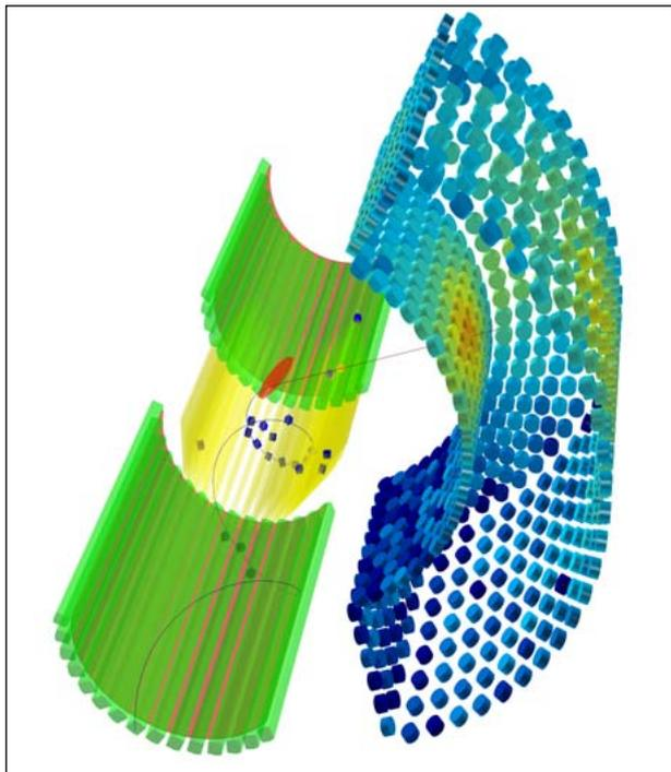
Figure 3: **One of the signal-like events, as seen by the MEG detector. The disc at the centre is the muon stopping target. The photon is detected on the right-hand side by the liquid xenon calorimeter, where each small cylinder corresponds to one photomultiplier, with the shade representing the light intensity seen by that photomultiplier. On the lower left-hand side, the positron track can be seen, first traversing the drift chamber system and then hitting three consecutive timing counters.**
