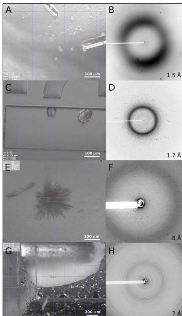
Figure 2: *isXds* experiments conducted at beamline X06DA at the SLS. *isXds* unambiguously aids in identifying salt crystals (A, B). Well-diffracting crystals, such as lysozyme, yield high-resolution diffraction images, using microfluidic chips to reduce background scattering (C, D). *isXds* also enables diffraction information to be obtained from small crystals (E, F). Even nanocrystals in high concentrations produce clearly visible powder diffraction patterns (G, H).
