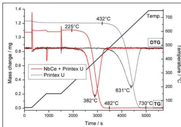
Figure 3: TG and DTG curves recorded during Printex U oxidation with (full line) or without (dotted line) NbCe.
