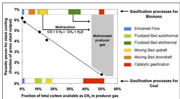
Figure 2: High methane content in producer gas from (coal and) biomass provides a benefit in fuel cell systems with integrated gasification.
