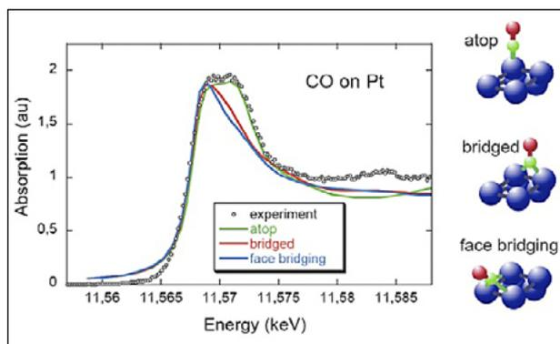
Figure 2: In a single-shot, time-resolved experiment at the SwissFEL, a near-edge X-ray absorption spectrum can be collected which reflects the instantaneous atomic and electronic structure of adsorbed molecules on a surface [4].
