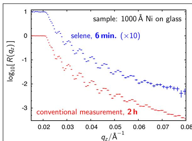
Figure 3: Performance gain using the new elliptical guide on SELENE/AMOR, demonstrated on an Ni layer.
