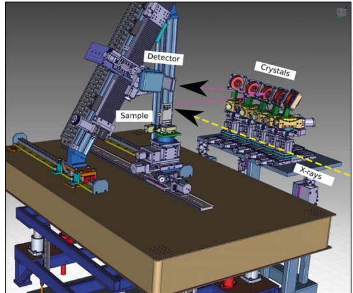
Figure 1: Compact X-ray emission spectrometer at the superXAS beamline of the SLS.
