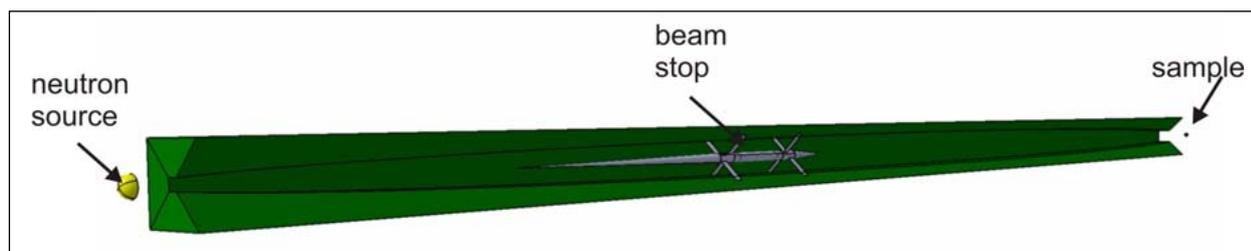
Figure 1: **Double-elliptic neutron guide with integrated beam stop.**
