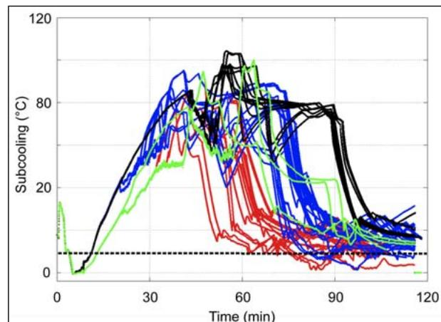
Figure 3: **Margin to saturation conditions.**
