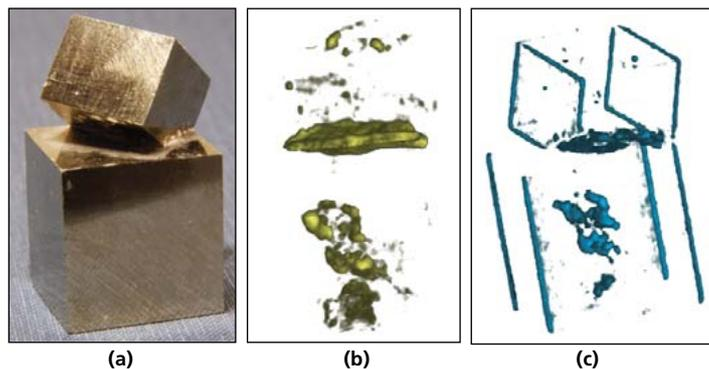
Figure 3: Picture of the pyrite sample (a); volume-rendered transmission NCT of the sample (b); and dark-field NCT (c).
