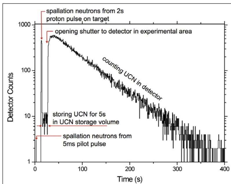
Figure 2: Count rate versus time after the beam pulse in one of the UCN counters. A peak due to spallation neutrons during the beam pulse (1.8 mA, 2 s) can be seen, which is followed by a 5 s storage time. Then the shutter towards the experimental area and detector is opened and the UCN are counted. The count rate decreases due to draining of the storage volume.
