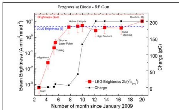
Figure 1: **Progress of the LEG beam brightness towards the SwissFEL goal.**
