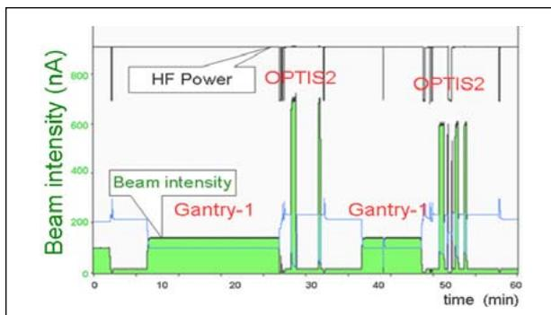
Figure 4: Beam switching between the treatment rooms involves a change in extracted beam intensity and is done within 20 sec.
