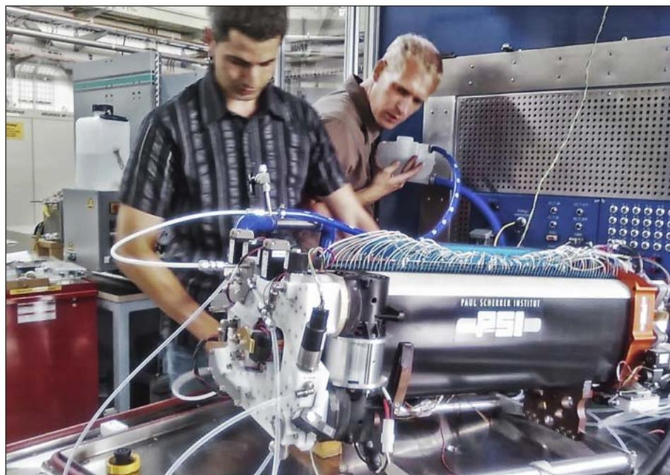
Figure 1: H<sub>2</sub>/O<sub>2</sub> polymer electrolyte fuel cell system developed in collaboration with Belenos Clean Power AG, Biel, Switzerland.
