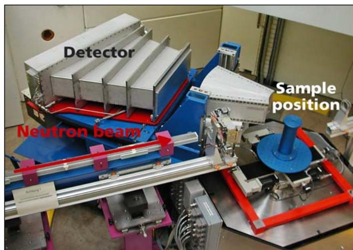
Figure 3: Layout of the neutron strain scanner POLDI (SINQ).
