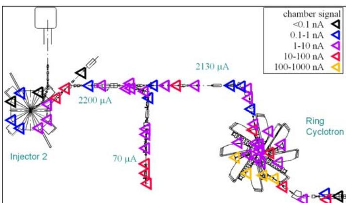
Figure 1: Ionisation chamber readings as a measure of beam loss at cyclotrons and beamlines.
