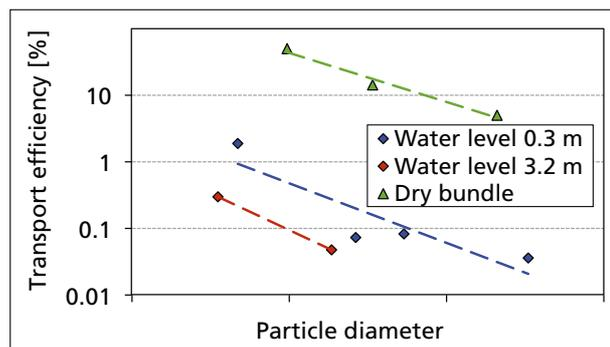
Figure 3: Aerosol transport efficiency in a dry steam generator bundle compared with that of the bundle flooded with water.
