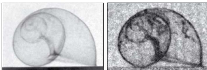
Figure 4: Transmission (left) and dark-field (right) images of a snail shell with a surface imperfection.
