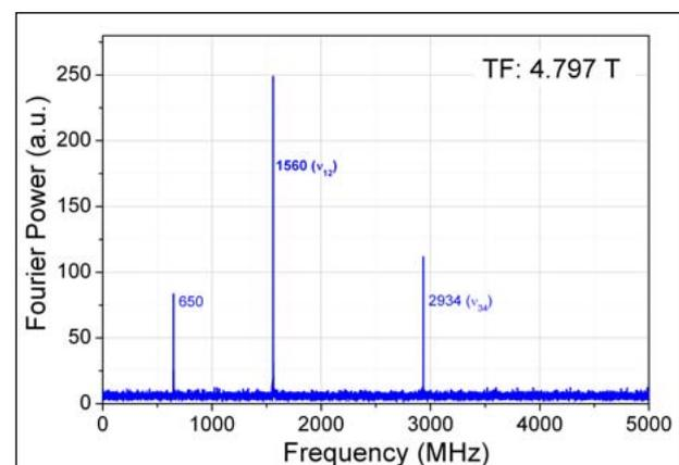
**Figure 1: Frequency spectrum of a  $\mu$ SR spectrum in a quartz crystal in a field of 4.797 T at ambient temperature, obtained with APD-based, fast-timing detector modules. The free-muon precession and two-muonium precession frequencies are observed. From the signal amplitudes, a time resolution of 80 ps is inferred. Such a high frequency  $\mu$ SR signal in a high magnetic field has never before been measured.**
