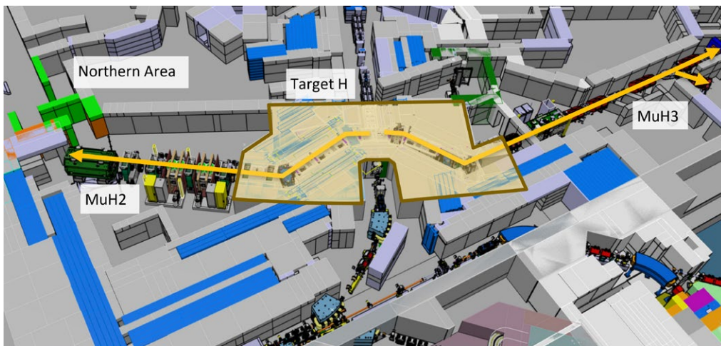
Figure 4.2.22: Size of the new steel shielding in yellow.
