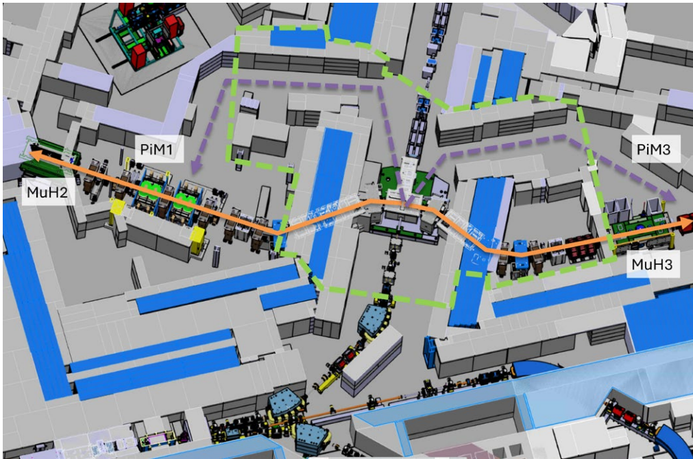
Figure 4.2.21: Current shielding situation with the new beamlines MuH2 and MuH3 in orange. Dashed violet current beamline PiM1 and PiM3.
