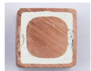
Figure 3.2.1: MIC cross section
