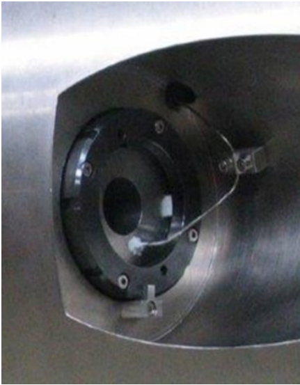
Figure 3.4.6: Thermocouple connection at front face of the protection collimator of Target M. Note that the protection collimator is electrically insulated to be able to measure the proton beam loss current in the collimator.
