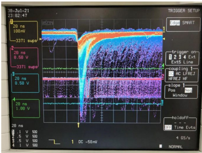
Figure 2.2.18: An example of the Pill signal at the oscilloscope. The beam momentum is 28 MeV/s. The high amplitude waveforms are associated with the muons while the low ones with the positrons (in this case cut by the trigger threshold). The separation between the two particle types is very clear.
