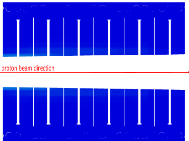
Figure 3.1.77: Power density on the vertical plane passing through the geometrical center of KHH1.
