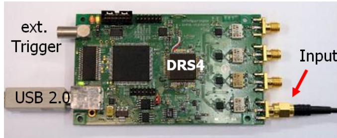
Figure 6 USB powered DRS4 evaluation board with four 2048 cells deep input channels
