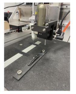
Retro reflective paint is used to dispense small dots on the rings
