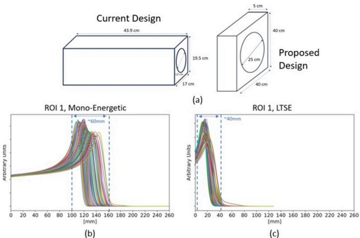
Showing (a) the current and our proposed design of a Multi-Layer Ionisation Chamber, (b,c) the difference in residual Range and Bragg peak spread of using a 210 MeV mono-energetic approach and the predicted Locally-Tuned Single Energy (LTSE) approach for one of the ROIs.
