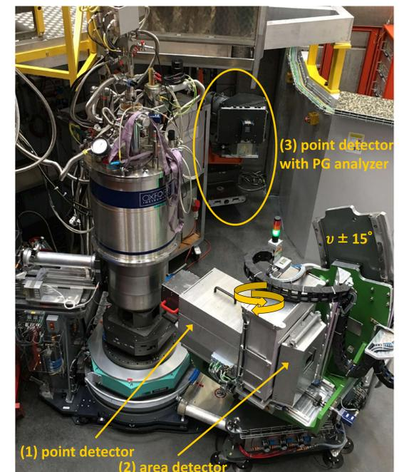
Zebra in 4-circle (left) and tilting (right) geometry, respectively using a CCR and a 10 T vertical magnet with dilution fridge. The three detectors are spotted on the right.
