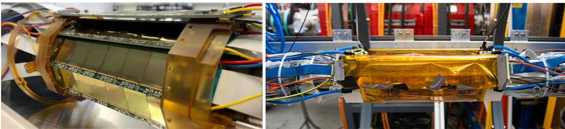
**Figure 4.** Demonstrator pixel tracker (left) and SciFi (right) installed along with the powering and cooling services during the Integration Run at PSI in 2021.
