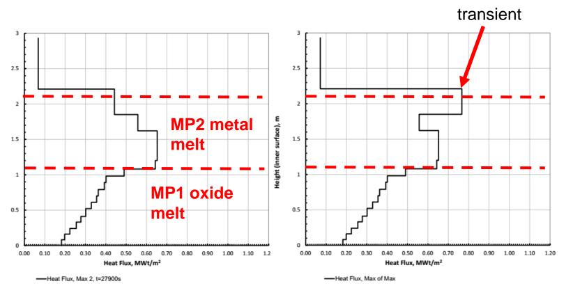
LH external heat flux at maximal value (t=27900s)
