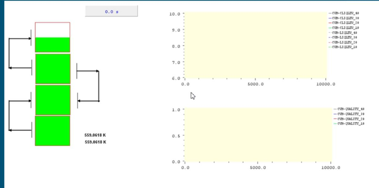
Setting FP Junction Elevation to top/bottom elevation is more representative of quiescent boiling
