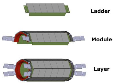
Each pixel layer  $\sim 0.1\%$  radiation length ( $X_0$ )
