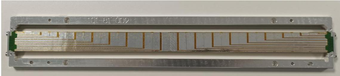
**1)** The HDI flex is installed on a ring frame and glue is applied at its back so that chips can be glued on it.
