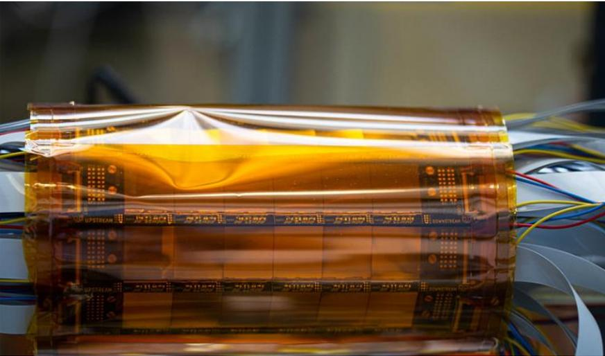
In this early prototype, the ladders were not built on HDI flexes. Instead, PCB were designed together with bus lines (white cables) and connectors.
