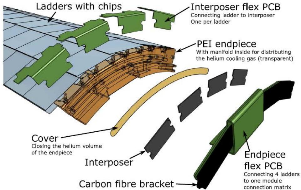
Exploded view of the outer layer module assembly.
