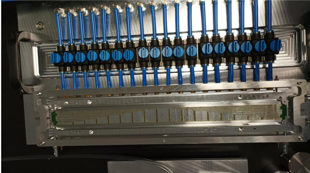
**3)** The ring frame is slotted in over the chips on the chip chuck.
