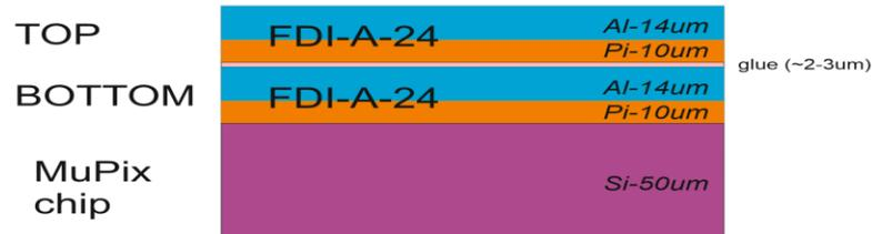
The HDI flex is a stack of two 14 $\mu$ m thick aluminium layers separated by 2 polyimide layers.
