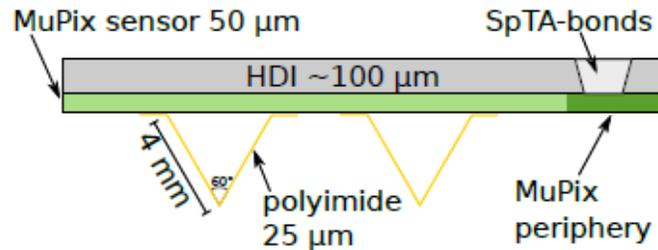
V-folds are made of  $25\mu\text{m}$  thick polyamide layer with a V-shaped cross section. They run along the ladder longitudinal side, from end to end.
