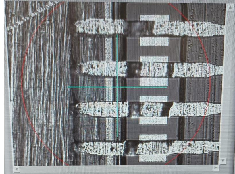
**4)** Fine alignment of Al traces on the HDI flex against the chip pads underneath.
