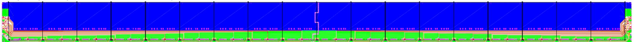
The top layer is electrically and mechanically divided in half (right-left symmetry) and it is glued on the bottom layer. The middle cut helps the alignment of the layers during the production phase.
