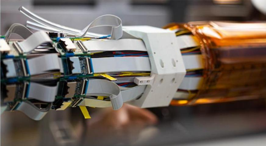
This is the inner module of the tracker detector in Mu3e. There are two layers made of 18 (8+10) ladders containing 6 chips each.
