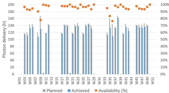
**Figure 11:** SwissFEL Aramis operation statistics during photon delivery weeks in 2021.
