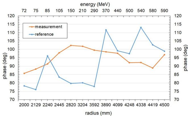
**Figure 3:** Phase in the Ring cyclotron vs the radius respectively the proton energy. Red denotes the measurement before the incident, blue a curve measured during the setup phase.
