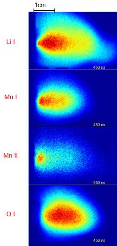
Fig.: Element-selective plasma imaging of the PLD thin film growth of  $\text{LiMn}_2\text{O}_4$
