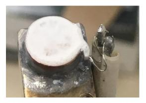
Figure S 4-6. K-feldspar powder sample coated on the sample cryo-holder surface.
