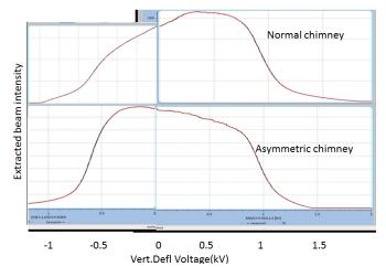
**Figure 9:** Intensity of extracted beam from COMET as a function of Vd, the voltage at the vertical deflector plate for two different chimney hole positions.
