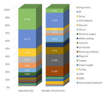
**Figure 2:** Downtime characteristics of the operational period 2019 by category. Shown are outages that lasted longer than five minutes. In total, only 94 were registered in 2019, which corresponds to a total downtime of 124 hours.
