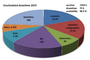
Figure 8: Beam outages per failure category for PROSCAN.
