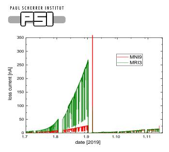
Figure 3: Röntgen radiation detected by the loss monitors MNI9 (red) and MRI13 (green) in the Ring cyclotron. After the treatment with AQUADAG the radiation level clearly diminished.
