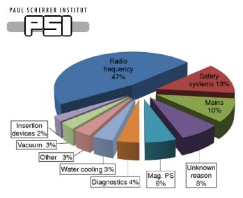
Figure 6: Beam outages per failure category for the SLS.
