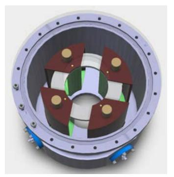
Figure 10: Axial view of the beam position monitor, which consists of four cavities surrounding the beam.
